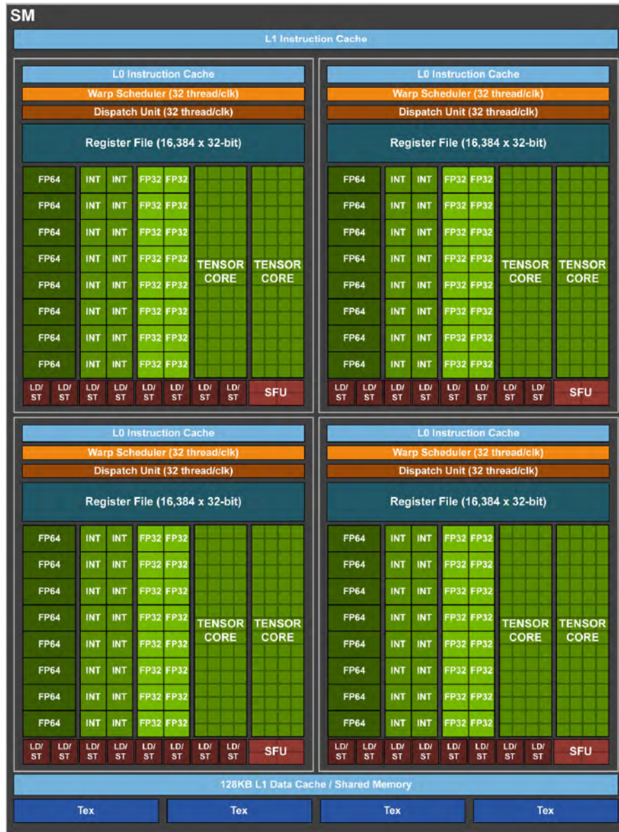
Figure 2.7: Details within one streaming multi-processors of Tesla V100.
