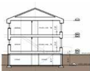
Figure 3-38: Fourplex Section showing basement storage (Design: EVOQ Architects and W Semple)
