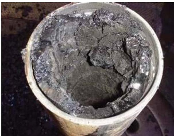
**Figure 9. Asphaltene deposition in a pipeline.**
