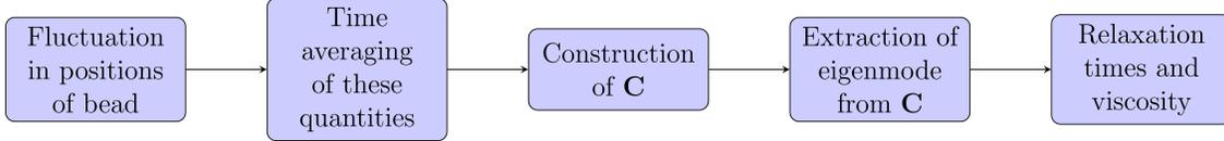
Figure A.2: Flow chart showing the procedure of POD analysis.
