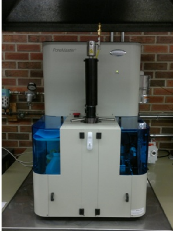
Figure 2.3 – PoreMaster 33 intrusion porosimeter, manufactured by Quantachrome Instruments.
