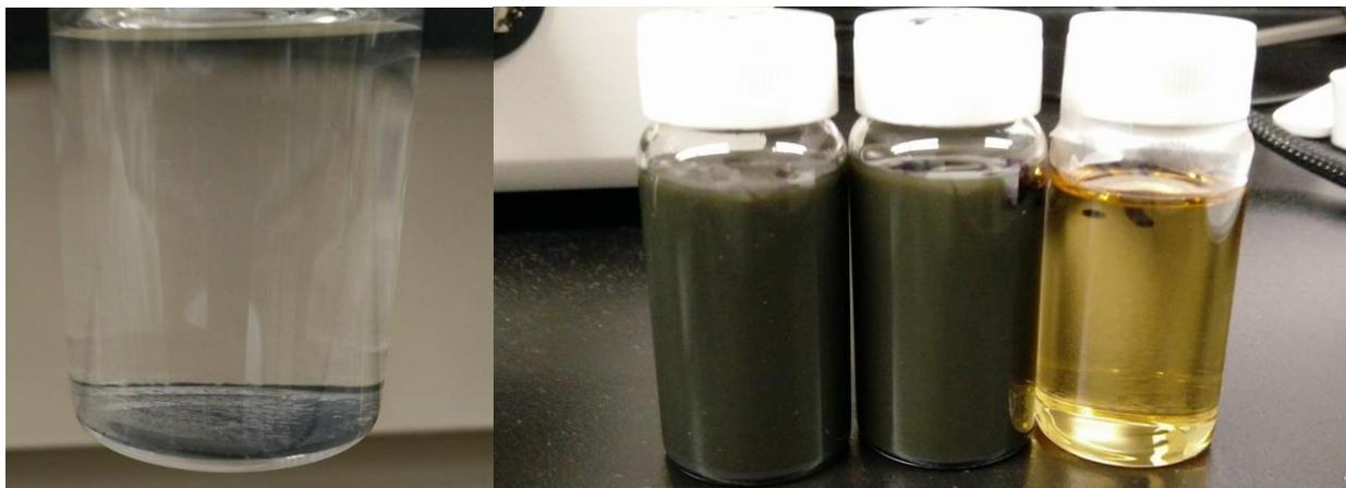
Figure 2.4 Precipitation of nanoparticles after 1 week in DI water, sample was the supernatant obtained 6000G RCF (left), yellowish color solution on the far right showing the organic solvent stabilized nanosheets compared to samples that have not been centrifuged after 1 week (right)
