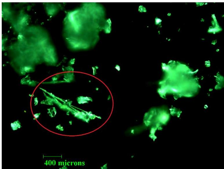
Figure 3.4 Top layer of MoS<sub>2</sub> mineral where the needle like shapes were suspected to be contaminants (primarily calcium)
