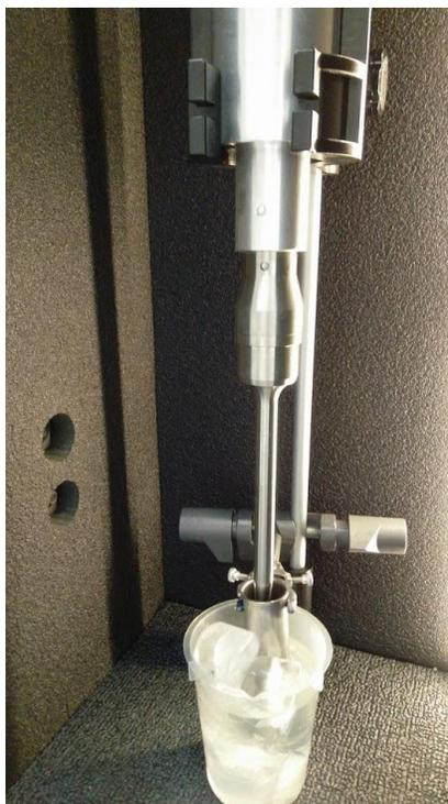
Figure 2.2 Liquid phase exfoliation experimental setup with the probe, stainless steel vial and ice bath
