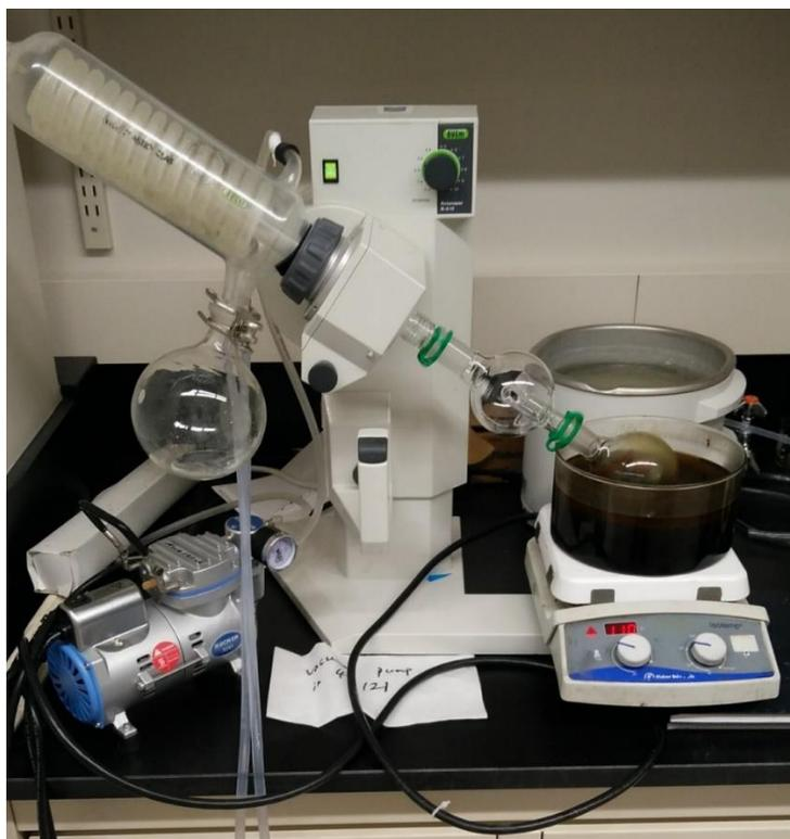
Figure 2.1 RotoVap experimental setup with vacuum pump and cooling water cycling system
