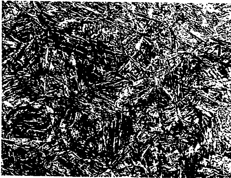
Figure 47. The Microstructure of 420 Steel Tempered at 650°C, FeCl 3 Etchant, 180x
