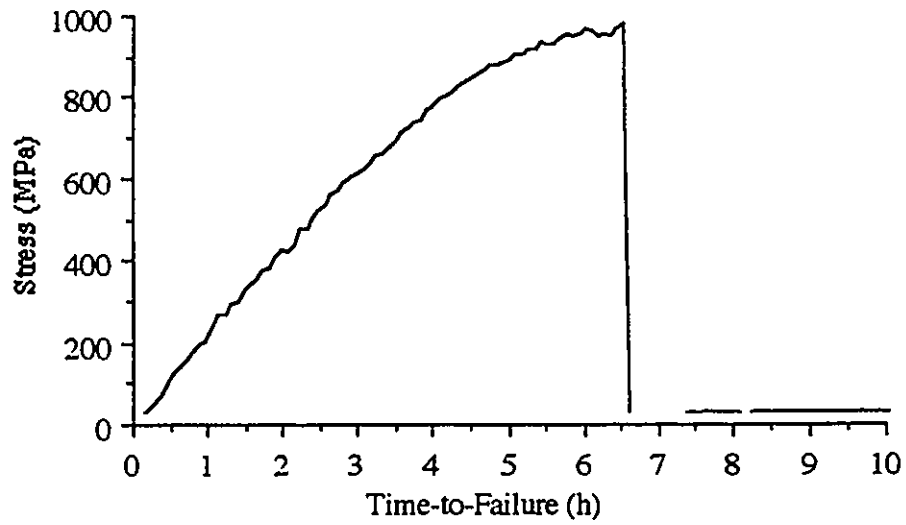
Figure 64. Stress versus Time Curve for Specimen 7 SSRT
