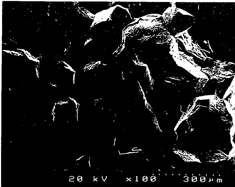
Figure 80. SEM Fractograph of Specimen 3
