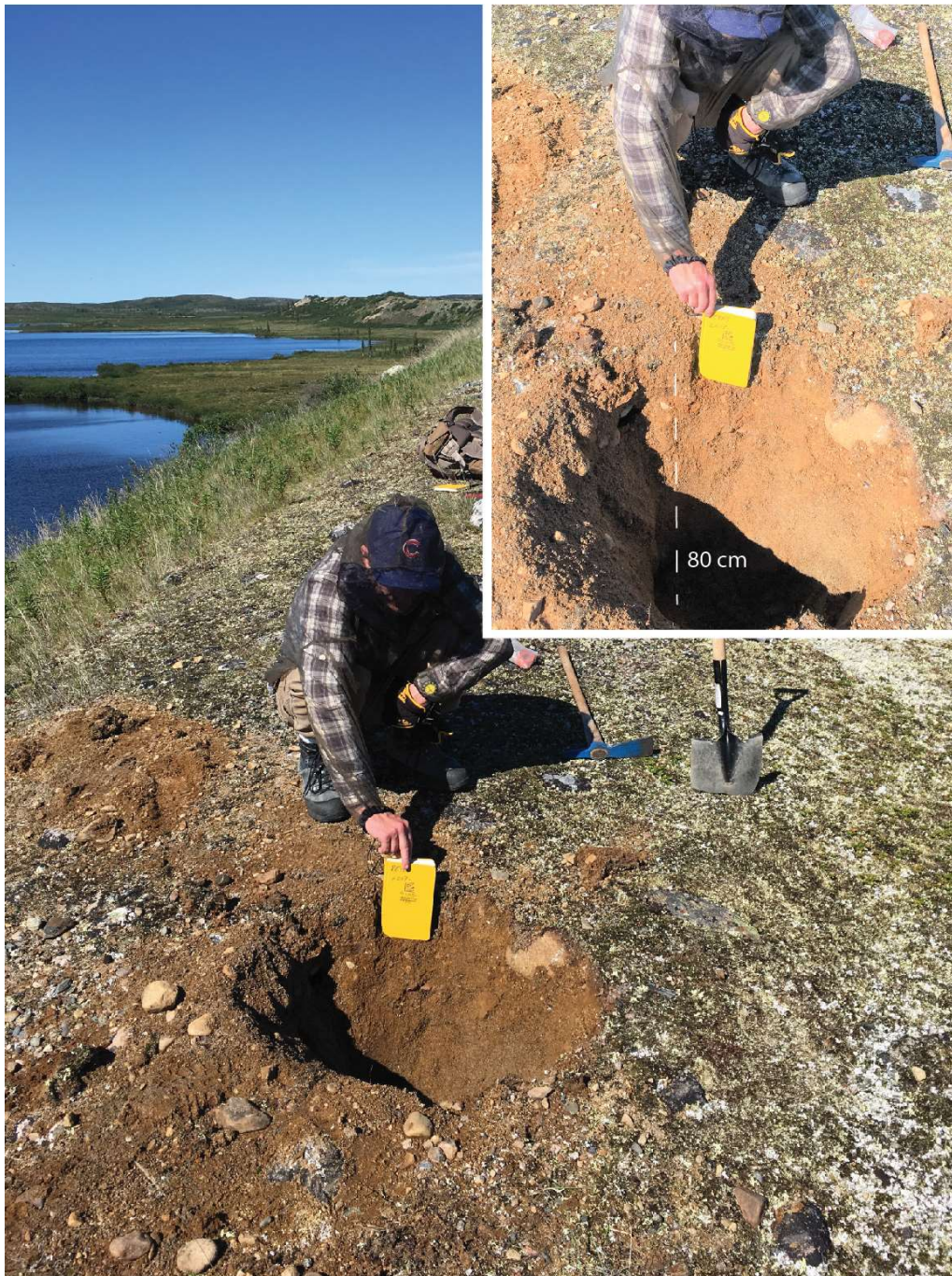
Figure 3.7. Sample location GSB17-D1. The esker crest stands ~ 15m above the nearby lake. Small shrubs and boulders are infrequent along the crest; however the slopes are heavily vegetated. A pit 80 cm in depth was excavated for sampling, and no obvious weathering horizon was observed. Grain sizes ranging from large cobbles to very fine sand are present within the sample pit, and the mean grain size sampled ranges from pebbles to medium sand.
