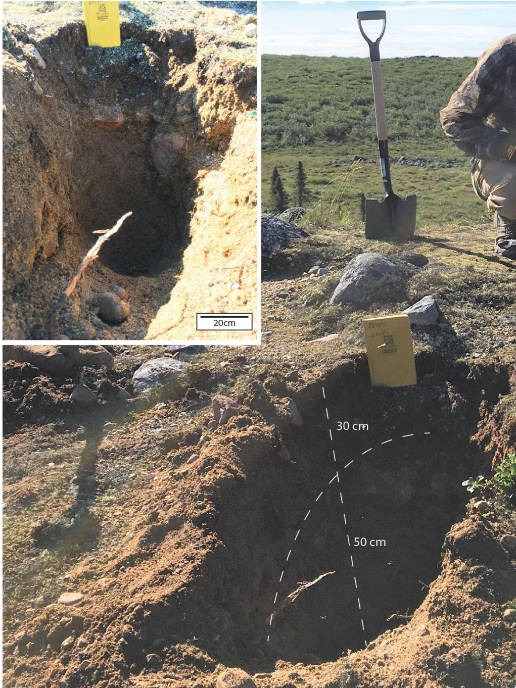
Figure 3.6. Sample location GSB17-B1. The surface of the esker is vegetated with small shrubs and lichen, along with occasional cobbles and boulders. A weathering horizon with small roots is visible within the top 30 cm of the sample pit (total depth 80 cm). Grain sizes ranging from boulders to very fine sand can be observed within the sample pit, although the largest grain sizes sampled were small cobbles while the mean grain size sampled ranges from pebbles to medium sand.
