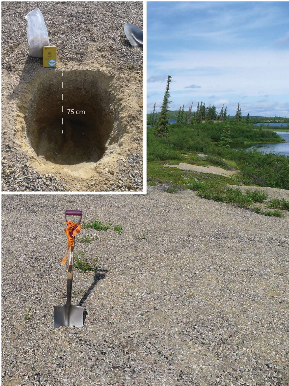
Figure 3.4. Sample location AVR16-15. The surface of the esker is intermittently bare gravel with vegetated areas of shrubs and small trees. The esker is composed almost entirely of pebble sized clasts or smaller and stands ~5m above the adjacent river. A sample ranging from pebbles to very fine sand was collected from a pit 75 cm in depth.
