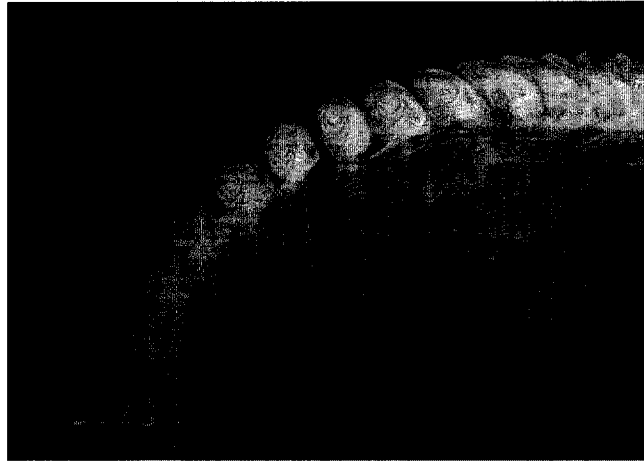
(c) The instability occurs closer to the jet shear layer at higher amplitudes. The upstream and downstream jet shear layer are unstable. Vortex pairs have more of an upward impulse. W_{sj} \approx 0.56 m/s, M_M \approx 1.51 , Re_d \approx 1250 .
