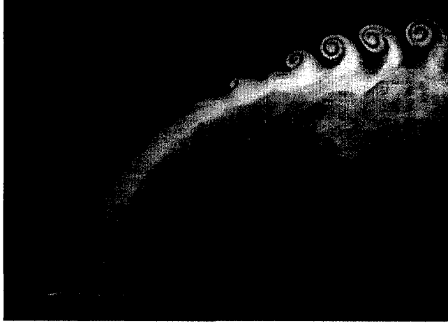
(a) The unforced JICF vortex structure. R = M_M = 1.39 and Re_d = 1147 . Vortex roll-up on the upstream side appears to be periodic, but the instability occurs intermittently.
