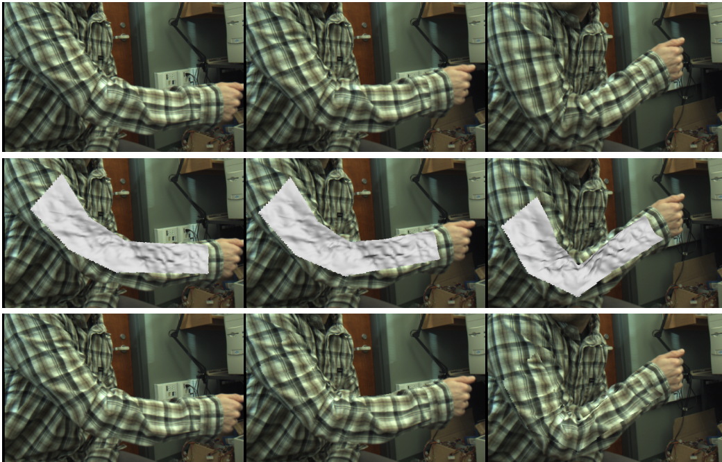
Figure 6.21: Top: input images from time 0, 5, 14. Middle: reconstructed geometry. Bottom: deformed textured with I_{1,0} .
