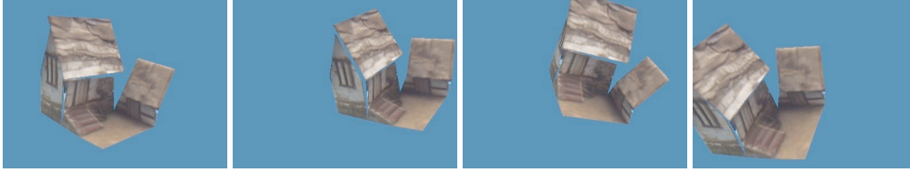
Figure 5.7: Frames 0, 30, 100, and 130 of 200 from one view of the fast moving synthetic house sequence. The object has sufficient texture (for the SSD method) and the silhouettes are perfect.
