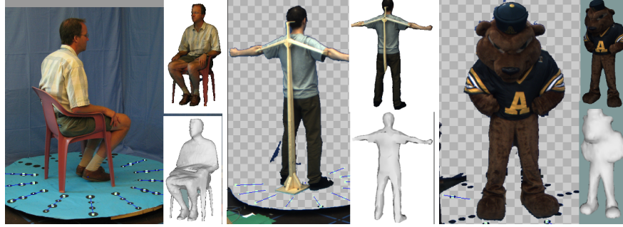
Figure 4.2: A single camera can be used when any subject wobbles are inhibited by a support system (either by a chair or vertical support). However, the support typically interferes with the geometry (left, chair) or the texture (vertical support). Using a human template geometry would restrict the acquisition to normal people-like geometries and would not allow such things as mascots or baggy clothing.
