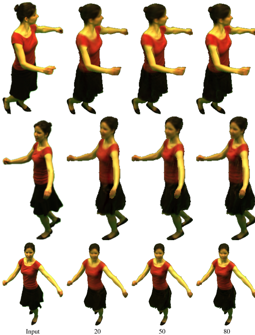
Figure 7.29: Rendered results for the Samba sequence using various numbers of basis functions. File sizes: 7MB, 13MB, 20MB.
