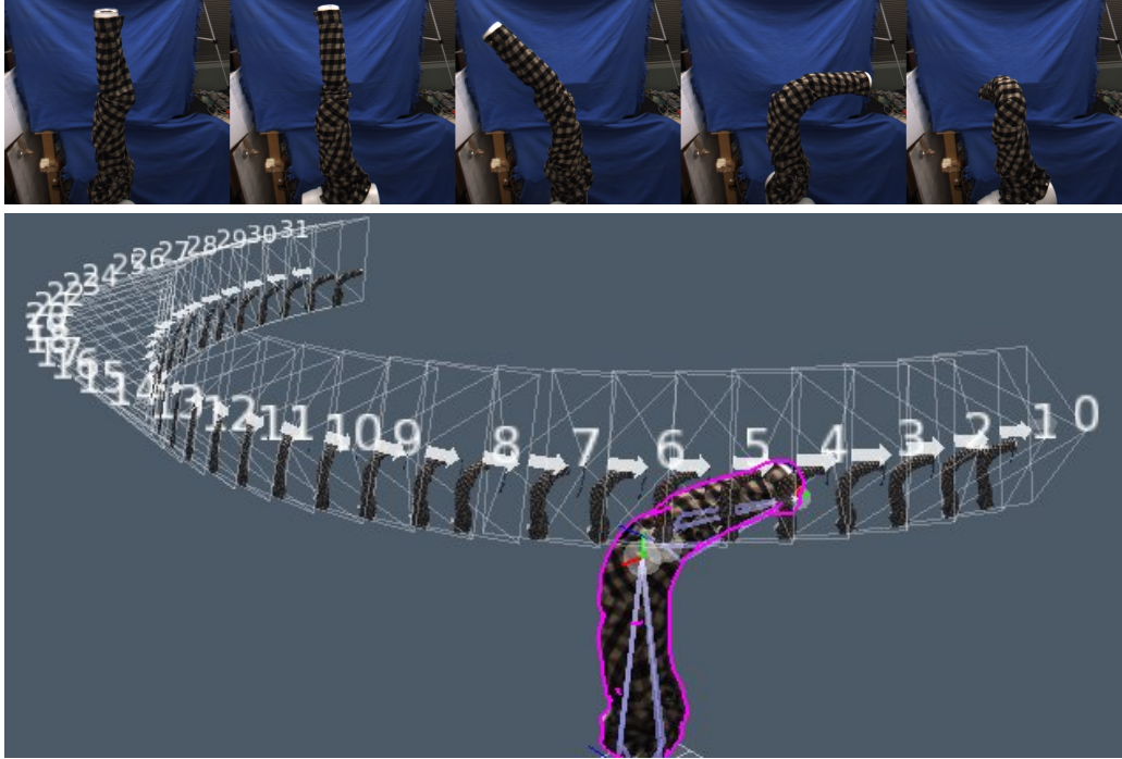
Figure 7.8: Input images of the Plaid cloth taken by a single camera (top). The arm was captured in 14 elbow poses differing by 10 degrees. For each pose, the base was rotated over 180 degrees giving 33 views for each pose (bottom)
