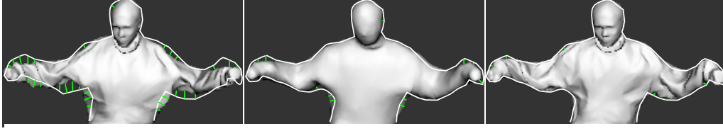
Figure 6.22: Left: the posed mesh doesn't agree with the silhouette (white line). Constraints are added (green lines) and Eq. 6.51 is solved with a low-level of detail to give the results (middle). The process is repeated with increasing detail to give the final result (right). The final result retains detail of the original model, but better fills the silhouette.
