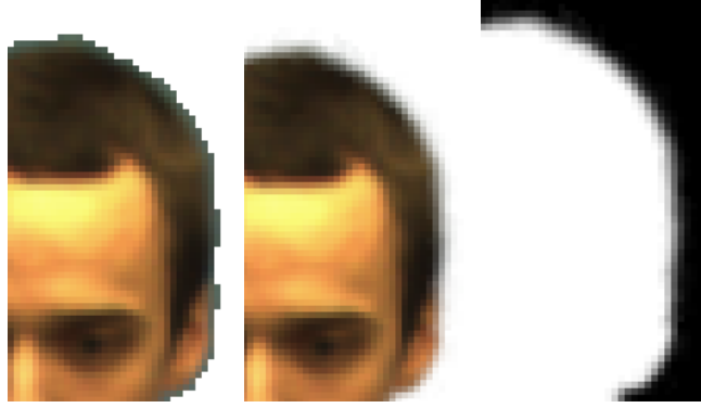
Figure 4.6: The input binary input images are matted to obtain a better estimate of the foreground color and alpha values. Input image (left), matted image (middle), and foreground alpha (right).
