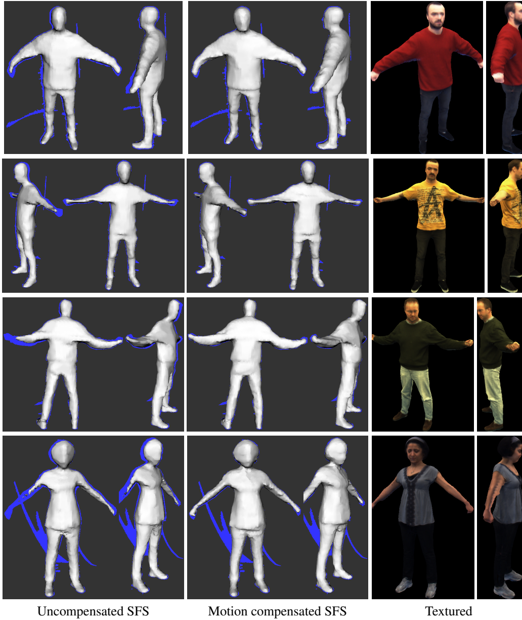
Figure 4.18: Uncompensated SFS, motion compensated SFS, and textured motion compensated views. The blue regions denote portions of the input silhouette not occupied by the reconstructed model. In all cases, the refined model covers more of the input silhouettes.
