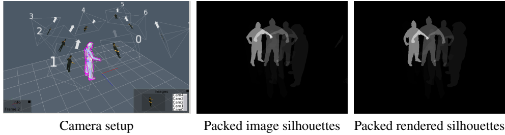
Figure 5.4: The silhouettes of the input images and rendered silhouettes are packed into bit planes of a single image. The XOR term is evaluated per-pixel by performing a bit-wise XOR and counting the number of bits that are set.
