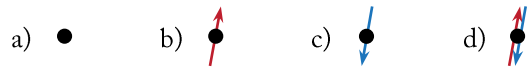
Figure 3 – Assignments of (a) vacancy, (b) spin “up”, (c) spin “down”, and (d) double occupancy for a given site.
