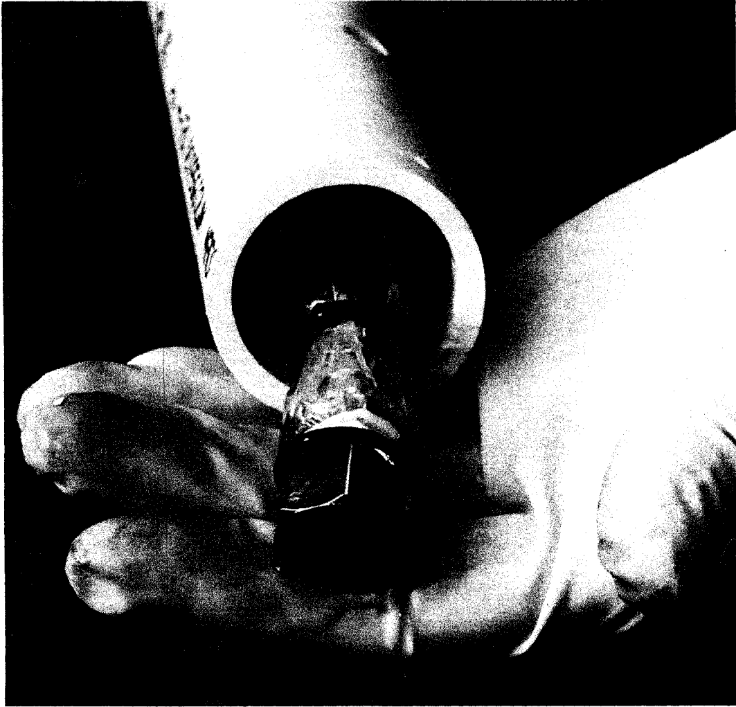
Figure 2.1. Diffusion Sampling Nozzle
