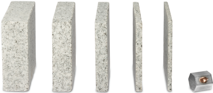
Fig. 1 Photograph of the tonalite targets (left to right: 40 mm to 7 mm thicknesses) with 65 g aluminum projectile with copper brushes. The projectile is 30 mm in length.
