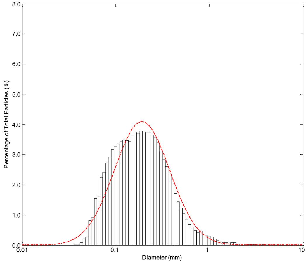
Figure 3-4: The raw size distribution of all particles (i.e. ice and sediment) observed at the Village Bridge on the Kananaskis River March 1, 2015. The dashed line represents the corresponding lognormal distribution calculated using the same mean and standard deviation as the measured size distribution.
