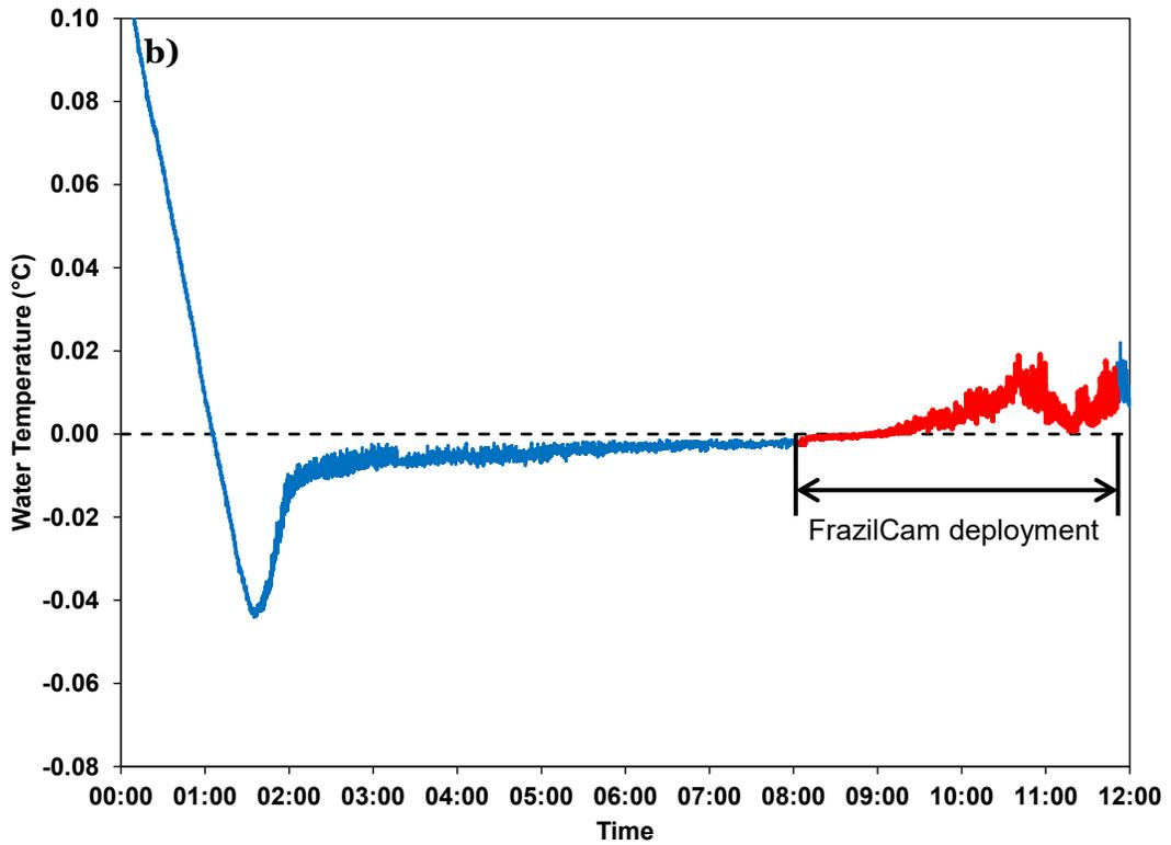
Figure 3-15: Time series of water temperatures during the supercooling events observed on the Kananaskis River a) at the Village Bridge overnight from February 28 to March 1, 2015, and b) at the Opal site on March 1, 2015.
