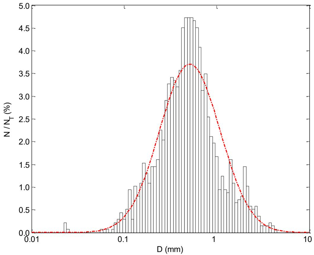
Figure 2-5: Size distribution for particles observed prior to flocculation for an experiment carried out at a propeller speed of 325 rpm.  $N$  is the number of particles in each bin,  $N_T$  is the total number of particles, and  $D$  is the diameter. The dot-dash line is the corresponding ideal lognormal distribution.
