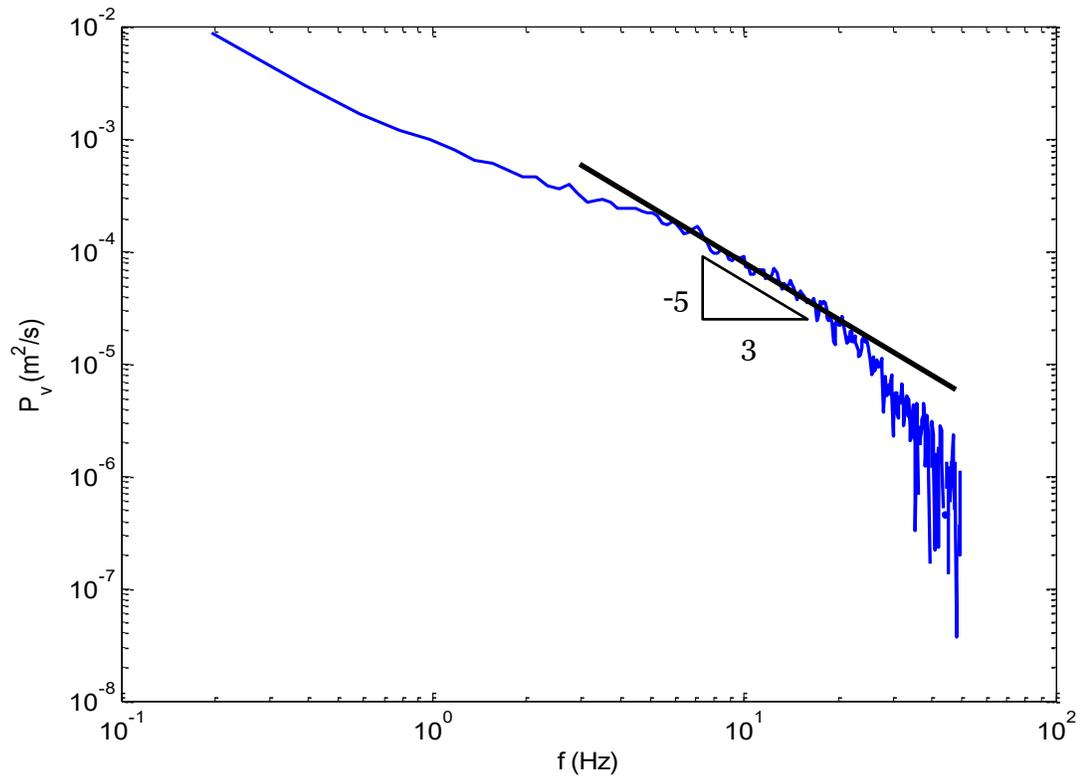
Figure 2-2: Power spectra calculated for the 325 rpm propeller speed in the centre of the tank at a depth of 625 mm.  $P_v$  is the value of the power spectral density ( $\text{m}^2/\text{s}$ ) in the  $y$ -direction and  $f$  is the frequency (Hz). A line with a slope of  $-5/3$  is shown over the region determined to be the inertial subrange, used to calculate the dissipation rate of the turbulent kinetic energy.
