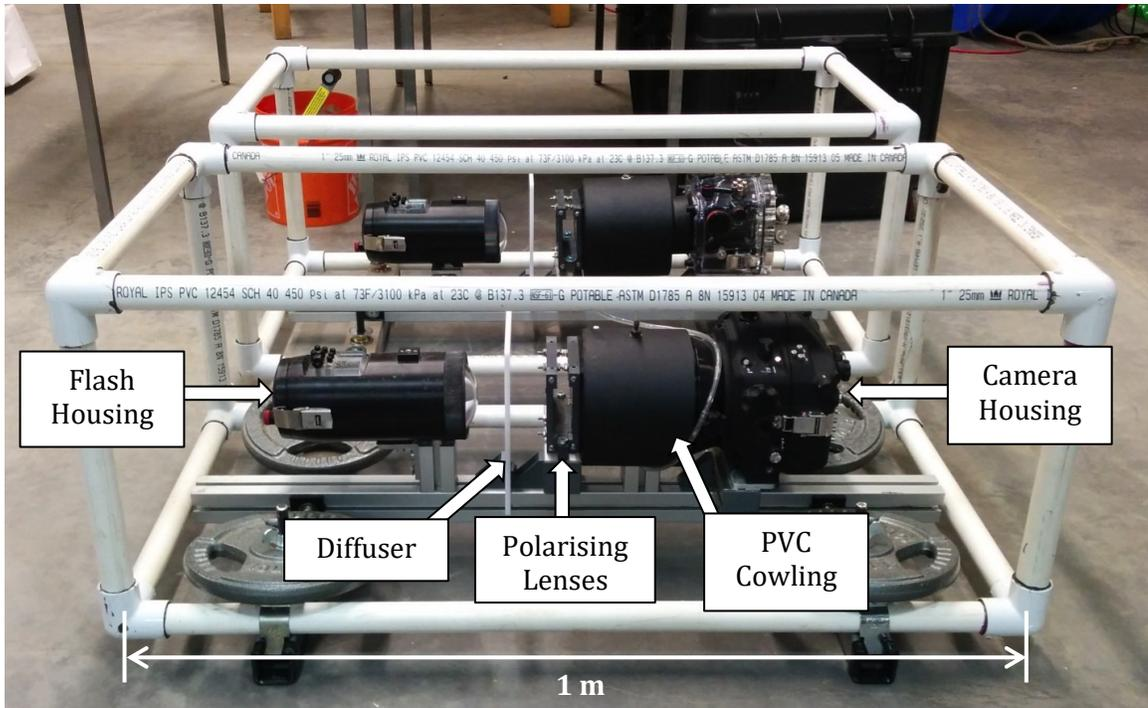
Figure 3-2: Digital image showing the final configuration of the two FrazilCam systems.
