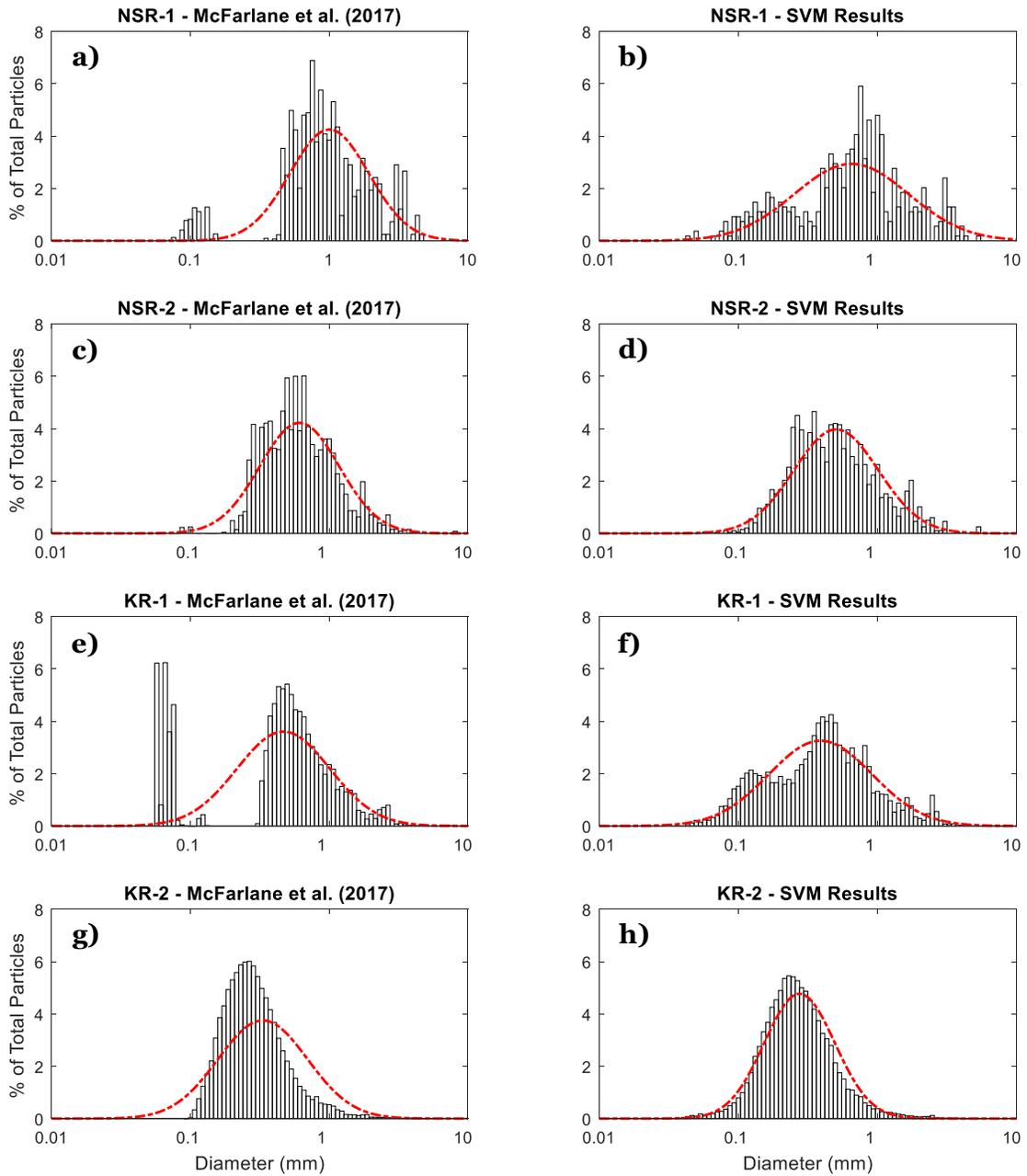
Figure 4-3: Comparison of the frazil ice size distributions estimated by McFarlane et al. (2017) (left column) to those calculated using the SVM (right column). The red dashed line indicates a lognormal distribution with the same mean and standard deviation as the observed particles.
