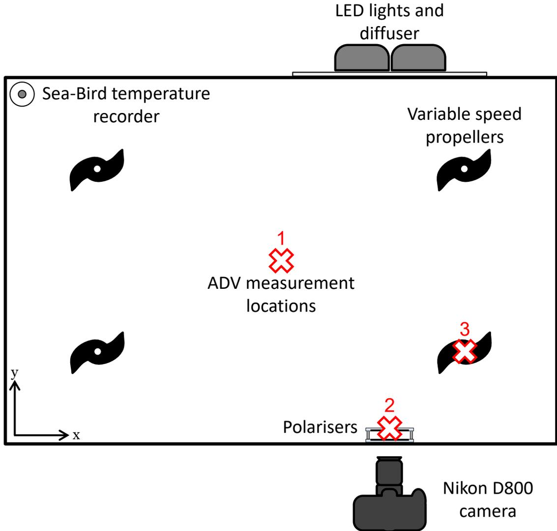
Figure 2-1: Plan view of the frazil ice tank showing the locations of the camera, LED lights, polarisers, four propellers, and the three locations where the ADV measurements were made (marked by the red X's). The coordinate system for the ADV measurements is defined such that the positive  $x$  and  $y$ -directions are towards the right and back of the tank, respectively, and the positive  $z$ -direction is towards the water surface.
