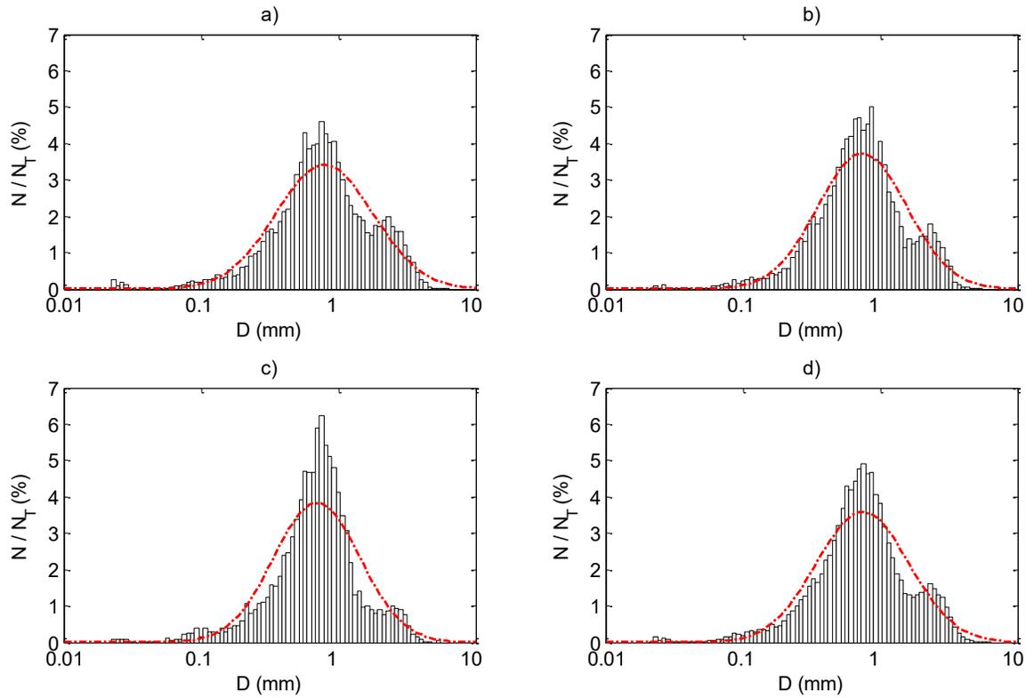
Figure 2-10: Ensemble size distributions at the 125 rpm propeller speed for a) the production range (i.e. from  $t_{10}$  to  $t_{90a}$ ), b) the peak range (i.e. between  $t_{90a}$  and  $t_{90b}$ ), c) the flocculation range (i.e. between  $t_{90b}$  and  $t_{30}$ ) and d) the entire data series.  $N$  is the number of particles in each bin,  $N_T$  is the total number of particles, and  $D$  is the diameter. The dot-dash lines are the corresponding lognormal distributions.
