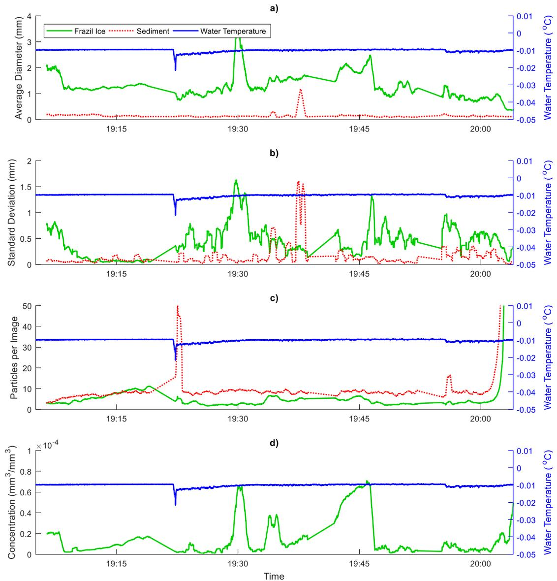
Figure 5-8: Time series data calculated over a period of 35 images for deployment KR-5. The variables plotted are a) the average particle diameter, b) the standard deviation of the diameter, c) the number of particles per image, and d) the volume concentration. The solid green line represents frazil ice particles, the red dotted line represents sediment particles, and the solid blue line is the water temperature.
