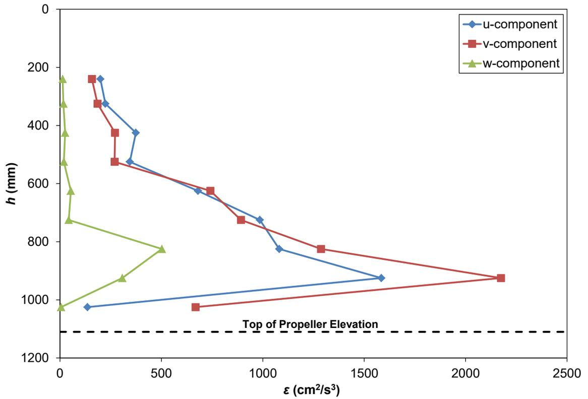
Figure 2-3: Turbulent kinetic energy dissipation rate ( $\epsilon$ ) throughout the water depth ( $h$ ), measured above the propeller for a speed of 325 rpm. The  $u$ ,  $v$ , and  $w$ -components represent the  $x$ ,  $y$ , and  $z$ -directions, respectively.
