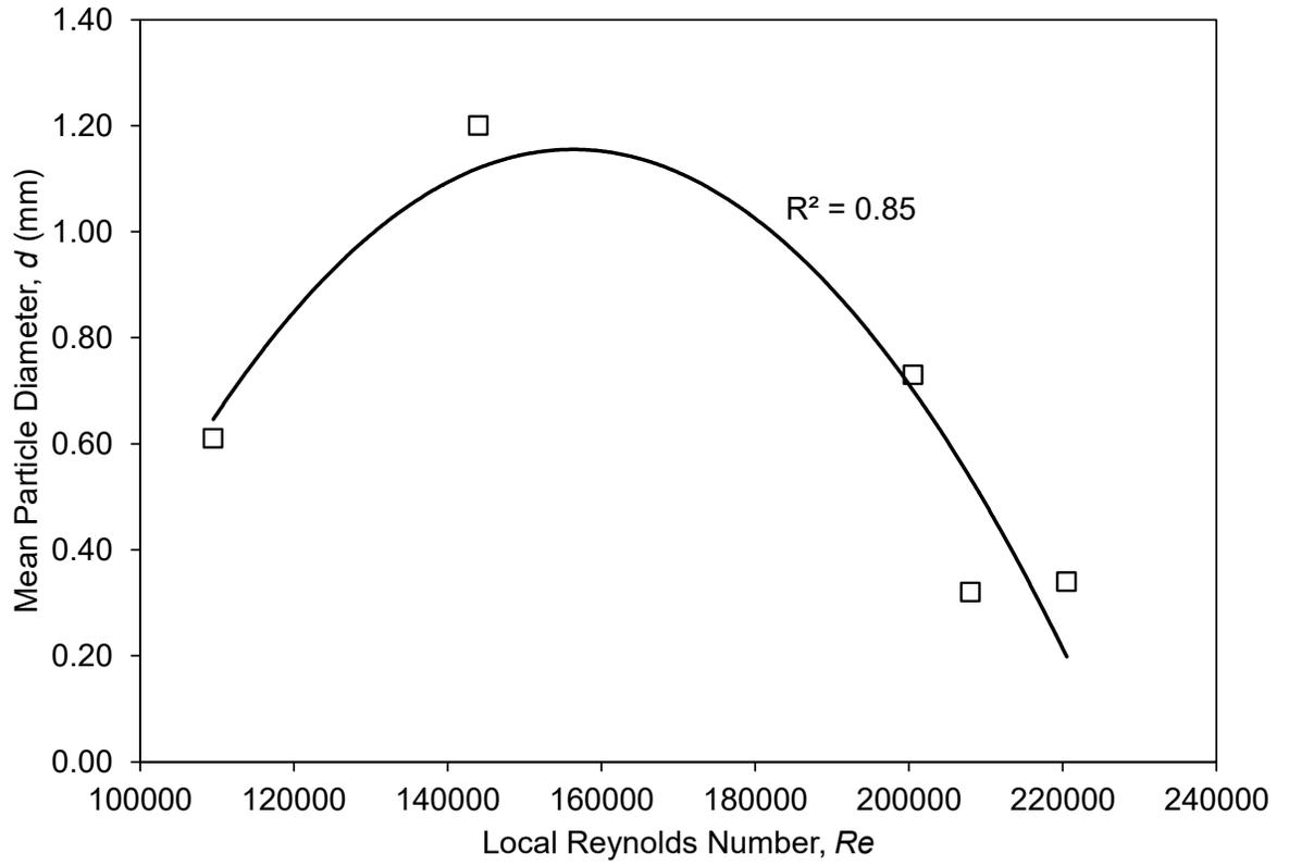
Figure 3-14: The mean frazil ice particle diameter plotted as a function of the local Reynolds number. The solid line is a second-order polynomial trendline.
