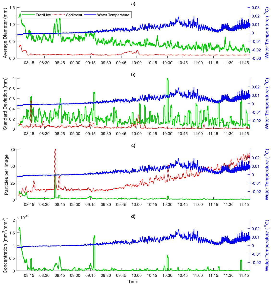
Figure 5-6: Time series data calculated over a period of 35 images for deployment KR-1. The variables plotted are a) the average particle diameter, b) the standard deviation of the diameter, c) the number of particles per image, and d) the volume concentration. The solid green line represents frazil ice particles, the red dotted line represents sediment particles, and the solid blue line is the water temperature.
