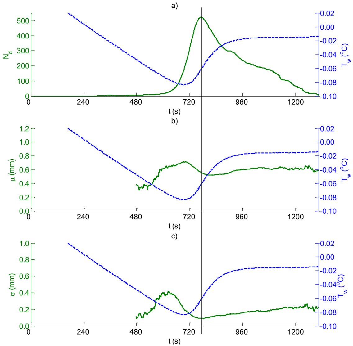
Figure 2-7: Time series of the 35 second moving average particle properties for the twelve 325 rpm experiments plotted along with the ensemble averaged supercooling curve,  $T_w$  (dashed line). a)  $N_d$ , the average number of particles observed in the 35 second window and summed over the 12 experiments, b) the mean particle diameter,  $\mu$ , and c) the standard deviation,  $\sigma$ . The black vertical line indicates the time at which the maximum number of particles were observed.
