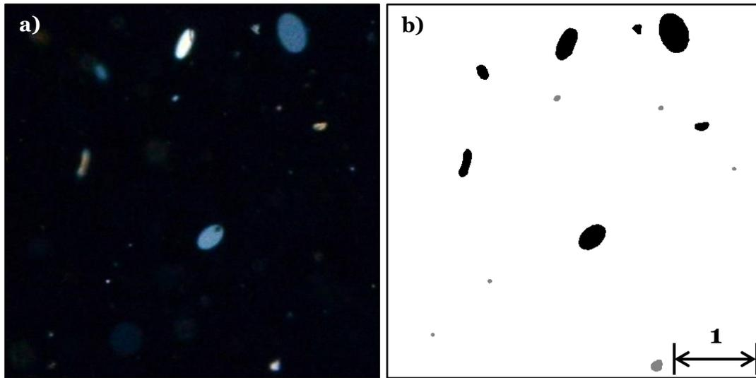
Figure 4-1: a) A small portion of a raw image captured in the Kananaskis River, and b) the SVM processed image where gray particles are sediment and black particles are ice. Note the small scale of the particles, with the largest particle being 0.5 mm in diameter.
