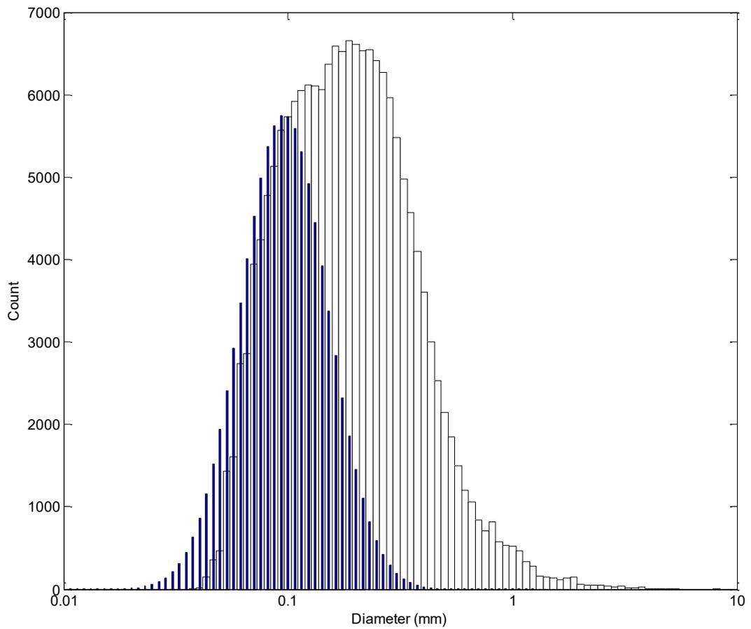
Figure 3-5: The raw size distribution of ice and sediment particles (white bars) at the Village Bridge site on the Kananaskis River March 1, 2015. The ensemble averaged randomly generated lognormal sediment size distribution (blue bars) computed using the mean and standard deviation of the sediment particles observed at the same site on March 2, 2015 is also shown.
