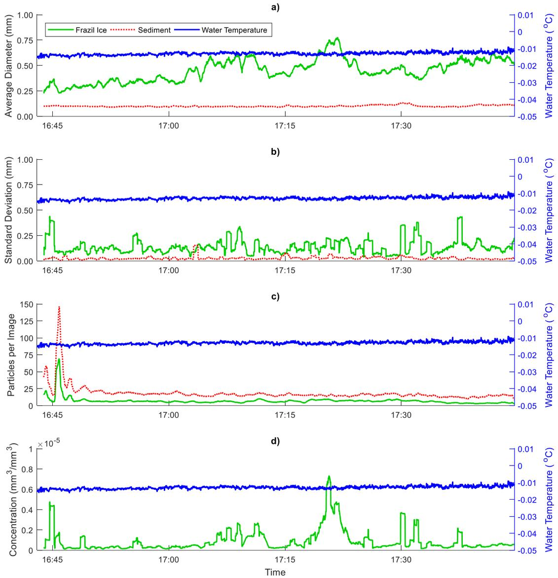
Figure 5-7: Time series data calculated over a period of 35 images for deployment PR-1. The variables plotted are a) the average particle diameter, b) the standard deviation of the diameter, c) the number of particles per image, and d) the volume concentration. The solid green line represents frazil ice particles, the red dotted line represents sediment particles, and the solid blue line is the water temperature.
