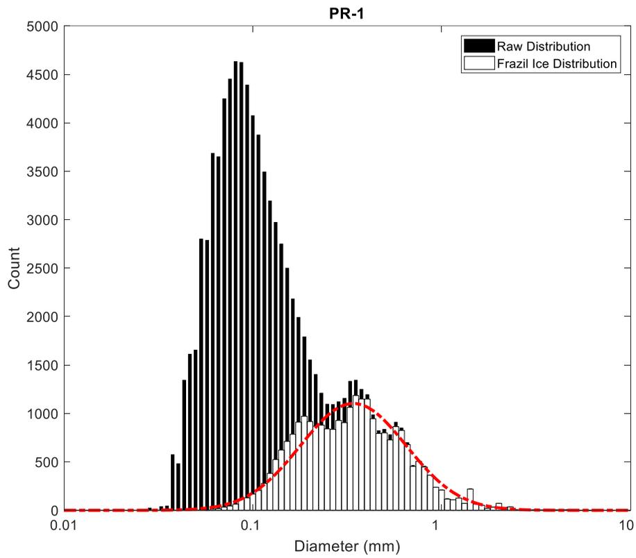
Figure 4-4: Comparison of the size distribution from deployment PR-1 before (black bars) and after (white bars) the SVM had been applied. The red dashed line indicates a lognormal distribution with the same mean and standard deviation as the observed particles.
