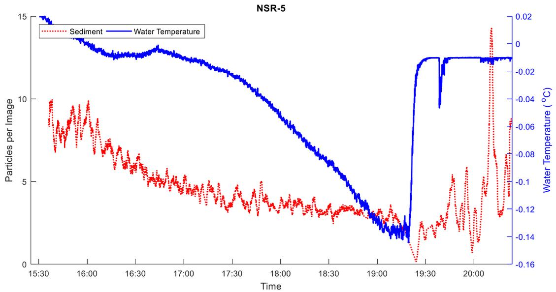
Figure 5-9: Time series data calculated over a period of 35 images for deployments NSR-5A and -5B. The number of sediment particles per image (red dotted line) and the water temperature (blue solid line) are plotted.
