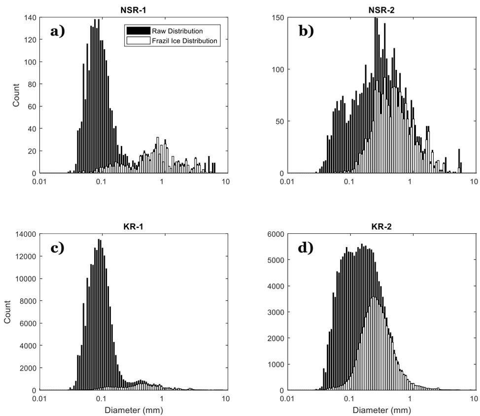
Figure 4-5: Comparison of the raw distributions to the frazil ice distributions obtained using the SVM for deployments a) NSR-1, b) NSR-2, c) KR-1, and d) KR-2.
