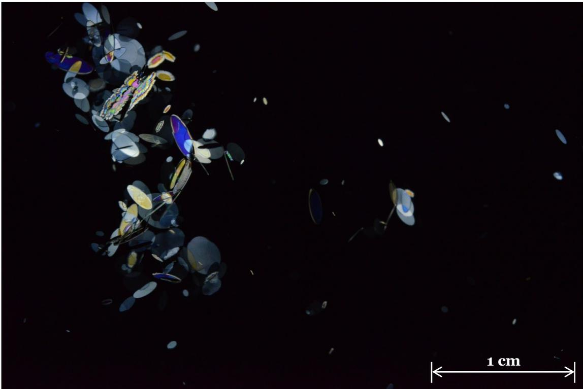
Figure 2-4: A sample unprocessed image, captured during one of the 225 rpm experiments, showing individual particles and a small frazil floc. The spacing between the polarisers was 2.2 cm.
