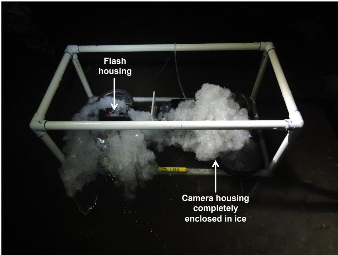
Figure 5-11: A large accumulation of shard-like anchor ice crystals on the FrazilCam following deployment NSR-5 on November 25, 2016. The flash (on the left) and the camera (on the right) are almost entirely covered in anchor ice.
