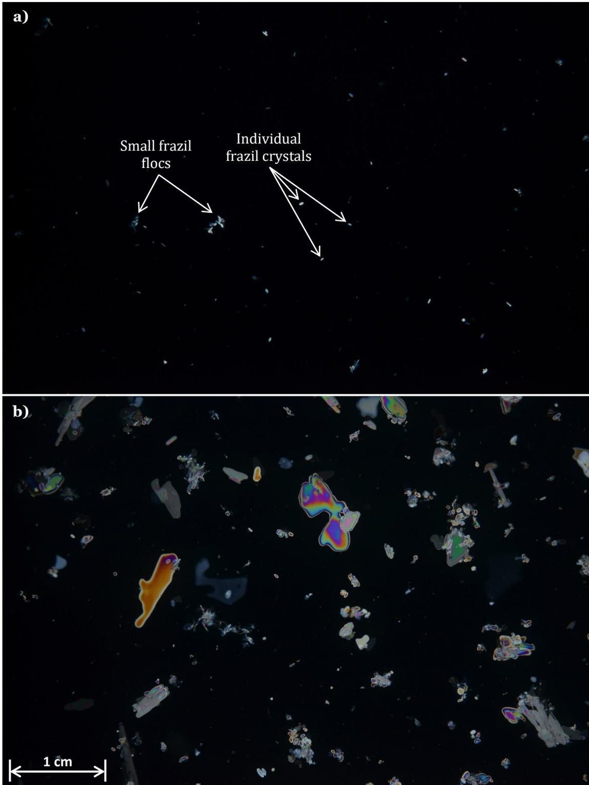
Figure 3-8: Two FrazilCam images captured in the North Saskatchewan River, November 27, 2014. a) Disc-shaped frazil particles and a few small flocs, and b) irregularly shaped ice particles observed in the flow.
