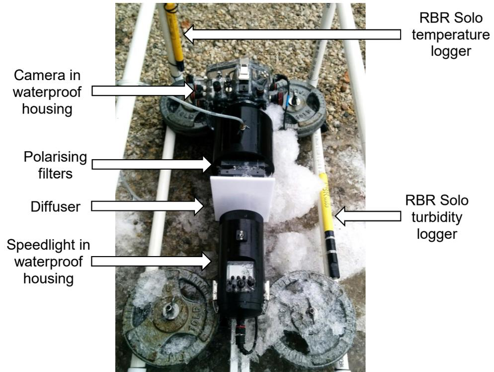
Figure 5-2: Top-down view of the FrazilCam after deployment in the North Saskatchewan River.
