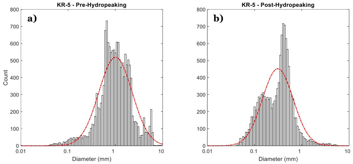
Figure 5-4: The frazil ice size distributions calculated a) before and b) after the hydropeaking event that occurred during deployment KR-5.
