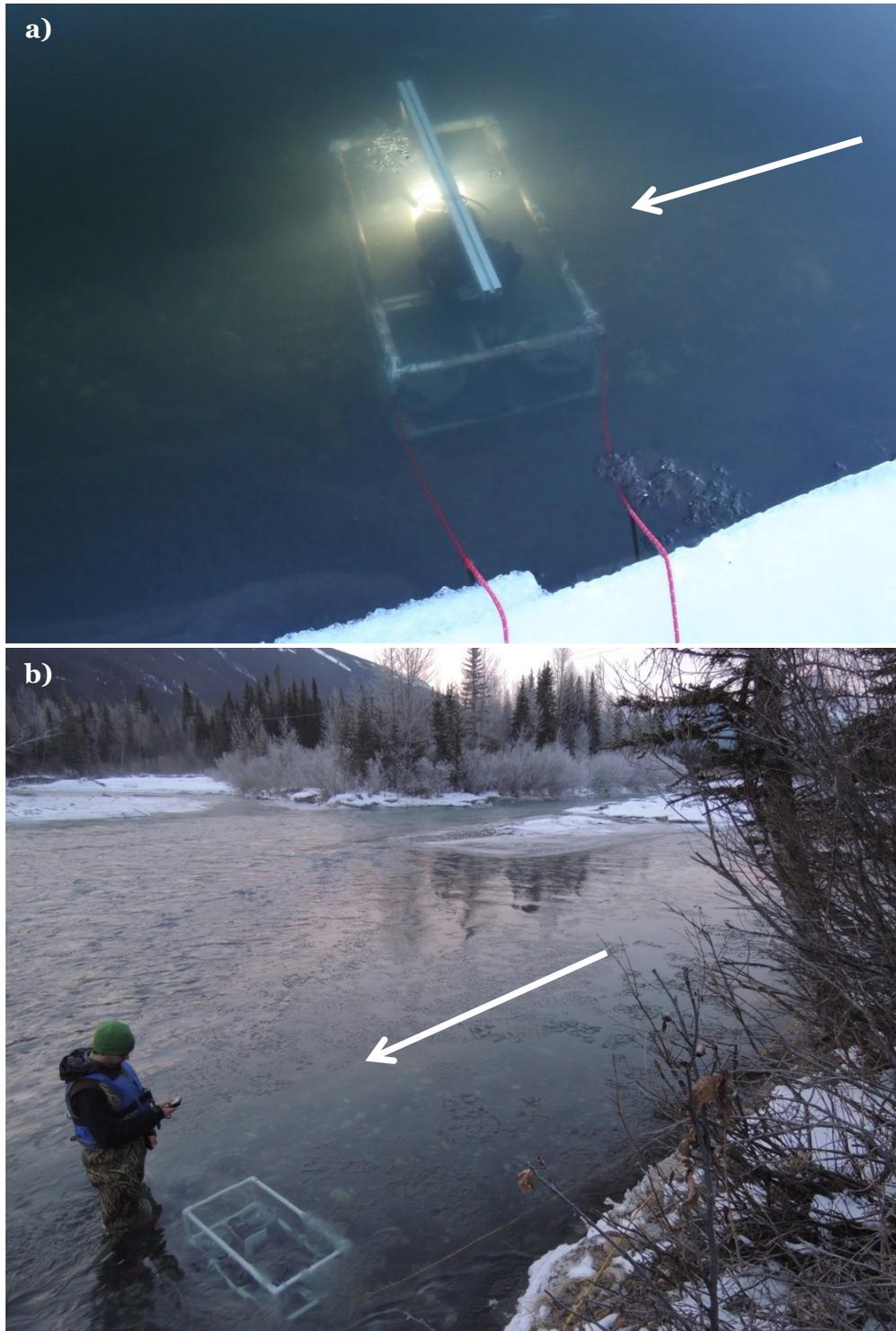
Figure 3-7: Digital image of the FrazilCam deployed a) at the Fairview site on the Peace River December 19, 2014 (photo credit: Martin Jasek), and b) at the Village Bridge site on the Kananaskis River March 1, 2015. Arrow indicates flow direction.
