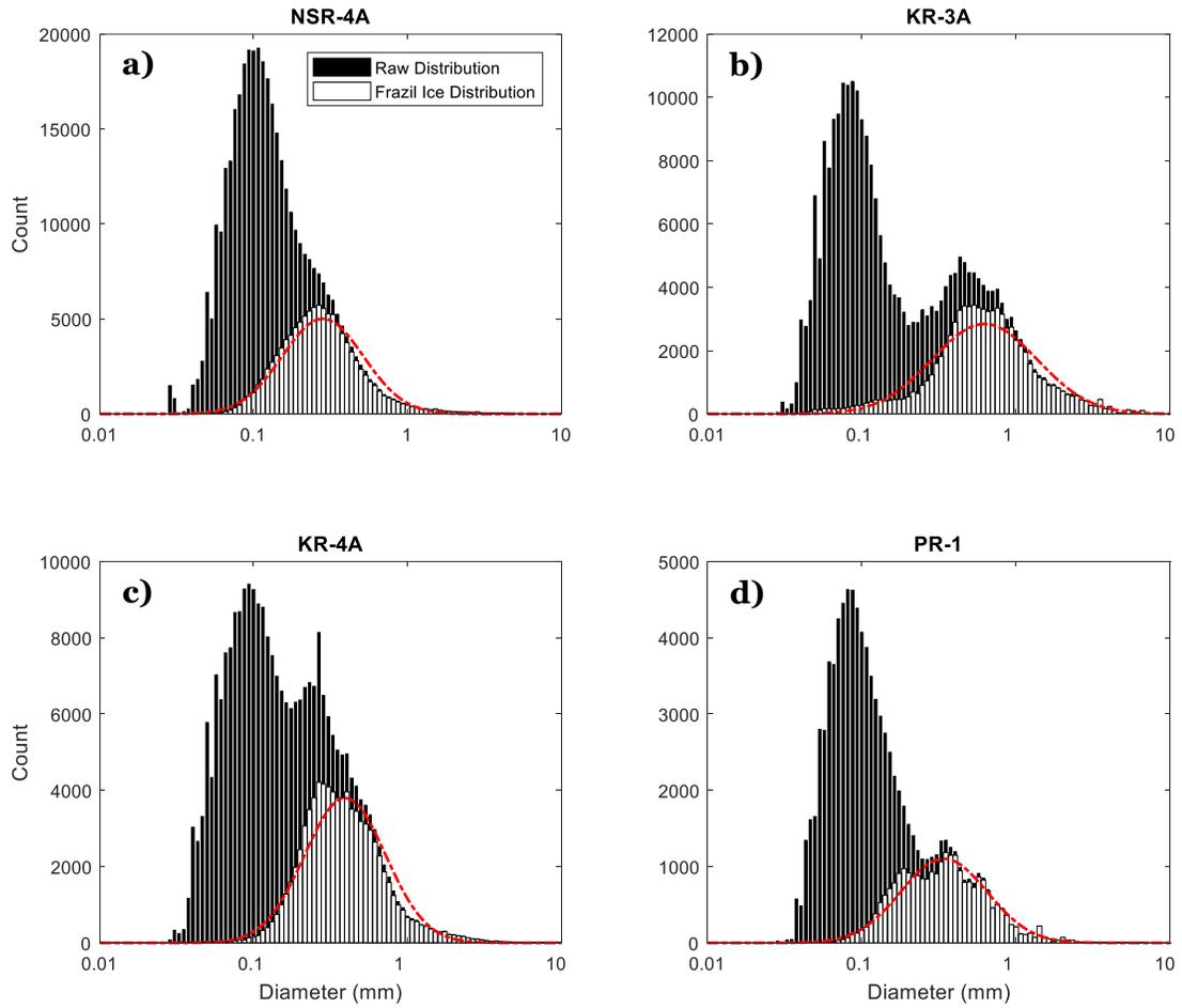
Figure 5-3: A comparison of the raw (black bars) and frazil ice (white bars) size distributions for deployments a) NSR-4A, b) KR-3A, c) KR-4A, and d) PR-1. The red dashed line indicates the lognormal distribution calculated with the same mean and standard deviation as the frazil ice distribution.
