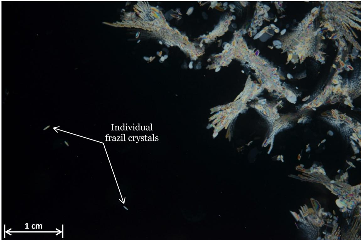
Figure 3-9: Raw digital FrazilCam image captured at the Fairview site on the Peace River on December 19, 2014. The irregularly shaped ice crystals concentrated on the right side of the image formed on the surface of the polariser nearest the camera lens as the camera was submerged.
