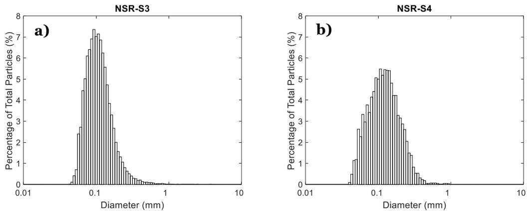
Figure 4-2: Comparison of the sediment size distributions observed during deployments a) NSR-S3 at Emily Murphy Park and b) NSR-S4 at the Quesnell Bridge. The different sediment distribution at the Quesnell Bridge site led to the creation of a site-specific SVM.
