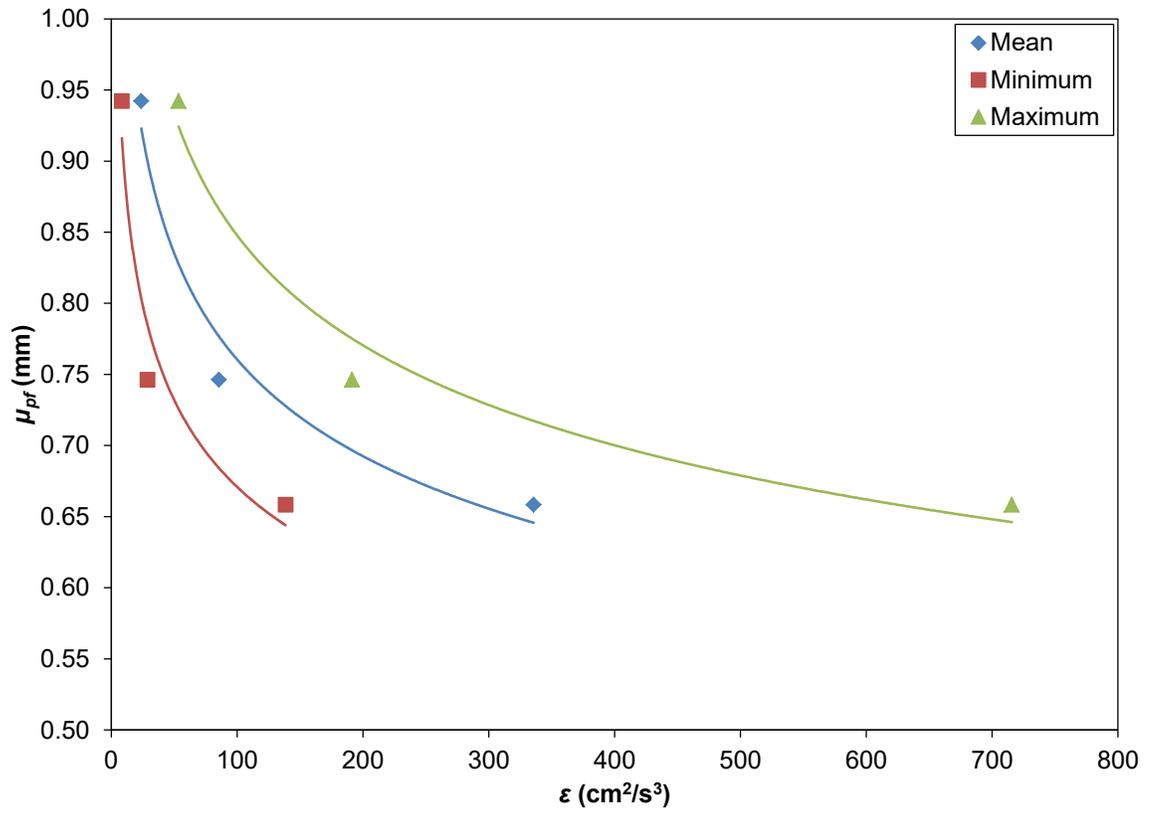
Figure 2-11: Mean pre-flocculation particle diameter,  $\mu_{pf}$ , plotted as a function of the depth-averaged turbulent kinetic energy dissipation rate,  $\epsilon$ .
