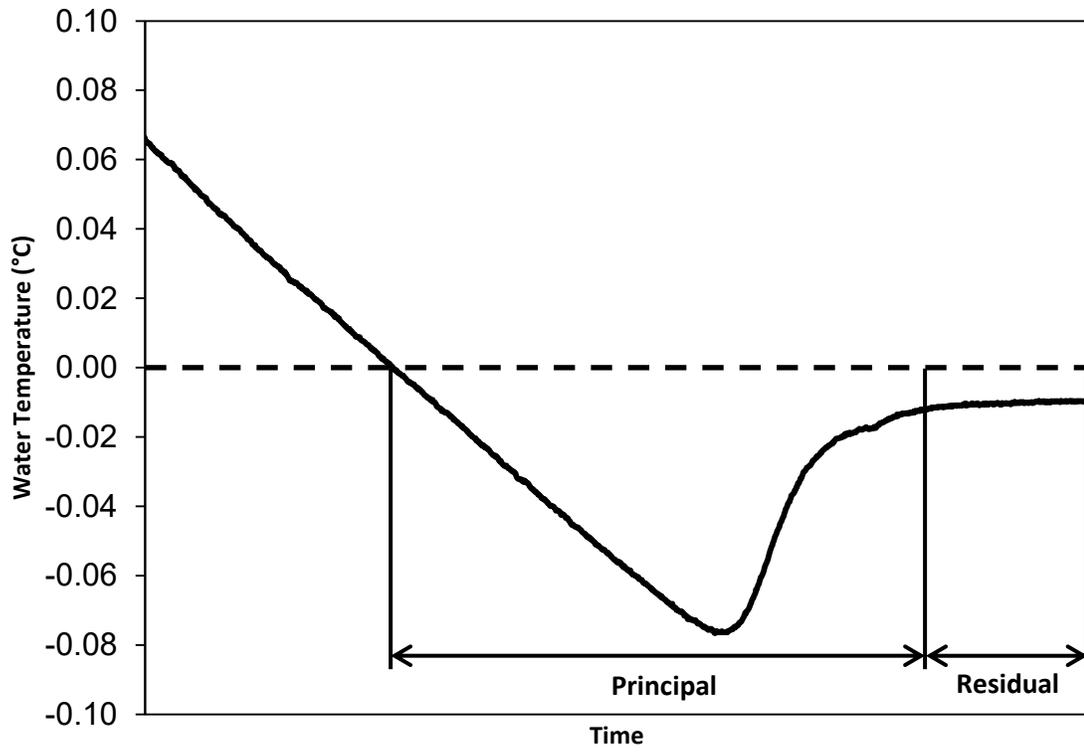
Figure 1-6: Illustration of a typical supercooling curve. The principal and residual supercooling phases are identified.
