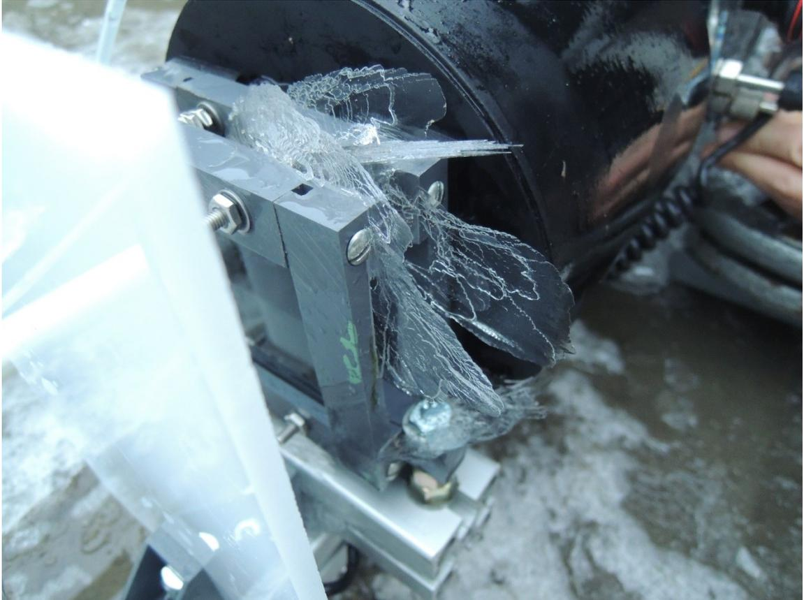
Figure 5-12: Shard-like crystals that grew off of the polariser frame during a FrazilCam deployment on November 20, 2016.
