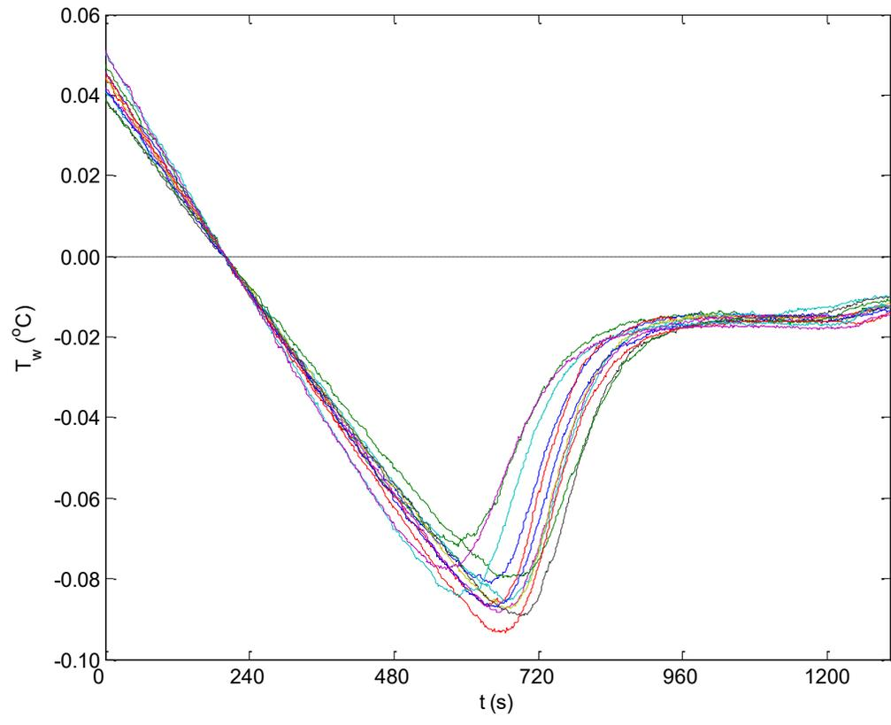
Figure 2-6: Superimposed supercooling curves showing the water temperature,  $T_w$ , as a function of time,  $t$ , for the 325 rpm experiments.
