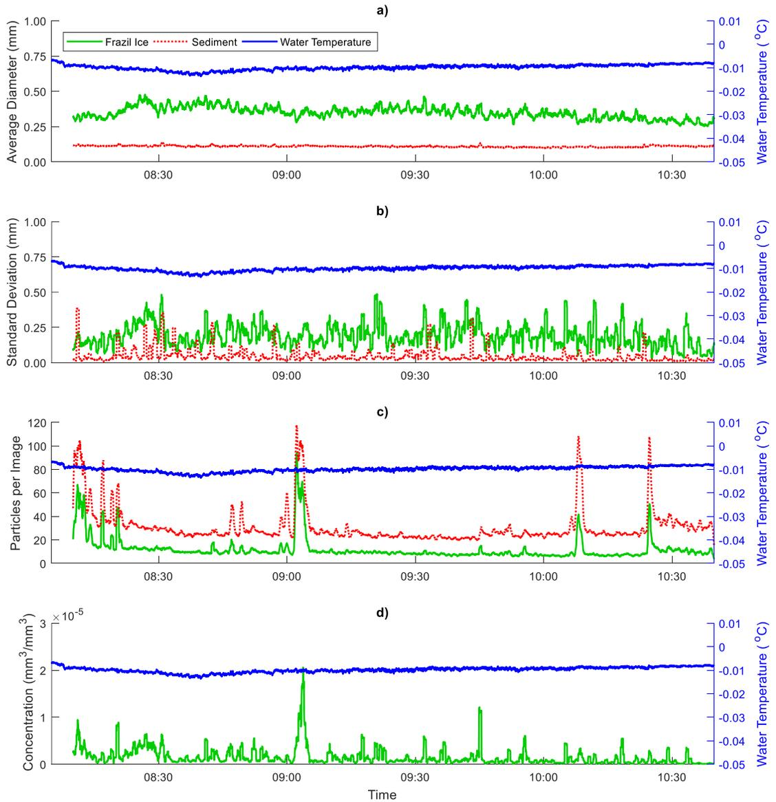
Figure 5-5: Time series data calculated over a period of 35 images for deployment NSR-4A. The variables plotted are a) the average particle diameter, b) the standard deviation of the diameter, c) the number of particles per image, and d) the volume concentration.
