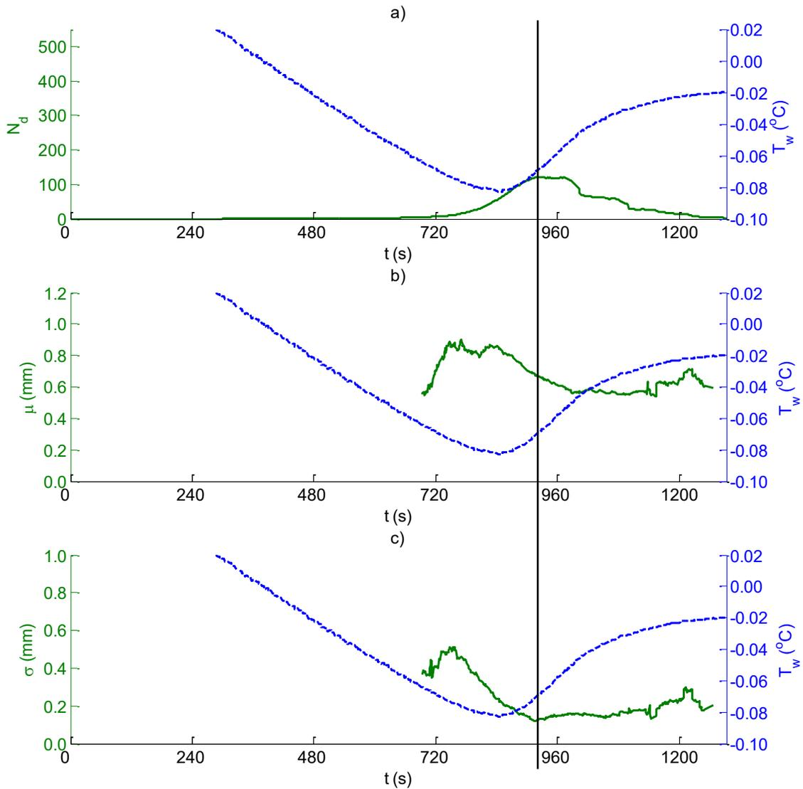
Figure 2-8: Time series of the 35 second moving average particle properties for the five 225 rpm experiments plotted along with the ensemble averaged supercooling curve,  $T_w$  (dashed line). a)  $N_d$ , the average number of particles observed in the 35 second window and summed over the 5 experiments, b) the mean particle diameter,  $\mu$ , and c) the standard deviation,  $\sigma$ . The black vertical line indicates the time at which the maximum number of particles were observed.
