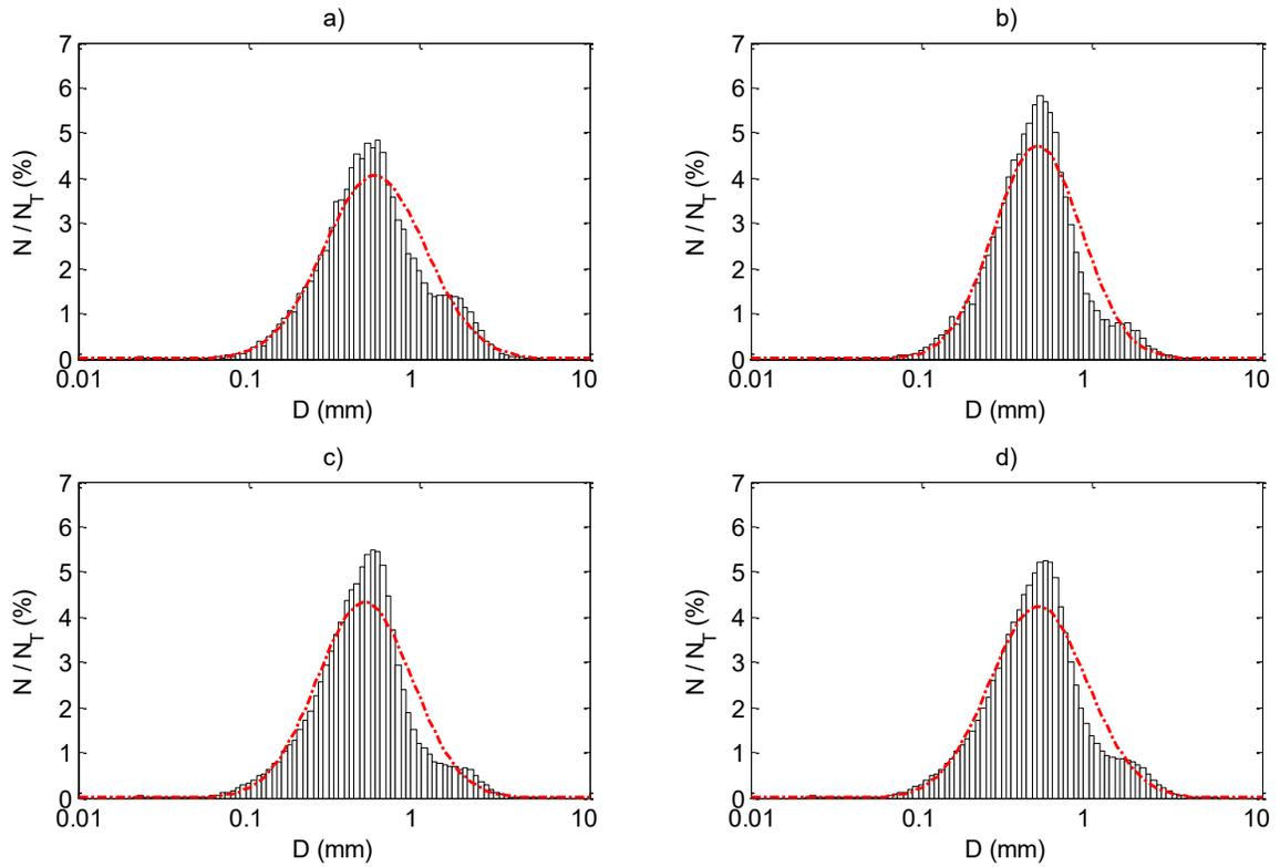
Figure 2-9: Ensemble size distributions at the 325 rpm propeller speed for a) the production range (i.e. from  $t_{10}$  to  $t_{90a}$ ), b) the peak range (i.e. between  $t_{90a}$  and  $t_{90b}$ ), c) the flocculation range (i.e. between  $t_{90b}$  and  $t_{30}$ ) and d) the entire data series.  $N$  is the number of particles in each bin,  $N_T$  is the total number of particles, and  $D$  is the diameter. The dot-dash lines are the corresponding lognormal distributions.
