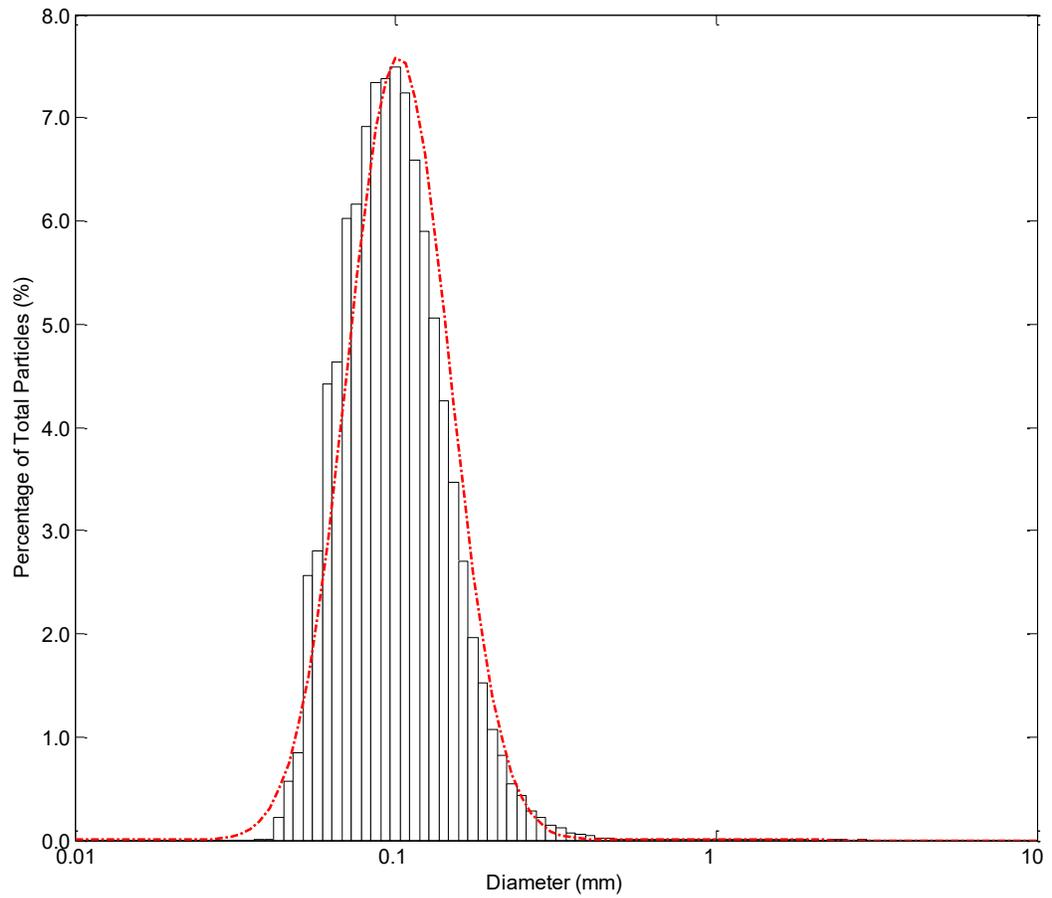
Figure 3-3: The size distribution of sediment particles observed at the Village Bridge on the Kananaskis River March 2, 2015. The dashed line represents the corresponding lognormal distribution calculated using the same mean and standard deviation as the measured size distribution.
