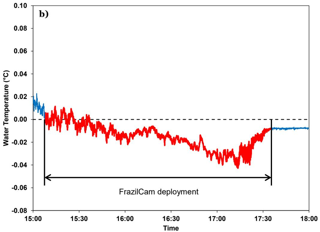
Figure 3-16: Time series of the water temperatures during the supercooling events observed at a) the Government House Park site, and b) the Quesnell Bridge site on the North Saskatchewan River, November 10, 2014.
