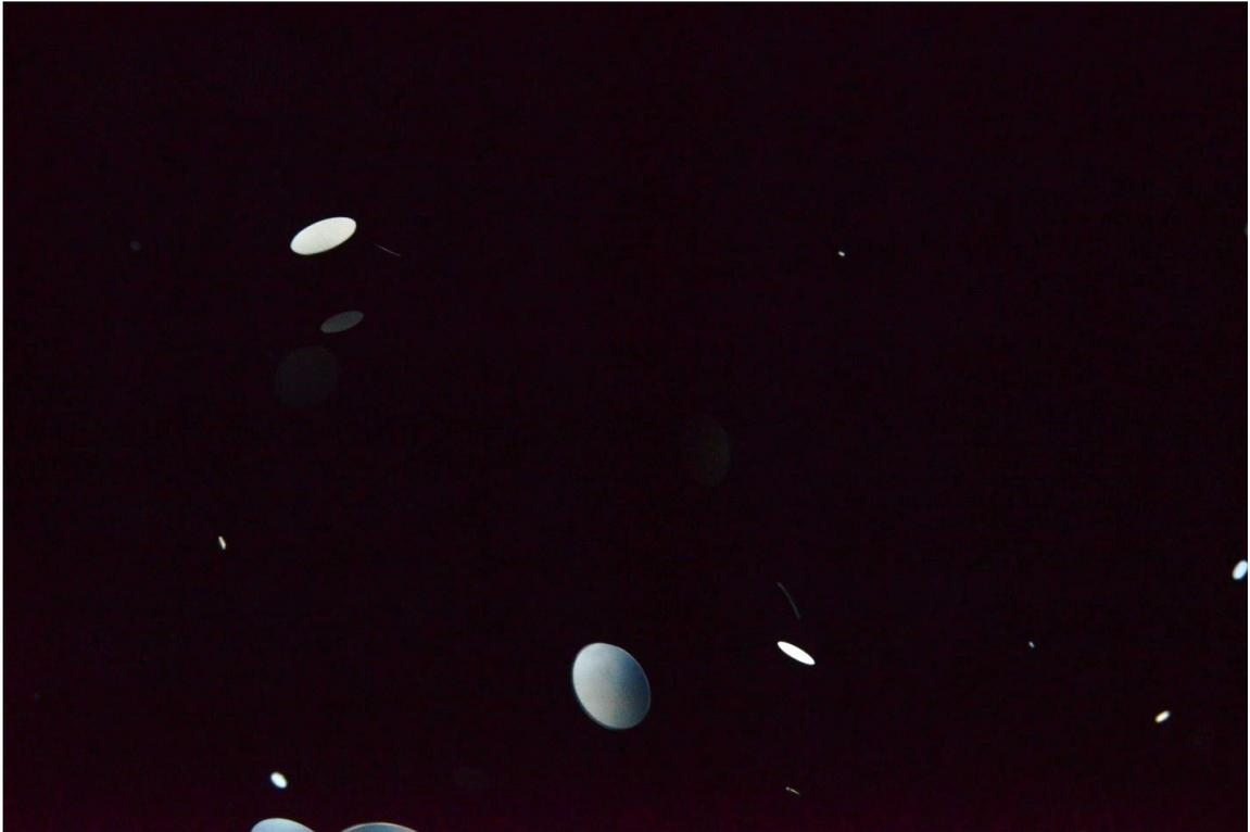
Figure 1-1: A digital image of frazil ice particles produced in the frazil ice tank in the University of Alberta cold room laboratory.
