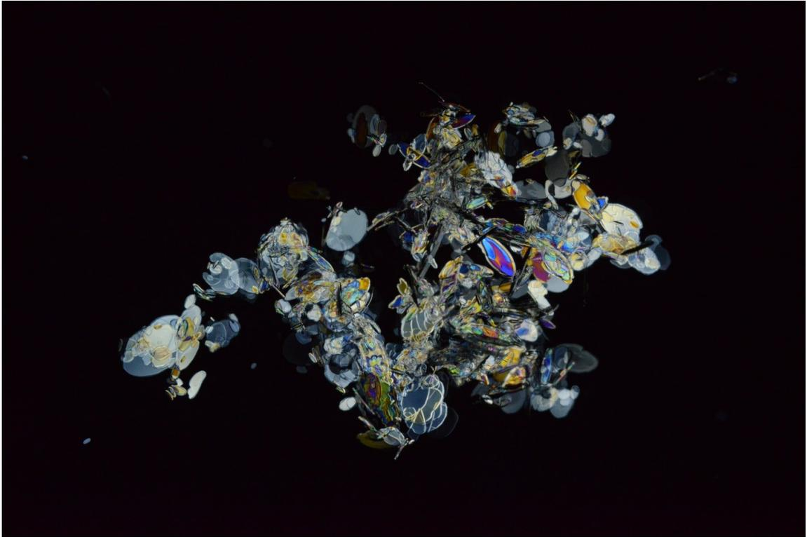
Figure 1-2: A digital image of a frazil ice floe produced in the frazil ice tank in the University of Alberta cold room laboratory.
