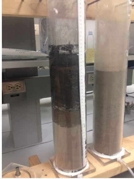
Figure 3-1 Soil columns for amendment and biochar study. The lower 20 cm was comprised of non-amended soil. Amendments were added to the top 10 cm of the soil.
