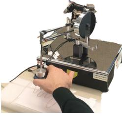
Fig. 3: Phantom Premium 1.5A Haptic Device in the squiggly line tracking task.
