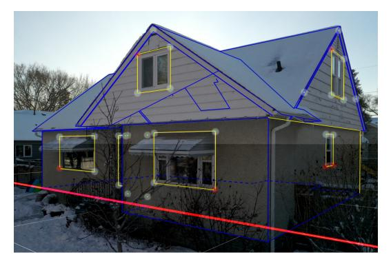
Figure 5.1: The total station points from the two visible elevations of building 1 (one station setup per side). The 6 red points are used for establishing scale.
