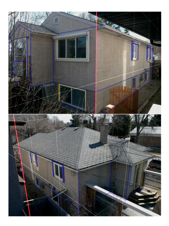
Figure 5.4: The two photos used to reconstruct building 3's east elevation. The red dots are the total station coordinates used to constrain the geometry, while the green dots are used to check the reconstruction.
