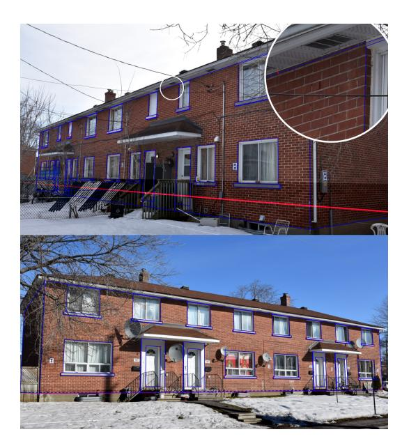
Figure 5.2: **Top:** The cluttered side of building 4. Also shown is a magnified view of several marked points (in red) demonstrating that they are actually lines showing the distance between the marked point (the edge in the image) and the model intersection line (blue). **Bottom:** The uncluttered side of building 4, which was reconstructed from two photos.
