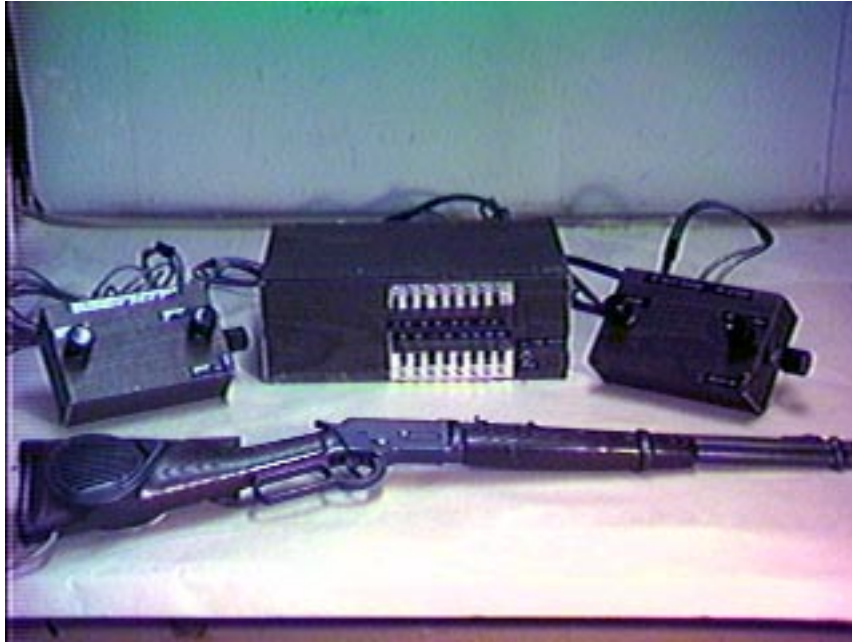
Figure 7. The ancestor of the computer mouse. Light guns, invented by Ralph H. Baer in 1967 were sold as point-and-shoot devices both for computerized and non-computerized arcade entertainment games. The gun was used by aiming at a CRT screen area. Source: Baer, Ralph H. "Inventions and Products," Ralph H. Baer (website). 19 Sept. 2009 < http://www.ralphbaer.com/ >.
