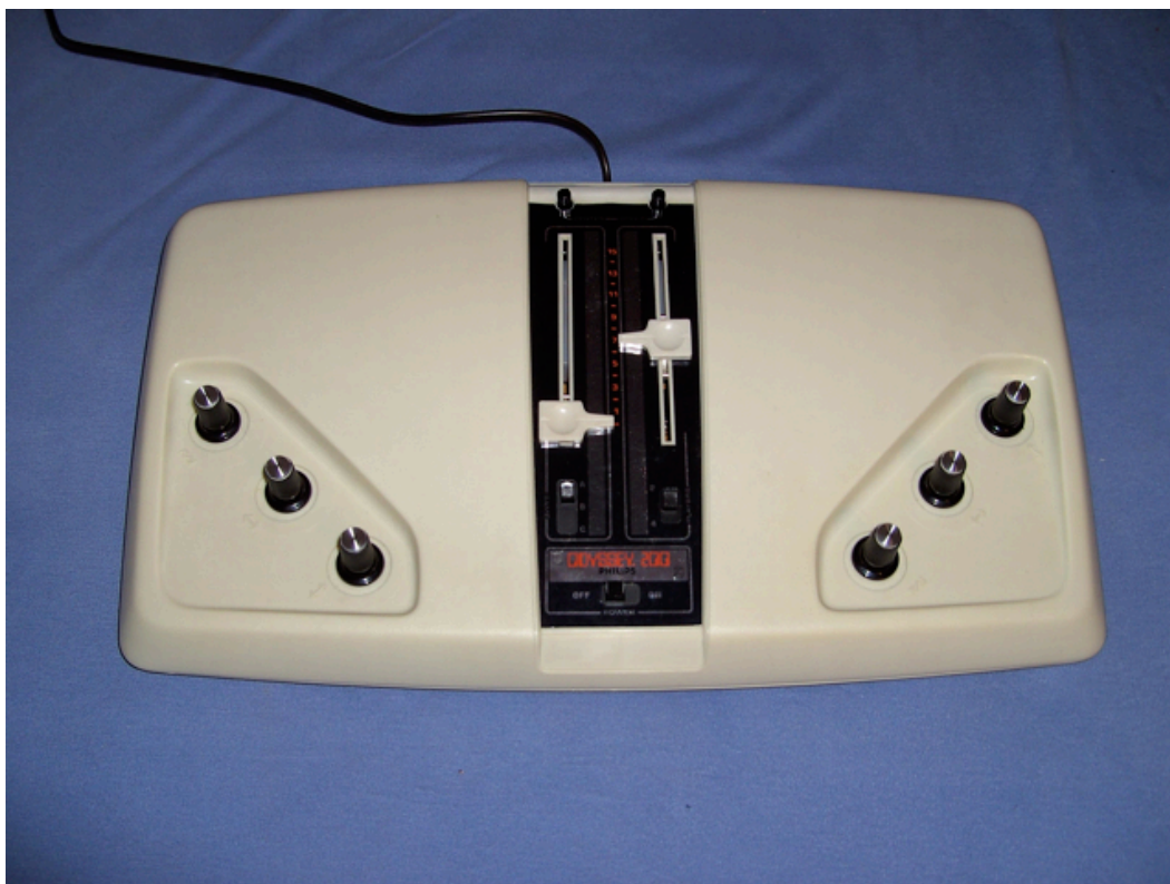
Figure 8. The Magnavox Odyssey 200 console featured two sliders to provide a manual scoreboard. Picture of a Magnavox Odyssey 200 console. In “Magnavox Odyssey 200,” Wikipedia Commons . 19 Sept. 2009 < http://en.wikipedia.org/wiki/File:ODYSSEY200_Konsole.JPG >.
