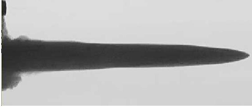
Figure 3.10: Side-view snapshot of rightward propagating front with  $N=1.40 \text{ s}^{-1}$ ,  $\rho_0=1.020 \text{ g/cm}^3$ ,  $Q_0=7.4 \text{ cm}^3/\text{s}$  and  $b_0=0.28 \text{ cm}$  at time  $t=90 \text{ s}$ .
