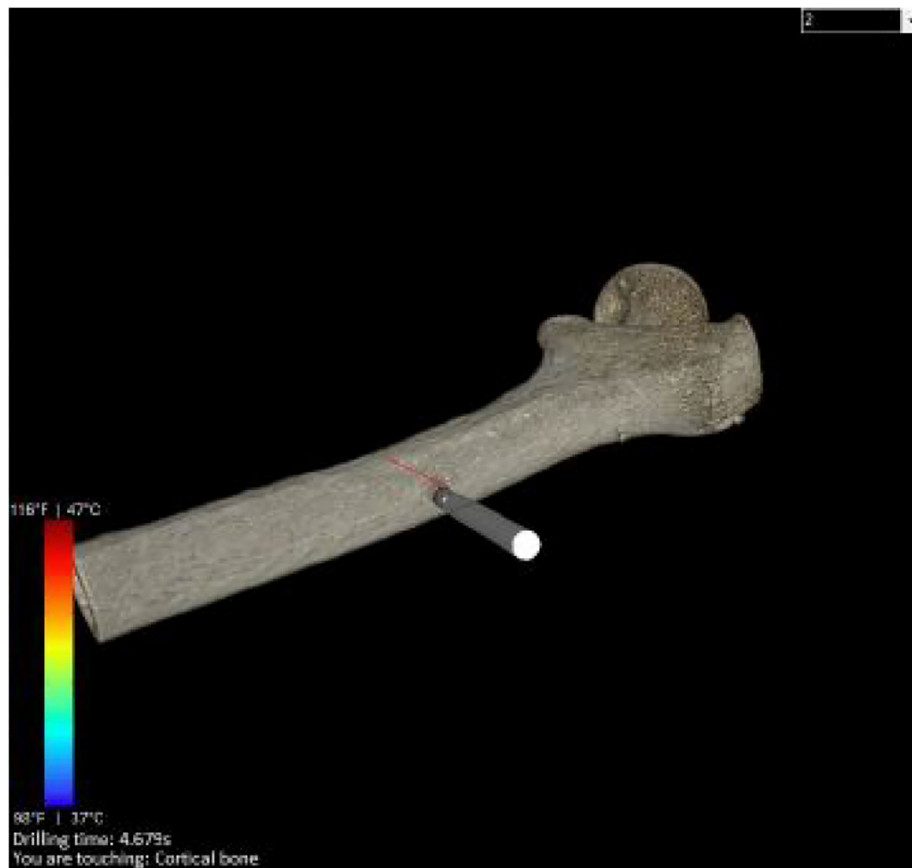
FIGURE 3 | The image shows a rendered bone obtained from the CT data. The user is able to touch or drill the shape, visually by moving the object stuck to the bone.
