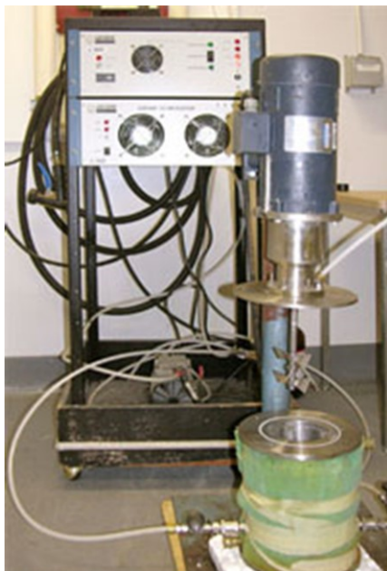
Figure 2A-5 Ozone generator, image from http://lipid.ualberta.ca
