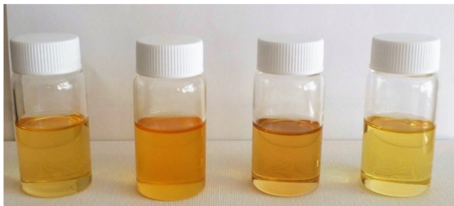
Figure 2A-3 Polyols produced from flax and canola oils, from left to right: canola oil polyol route C, flax oil polyol route C, flax polyol route B, and flax fame polyol route A, See Figure 7-2 .
