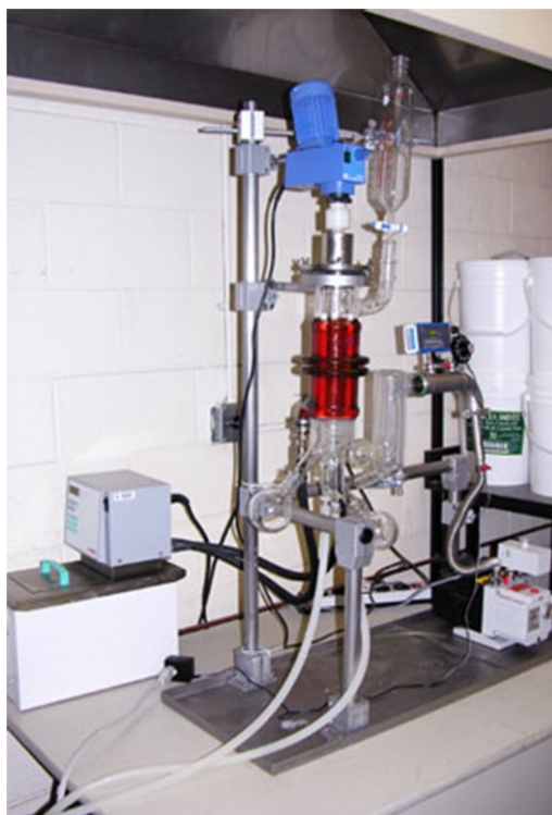
Figure 2A-6 Wiped Film Evaporator (WFE), image from http://lipid.ualberta.ca
