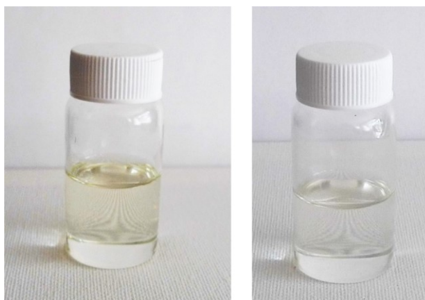
Figure 2A-2 Epoxidized Flax (left) and epoxidized canola (right) oils (at room temperature). Epoxidized canola oil crystallizes after few days.
