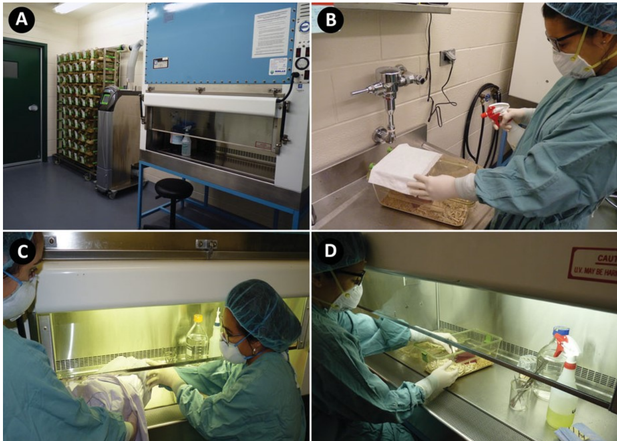
Figure 2.2 Cage changing and sampling protocol. (A) Animal room with a Class 2A biological safety cabinet (BSC), Tecniplast® Green Line Sealsafe Plus individually ventilated cages (IVCs) in an IVC rack attached to a high efficiency particulate air handling unit operated in containment mode. (B) The assistant spraying Clidox® onto the IVC surface while covering the cage filter with a sterile towel. (C) The assistant aseptically handing the cage to the primary individual for placement of the IVC within the BSC (the assistant does not handle the cage by its inner sterile wrap, and both individuals wear sterile gloves and surgical gowns). (D) The primary individual collecting samples from the cage after the GF-mouse has been transferred to a replacement sterile cage and it has been returned to the IVC rack by the assistant.
