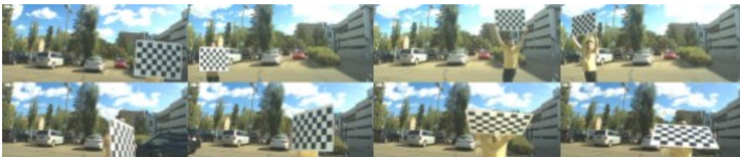
Figure 4.3: Stereo camera intrinsic and extrinsic calibration using checkerboards.
