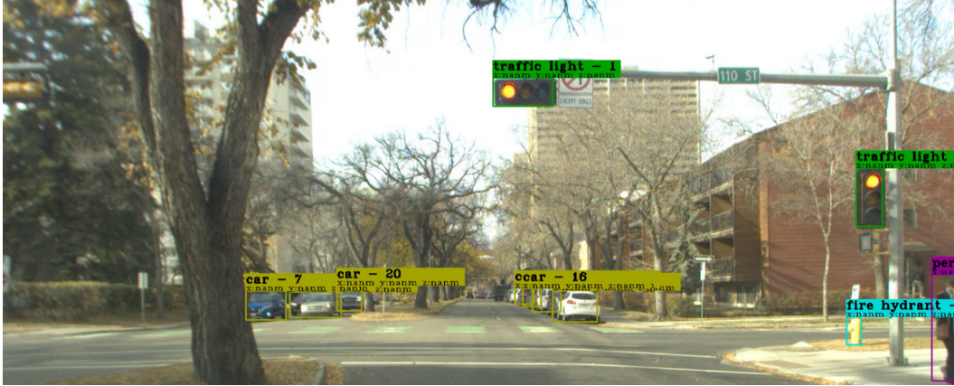
Figure 4.2: Bounding box detections for several classes in the COCO dataset. The potentially dynamic classes will be picked from all the detections based on their class number. These objects include cars, trucks, buses, pedestrians, cyclists, and motorbikes.
