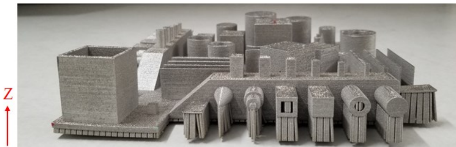
Figure 30. GBTA after the removal of the base plate. a) Isometric view, b) Side view showing warped features
