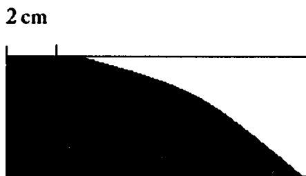
Figure 4.9: Visual observation of asphalt-in-water emulsion plug advance into core 3
