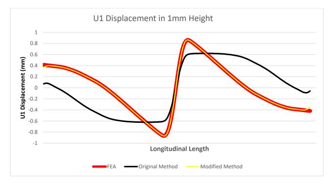
Fig. 17 U1 Displacement in the longitudinal direction in 1mm Height
