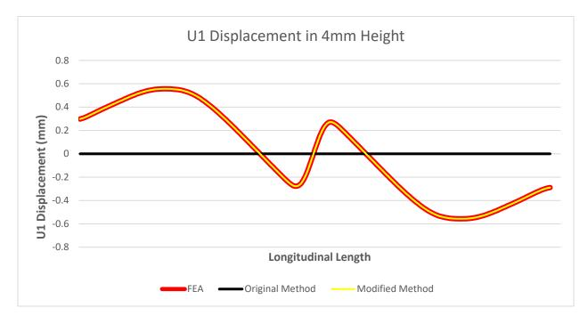
Fig. 20 U1 Displacement in the longitudinal direction in 4mm Height
