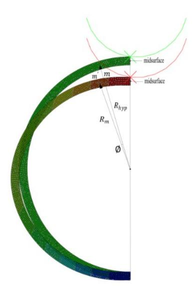
Fig. 39 displacement along the circumferential direction
