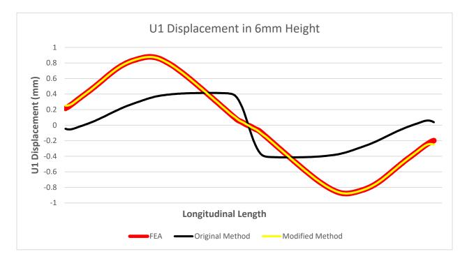
Fig. 22 U1 Displacement in the longitudinal direction in 6mm Height
