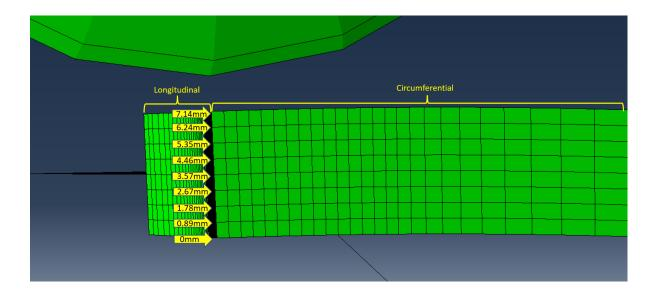
Fig. 37 3D model of wall thickness in the circumferential direction
