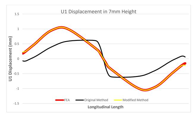
Fig. 23 U1 Displacement in the longitudinal direction in 7mm Height
