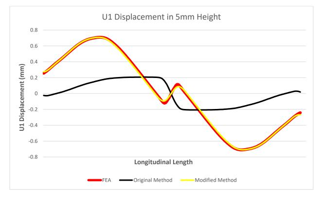
Fig. 21 U1 Displacement in the longitudinal direction in 5mm Height
