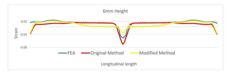
Fig. 33 Plots of the LE11 in the longitudinal direction in the 6 mm height of the pipe
