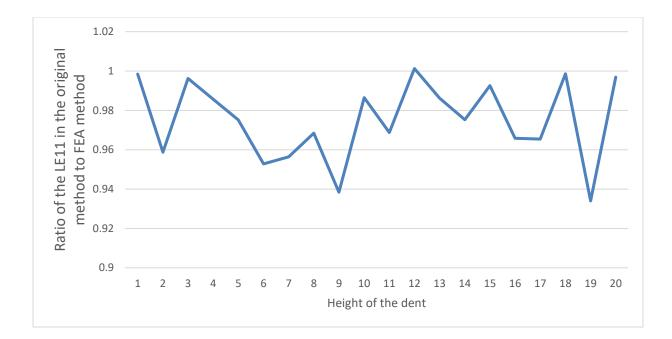
Fig. 43 Ratio of the LE11 in the bottom of the pipe in the e circumferential direction in 2D
