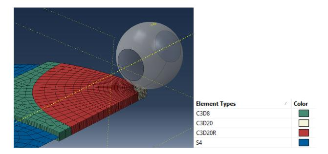
Fig. 9-b Element types in 3D direction
