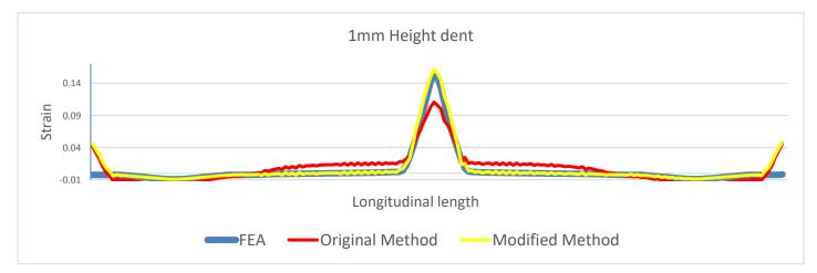
Fig. 28 Plots of the LE11 in the longitudinal direction in the 1 mm height of the pipe
