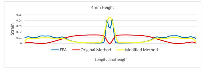
Fig. 31 Plots of the LE11 in the longitudinal direction in the 4 mm height of the pipe
