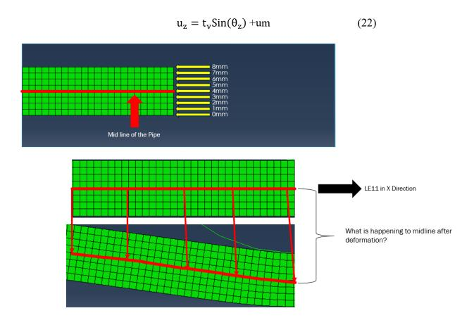
Fig. 14 displacement in the mid-line of the pipe in the longitudinal direction where  $u_m$  and  $t_v$  indicate the displacement of the mid surface in the deformed pipe and the coordinate normal to the mid surface of the pipe, respectively. Additionally, t and  $t_v$  are the
