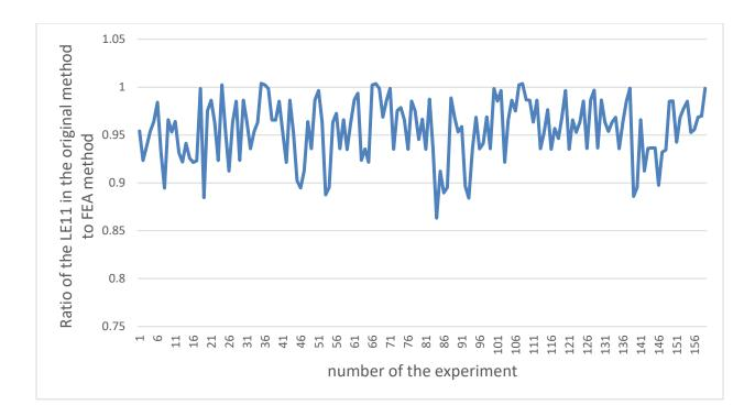
Fig. 41 Ratio of the LE11 in the top of the pipe in the circumferential direction in 3D model
