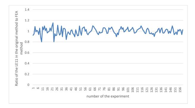
Fig. 42 Ratio of the LE11 in the bottom of the pipe in the circumferential direction in 3D model
