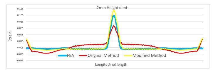
Fig. 29 Plots of the LE11 in the longitudinal direction in the 2 mm height of the pipe
