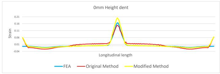
Fig. 27 Plots of the LE11 in the longitudinal direction in the 0 mm height of the pipe
