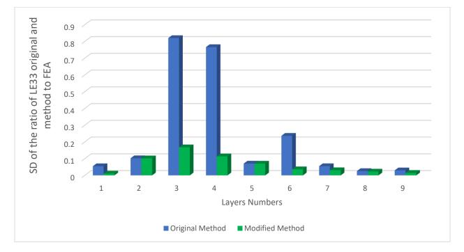
Fig. 26 The standard deviation ratio of the LE33 in modified and original method to FEA
