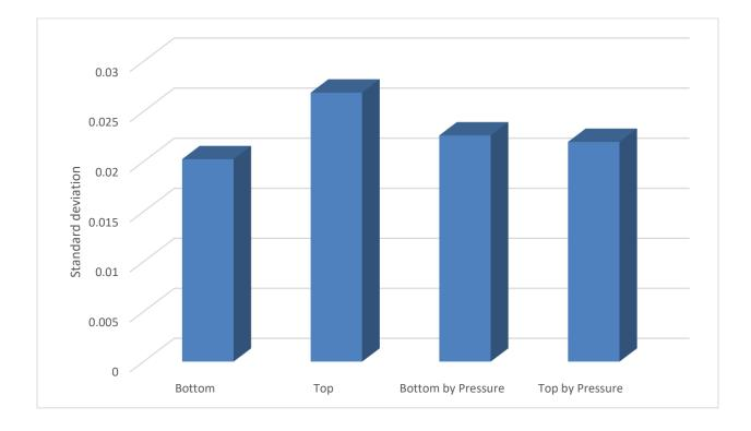
Fig. 50 Standard deviation of the LE11 in the circumferential direction in 2D model
