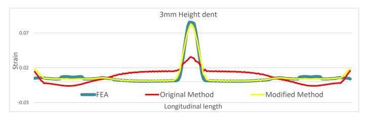
Fig. 30 Plots of the LE11 in the longitudinal direction in the 3 mm height of the pipe
