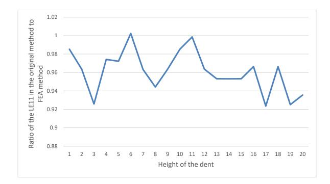
Fig. 45 Ratio of the LE11 in the bottom of the pipe in the circumferential direction in 2D
