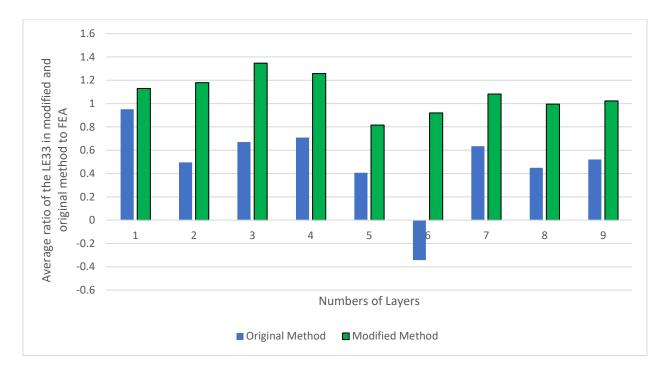
Fig. 25 The average ratio of the LE33 in modified and original method to FEA method
