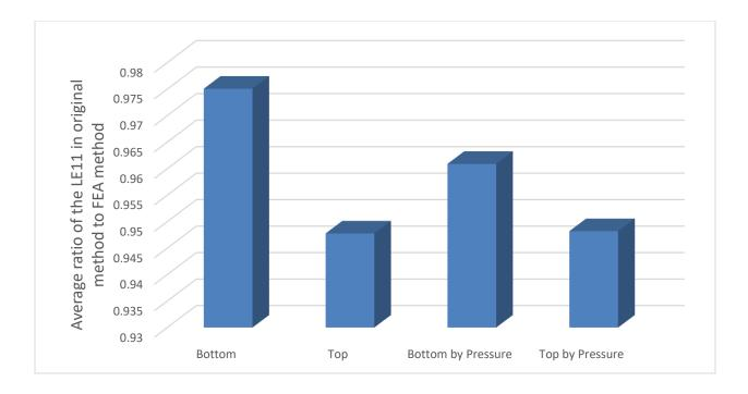
Fig. 49 Average ratio of the LE11 in the circumferential direction in 2D model
