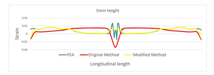
Fig. 32 Plots of the LE11 in the longitudinal direction in the 5 mm height of the pipe
