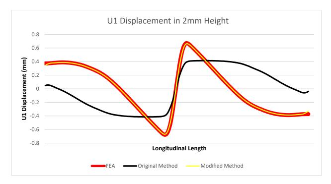
Fig. 18 U1 Displacement in the longitudinal direction in 2mm Height
