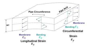
Fig. 1 Strain components in the pipe wall
