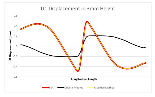
Fig. 19 U1 Displacement in the longitudinal direction in 3mm Height
