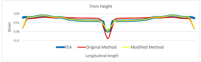
Fig. 34 Plots of the LE11 in the longitudinal direction in the 7 mm height of the pipe
