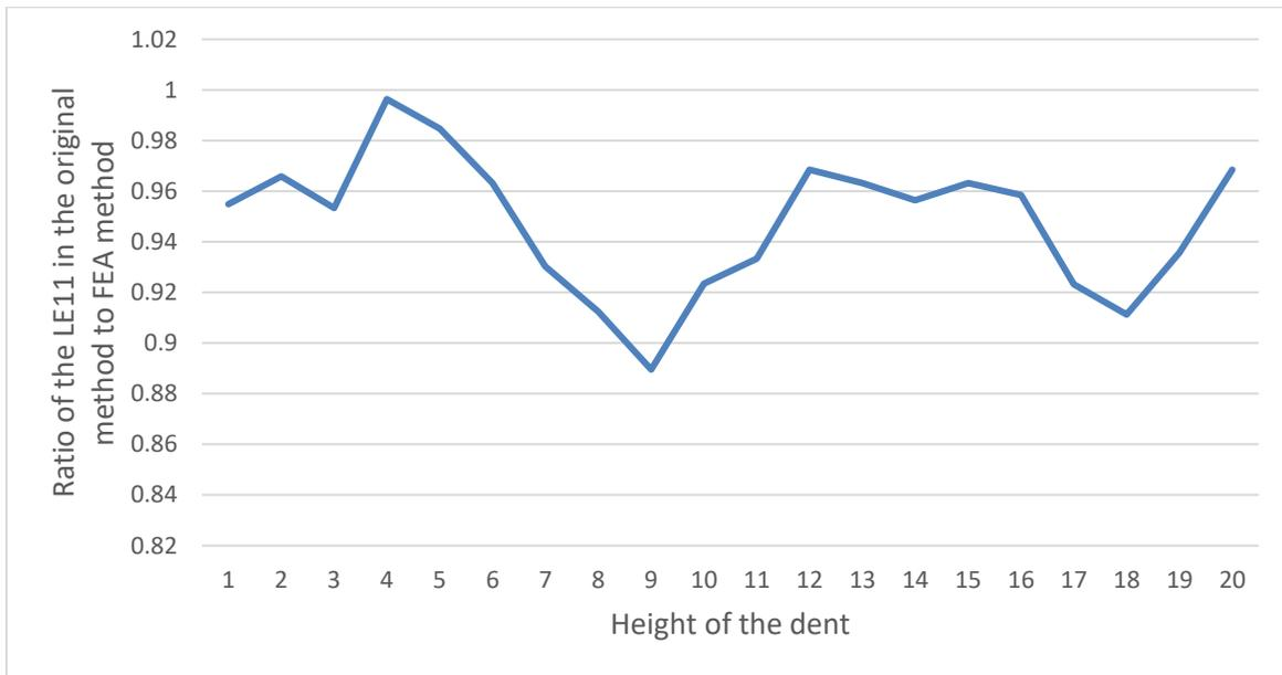
**Fig. 44 Ratio of the LE11 in the top of the pipe in the circumferential direction in 2D model with pressure**
