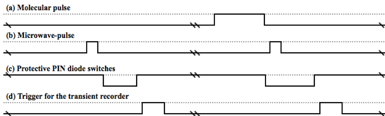
Figure 2.3.2 A typical pulse sequence programmed in the cavity-based FTMW spectrometer.
