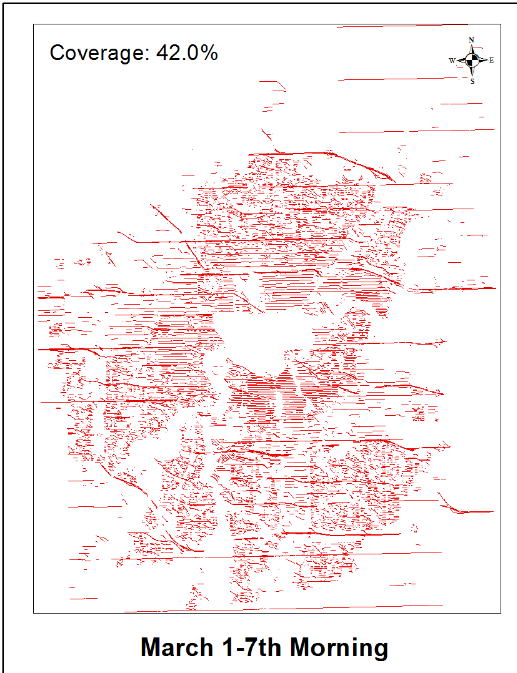
Figure A. 2 Glare prone locations of morning glare period in March 1-7th
