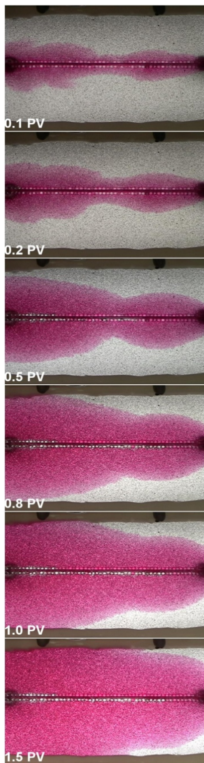
Figure 3.6 Horizontal light mineral oil (white) displacement at 15 ml/hr with water wet sample.
