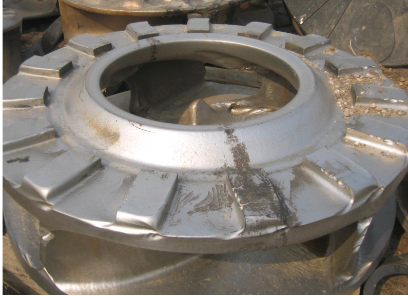
Figure 1.1: A damaged slurry pump impeller (provided by Syncrude Canada Ltd.)
