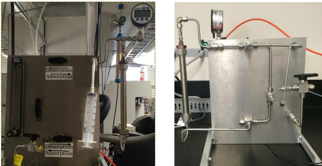
**Figure 7.2: Multicomponent Adsorption/Desorption test stand. Left picture shows front of the set-up and right one displays the rear of the set-up.**
