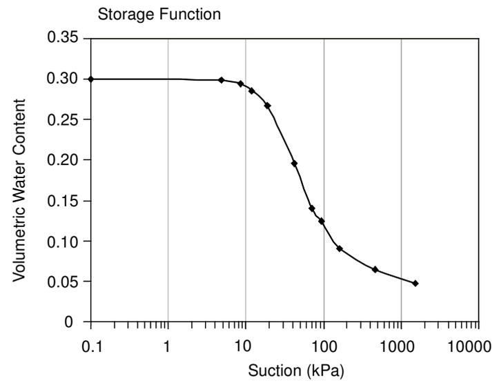
Figure 4.8. Hydraulic conductivity function and storage function for glacial till in Slide CN50.9.
