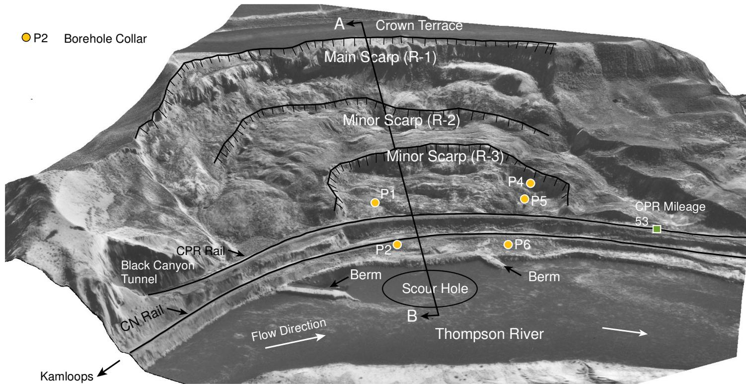
Figure A1.2 A 3-dimensional view of the South Slide with its three scarps, scour hole at the Thompson River bed, borehole locations, and cross-section line. The slide is 600 metres wide at the river level.
