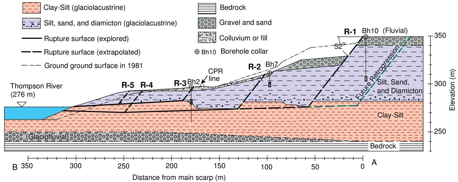
Figure 4.16. Cross section after the Goddard 1982 reactivation showing borehole and piezometer locations, ground profile before the Goddard 1982 reactivation, the CPR rail line, five translational blocks, and the stratigraphy of the slide (see Figure 1 and Figure 15 for location of the section).
