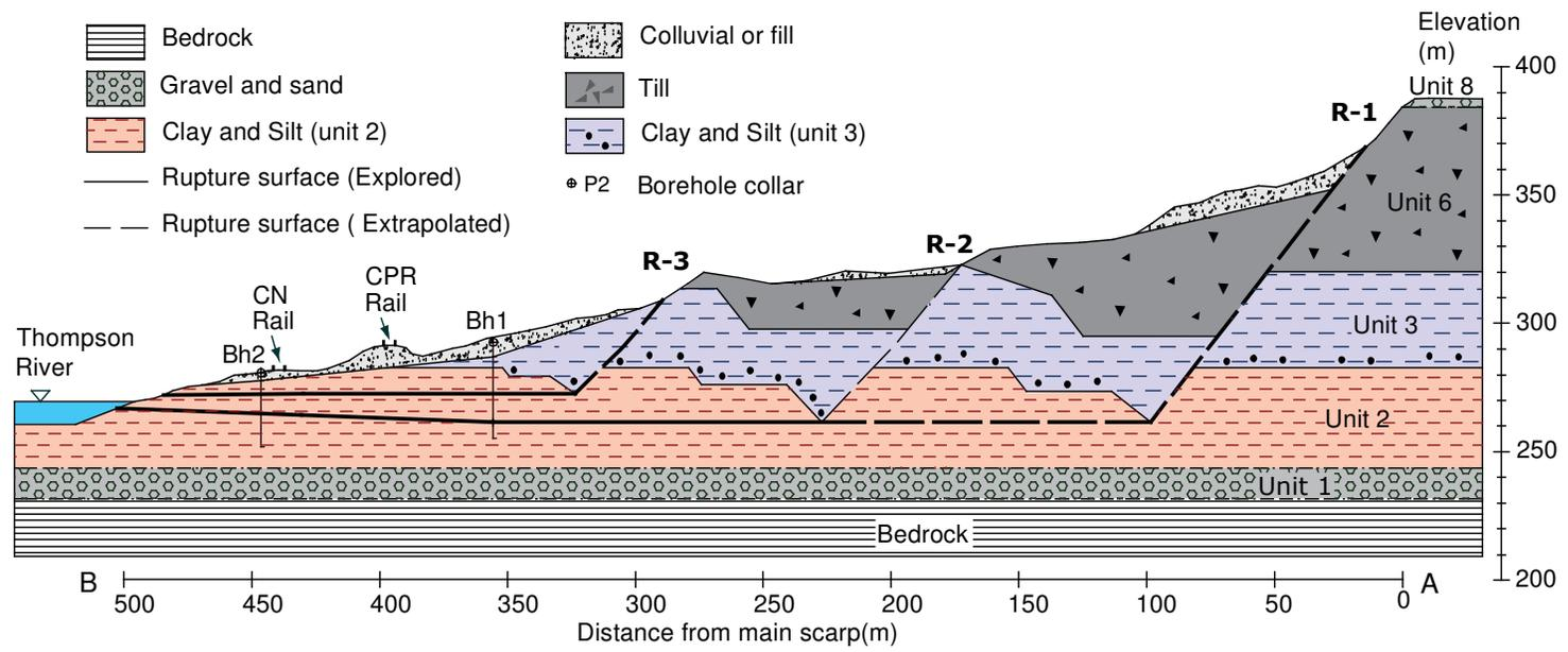
Figure 3.20. Cross section through the South Slide.
