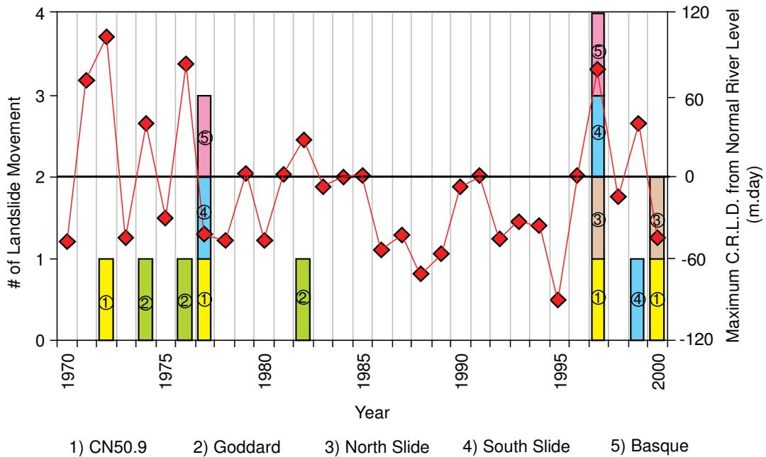
Figure 4.2. Correlation between the annual Thompson River's maximum Cumulative River Level Difference from its normal river level and slides in Ashcroft area with a noticeable increase in their rate of movement.
