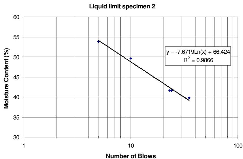
Figure A3.12 Liquid limit curve for specimen 2.
