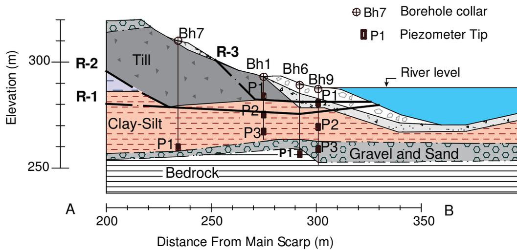
Figure 4.5.B. Piezometers installed at the Slide CN50.9 toe.
