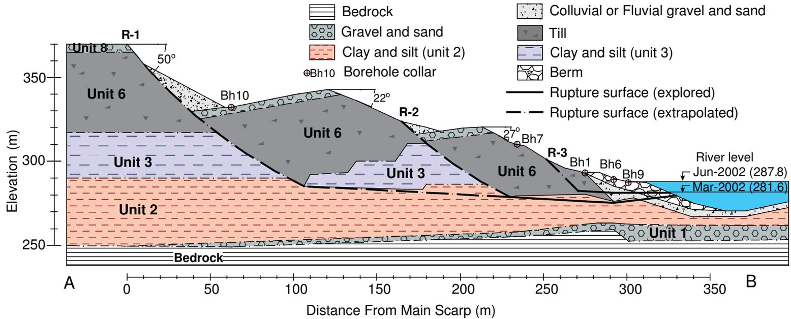
Figure 3.10. Cross section through Slide CN50.9 showing rupture surfaces, stratification, and borehole locations (see Figure 3.10 for cross-section position).
