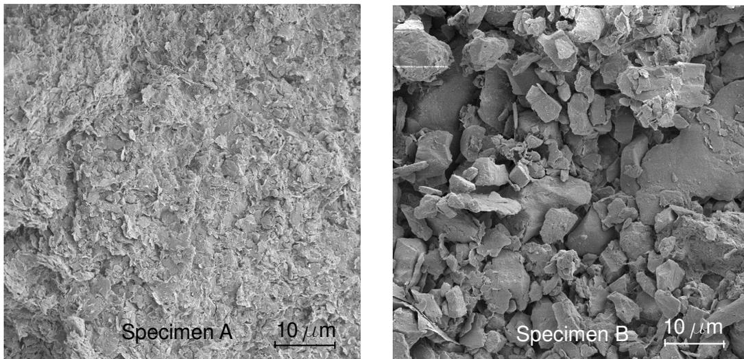
Figure 3. 23. SEM photographs of Sample A, the plastic brown clay layer forming the shear zone of the South Slide, and Sample B, the silty clay layer at South Slide.
