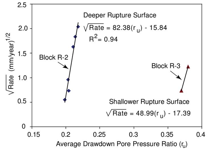
Figure 6.3. Correlation between pore pressure ratio during drawdown period and movement rate for reactivation blocks.
