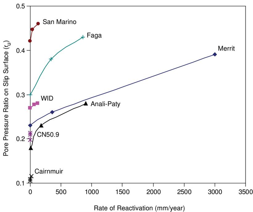
Figure 5.2. Movement acceleration with pore pressure ratio ( $r_u$ ) increasing on the slides' rupture surfaces.
