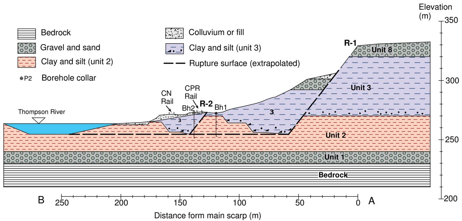
Figure 3.22. Cross section through the Basque Slide.
