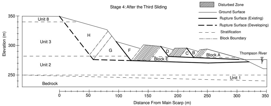
Figure A2.15 Goddard Slide after the third retrogression on the deeper rupture surface.
