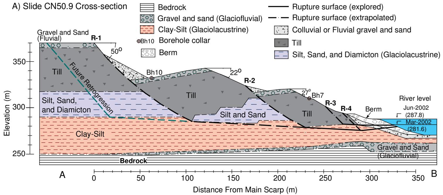
Figure 4.5A. Slide CN50.9 cross section showing the rupture surfaces, stratification, and borehole (see Figure 1 for cross-section line)
