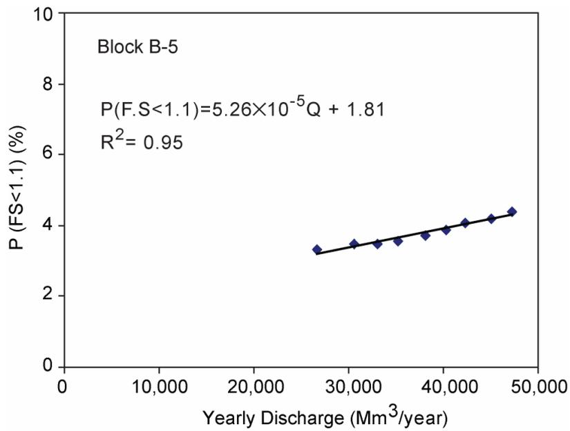
Figure 6.17. Change in the probability of Factor of Safety being less than 1.1 for the retrogressive block (block B-5) with river discharge
