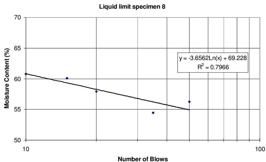
Figure A3.18 Liquid limit curve for specimen 8.
