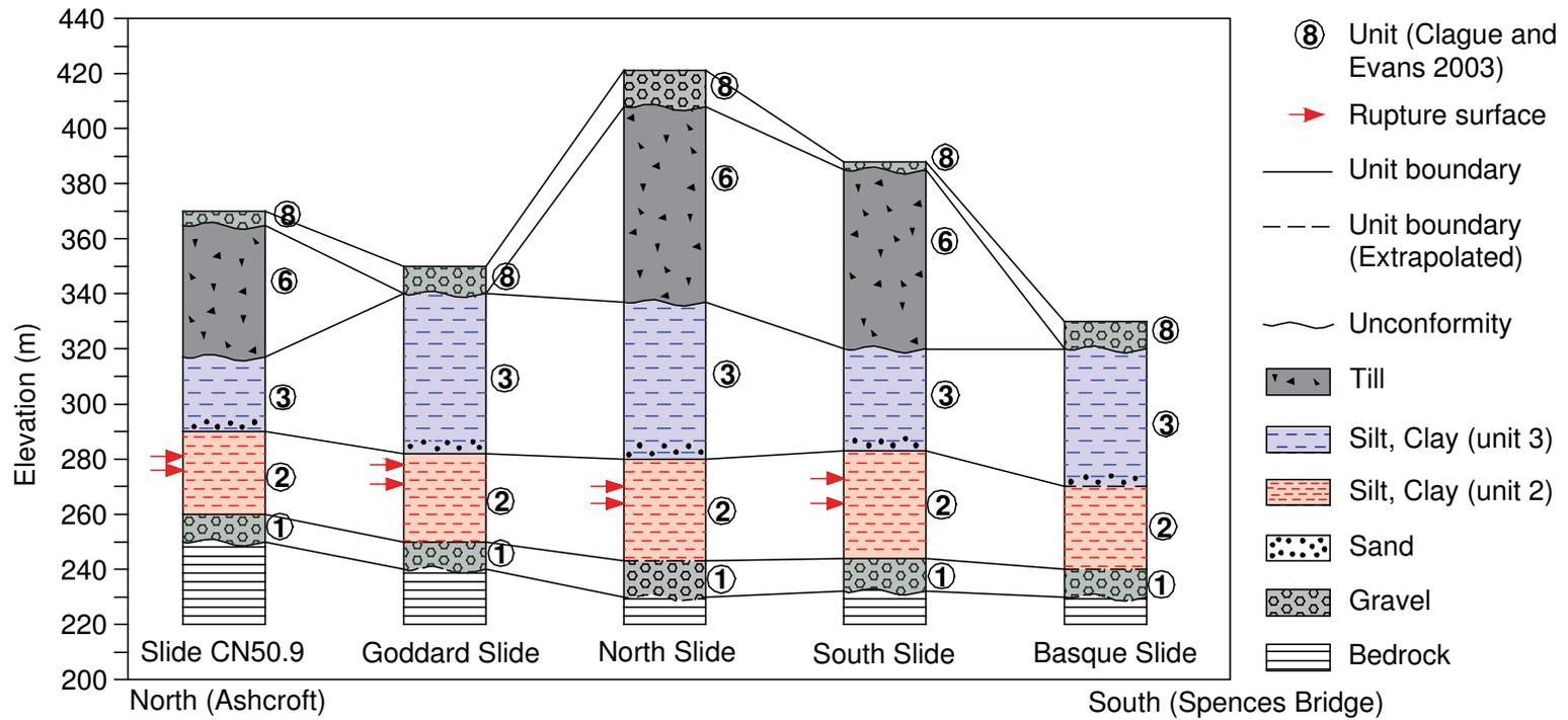
Figure 3.3. Geological units in the earth slides and highland terraces in Ashcroft area (the horizontal distance is not to scale)
