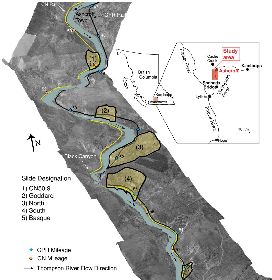
Figure 3.1. Landslides south of Ashcroft, BC, between 50° 10' to 50° 20' N and 121° 15' to 121° 20' W.
