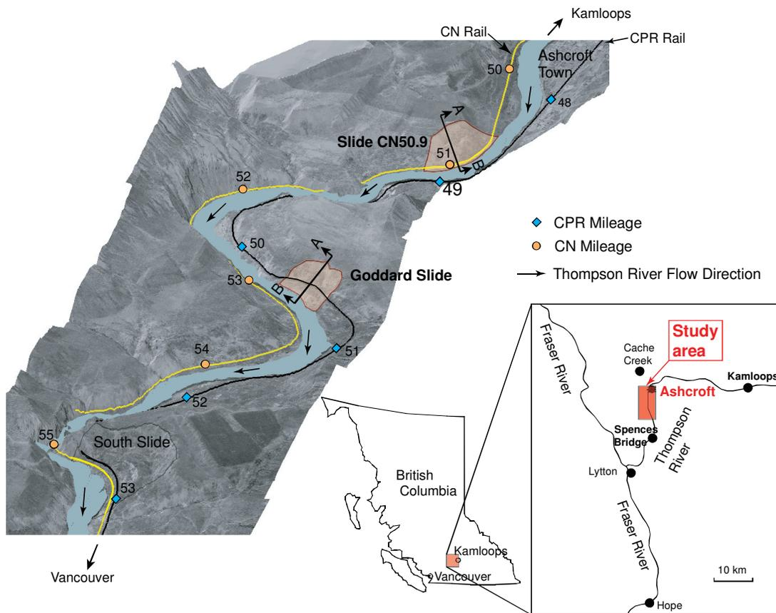
Figure 4.1. Study area south of Ashcroft, BC, between 50° 10' to 50° 20' N and 121° 15' to 121° 20' W in a view from south showing the location of the Goddard Slide and Slide CN50.9.
