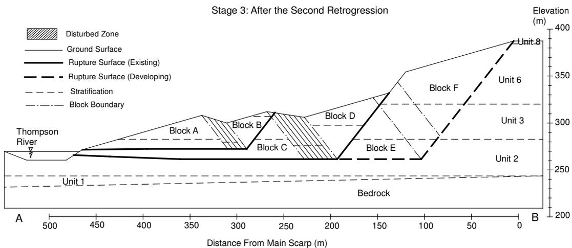
Figure A2.30 South Slide after the second retrogression on the deeper rupture surface.
