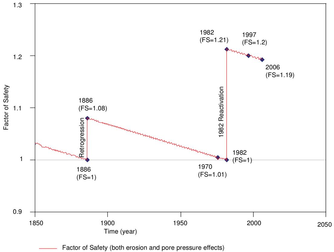
Figure 4.20. Change of factor of safety of the Goddard Slide within last 150 years.
