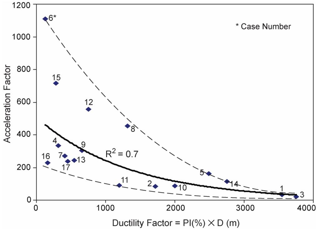
Figure 5.9. Acceleration Factor (A.F.) versus Ductility Factor.
