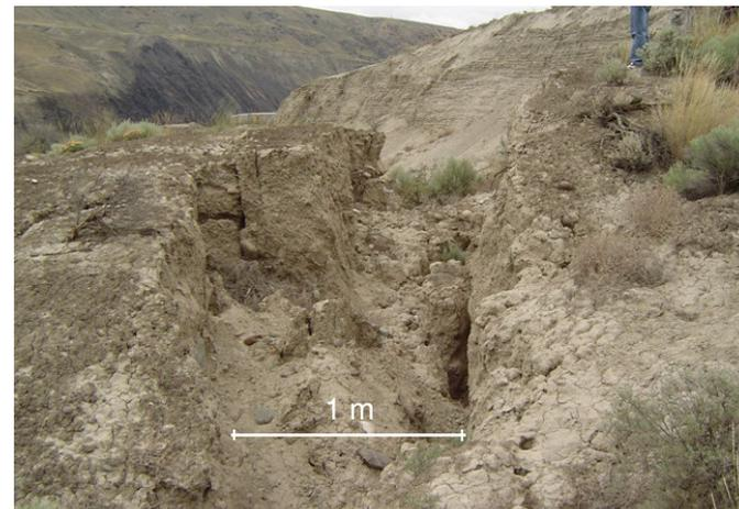
Figure 4. 21. Cracks at the Goddard Slide toe (A) resulted from toe erosion by the Thompson River at the active erosion site (see Figure 4.15 for location), and (B) resulted from the toe block (block R-4) translational movement (see Figure 4.15 for tension crack location).
