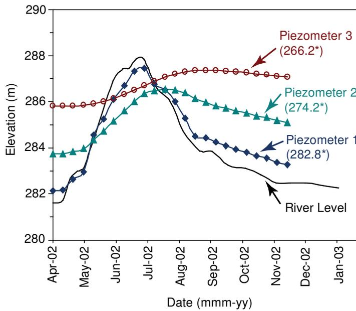
\*. Piezometer tip elevation (m)
