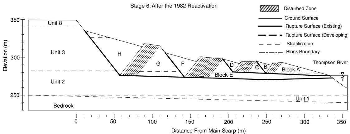
Figure A2.17 Goddard Slide after the 1982 reactivation.
