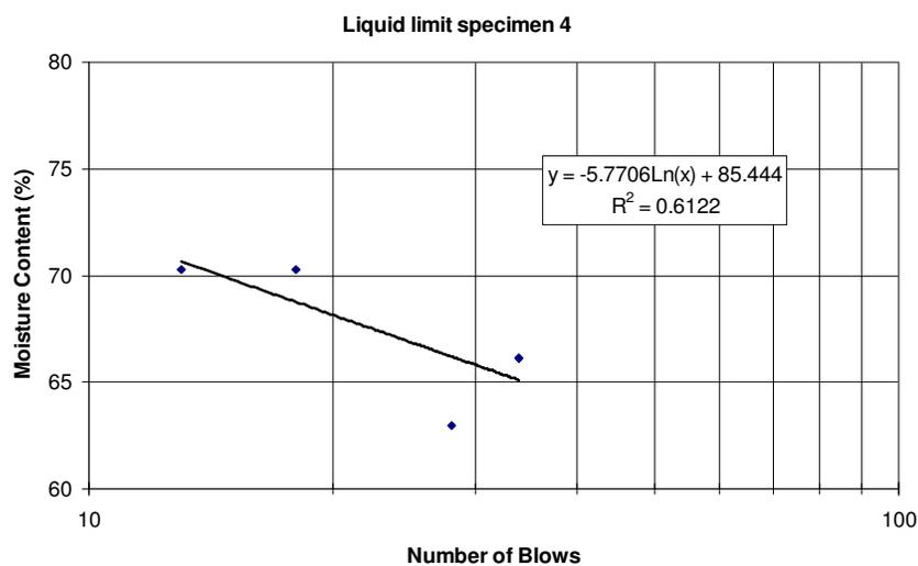
Figure A3.14 Liquid limit curve for specimen 4.
