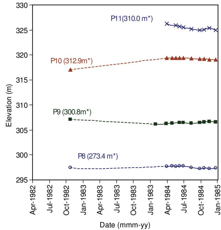
Figure 4.17. Data from piezometers installed in the Goddard Slide post-reactivation: (A) main body and foot and (B) crown.
