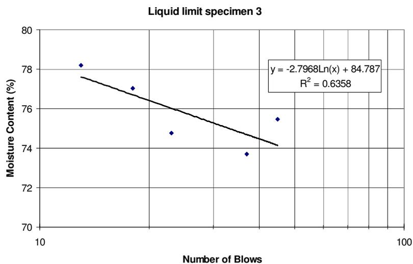
Figure A3.13 Liquid limit curve for specimen 3.
