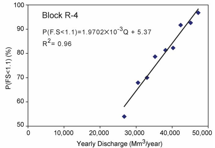
Figure 6.15. Change in the reactivation blocks' probability of Factor of Safety being less than 1.1 with the Thompson River yearly discharge
