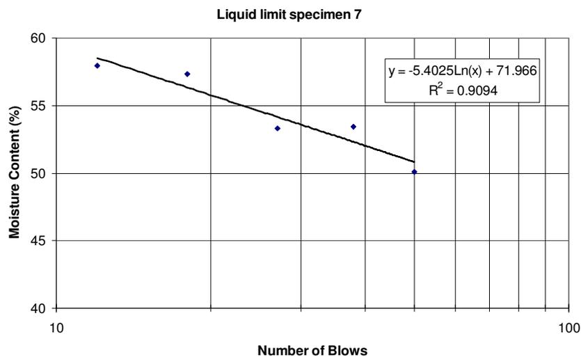
Figure A3.17 Liquid limit curve for specimen 7.
