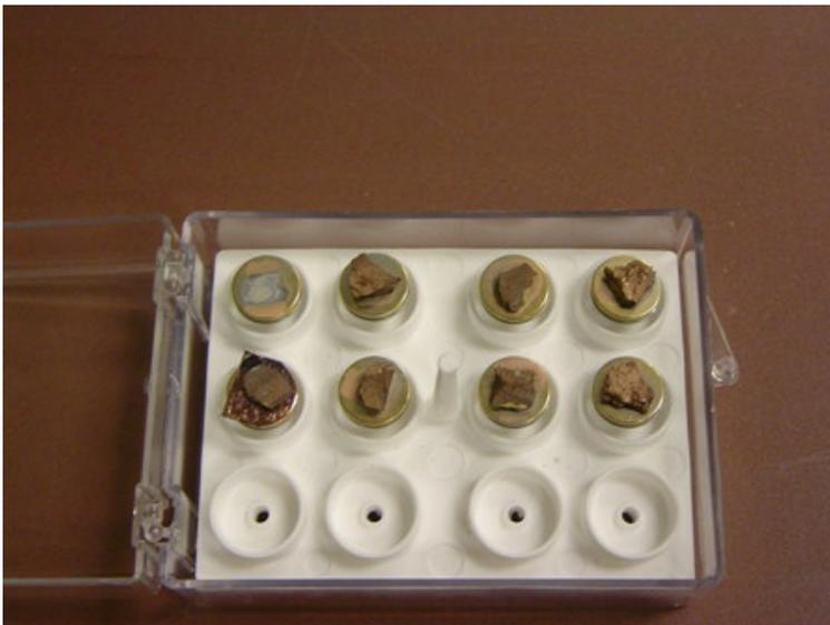
Figure A3.29 Gold coated specimens ready for Scanning Electronic Microscope.
