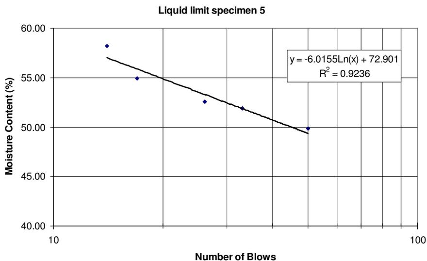
Figure A3.15 Liquid limit curve for specimen 5.
