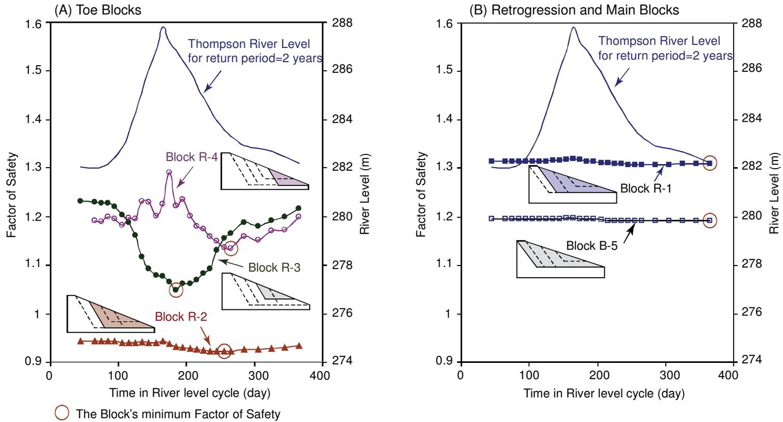
Figure 6.12. Deterministic stability analysis results with the Thompson River level fluctuation from the Thompson River 2-year return period discharge for (A) reactivation toe blocks, and (B) retrogression and main blocks
