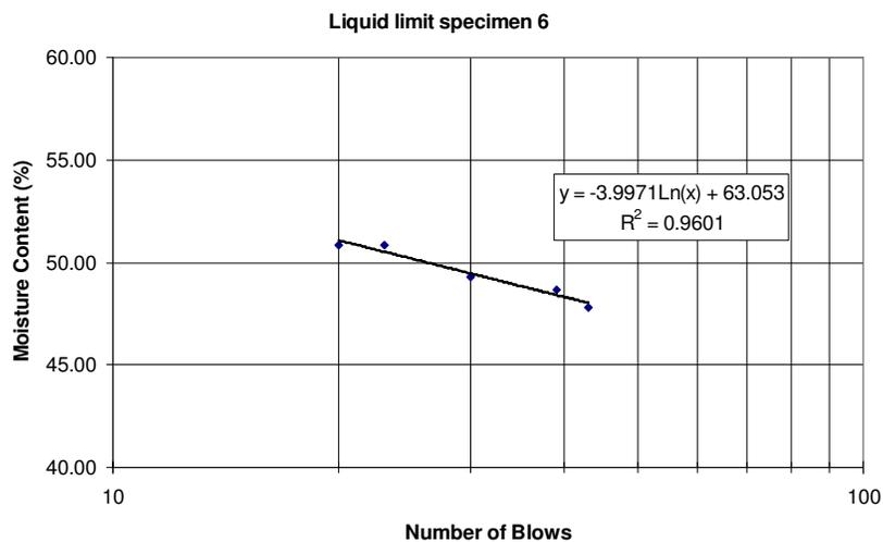
Figure A3.16 Liquid limit curve for specimen 6.
