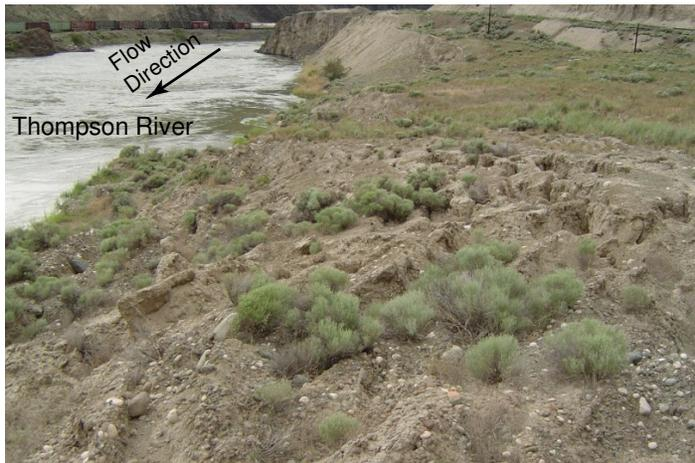
(B) Tension cracks from translational movement
