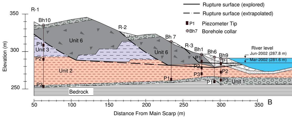
Figure 3.12. Piezometer locations at Slide CN50.9.
