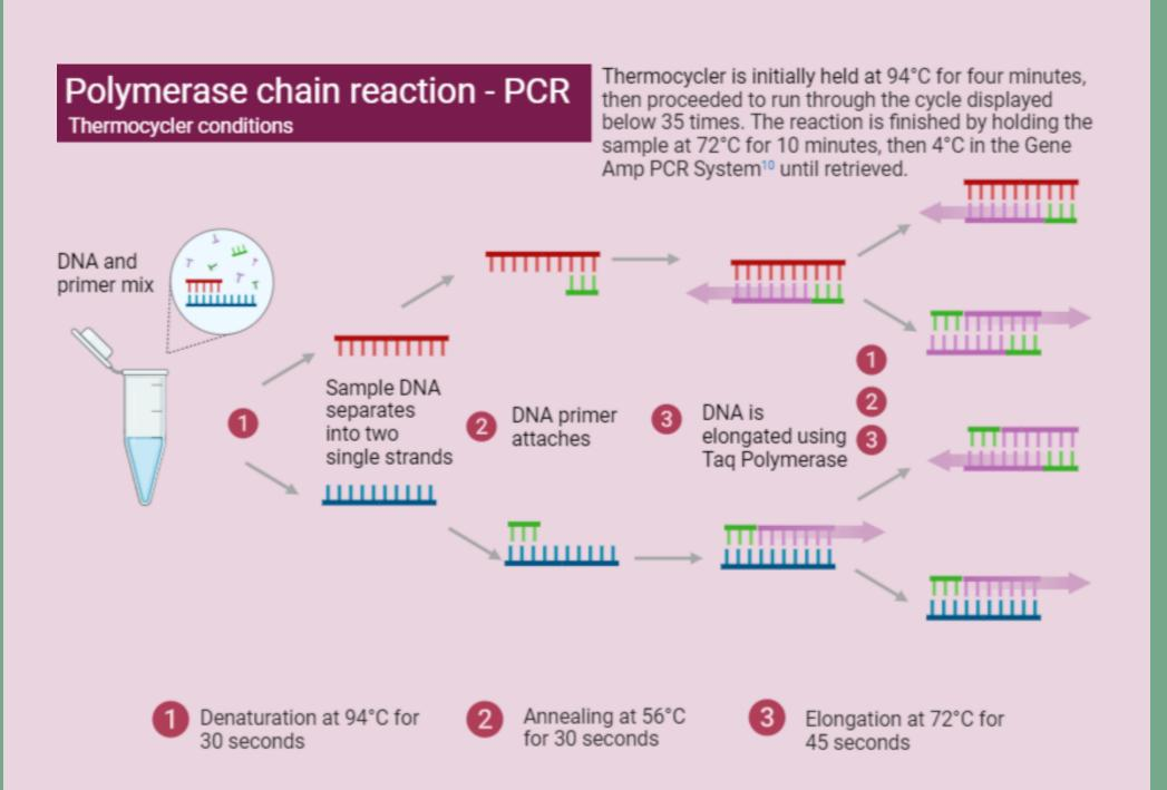
Figure 1.6: PCR test procedure and thermocycler conditions
