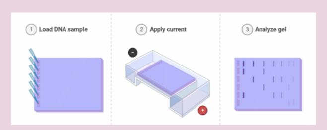
Figure 1.7: Agarose Gel Electrophoresis procedural diagram.
