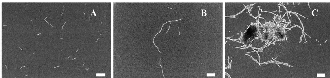
**Figure 2.13:** SEM images of **2.2a** in DMSO (0.01 mg/mL) at 0 h (A), 1 h (B) and 2 d (C).
