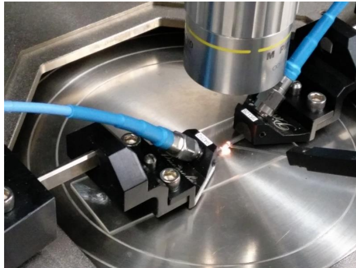
Fig. 4-15. Measurement with probe station .
