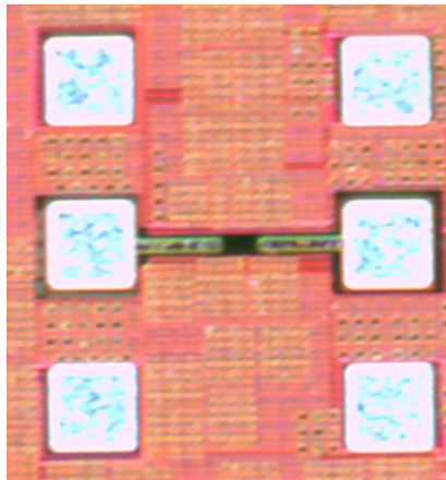
Fig. 3-21 Fabricated open structure for de-embedding.
