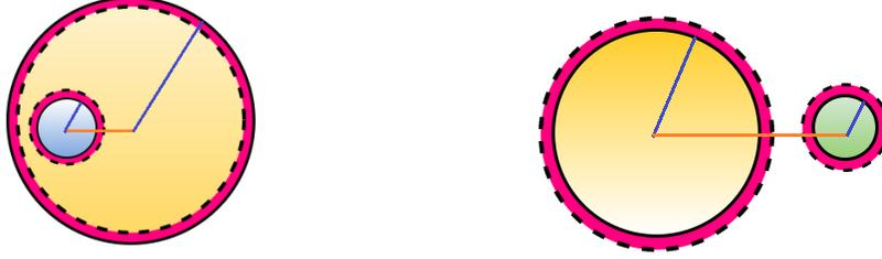
Figure 5.2: Implication constraints (left) guarantee that the region assigned to an implying variable is inside the region assigned to the implied variable. Mutual exclusion constraints (right) guarantee that regions assigned to the two variables are mutually exclusive.
