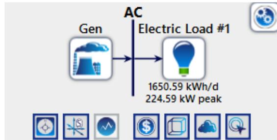
**Figure 28. Schematic of standalone microgrid with diesel generator (Scenario 1 – Community microgrid).**
