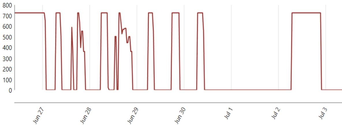
**Figure 24. Sample Generator power output (kW) for microgrid with diesel generator, solar PV, BESS, and FESS (Scenario 3 – Business microgrid).**
