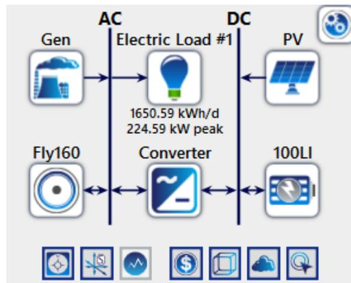
**Figure 26. Schematic of standalone microgrid with diesel generator, solar PV, BESS and FESS (Scenario 3 - Community microgrid).**
