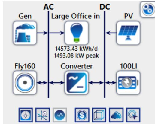
**Figure 22. Schematic of standalone microgrid with diesel generator, solar PV, BESS and FESS (Scenario 3 - Business microgrid).**
