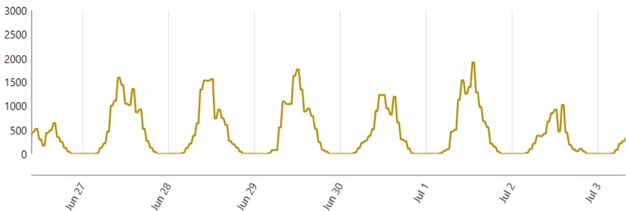
**Figure 19. Sample PV array power output (kW) for microgrid with diesel generator, solar PV, and BESS (Scenario 2 – Business microgrid).**
