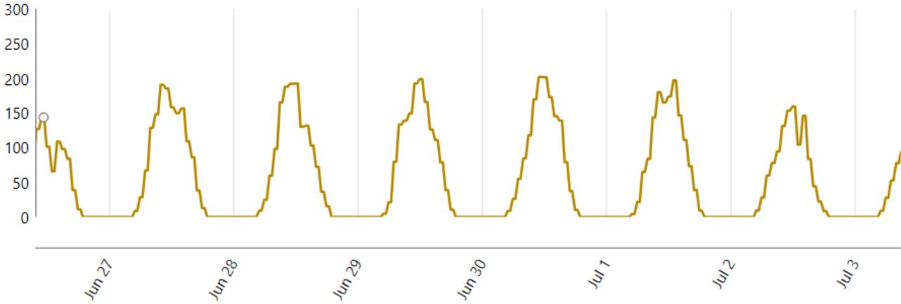
**Figure 36. Sample PV array power output (kW) for microgrid with diesel generator, solar PV, BESS, and FESS (Scenario 3 – Community microgrid).**
