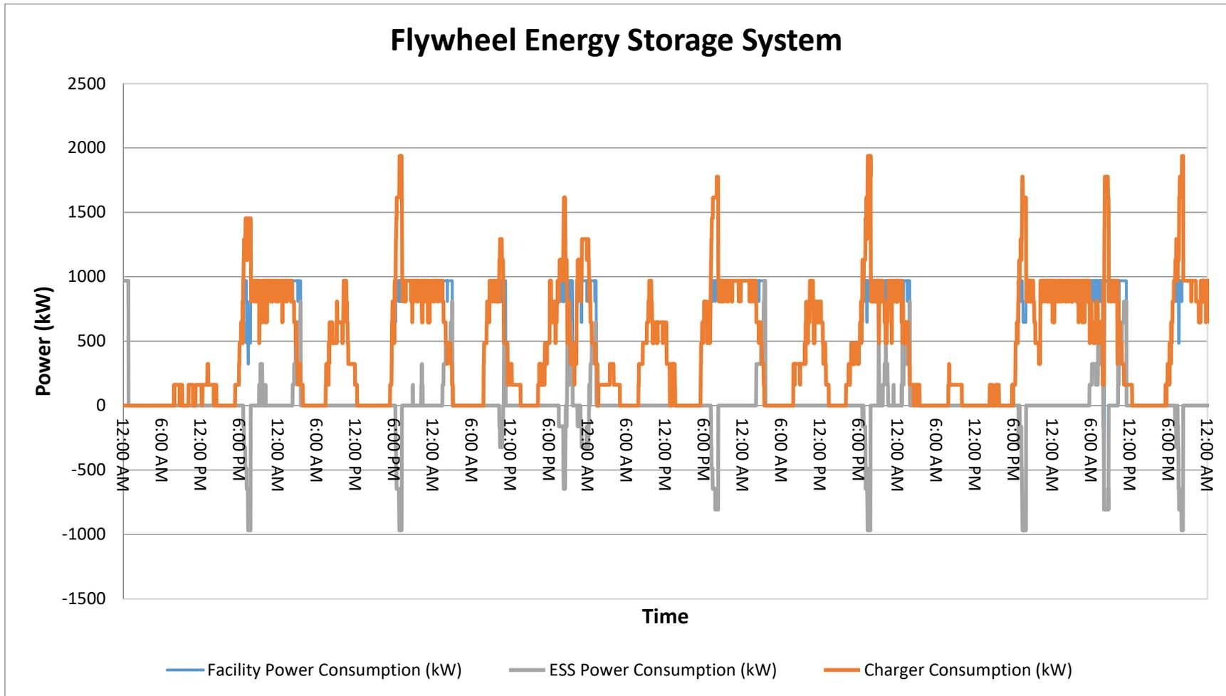
*Figure 9. FESS power performance (simulation results).*
