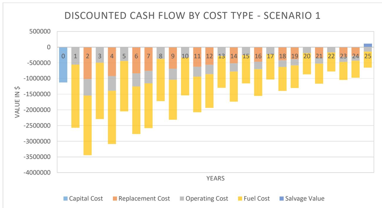
**Figure 16. Discounted cash flow by type of cost incurred for microgrid with diesel generator (Scenario 1 - Business microgrid).**
