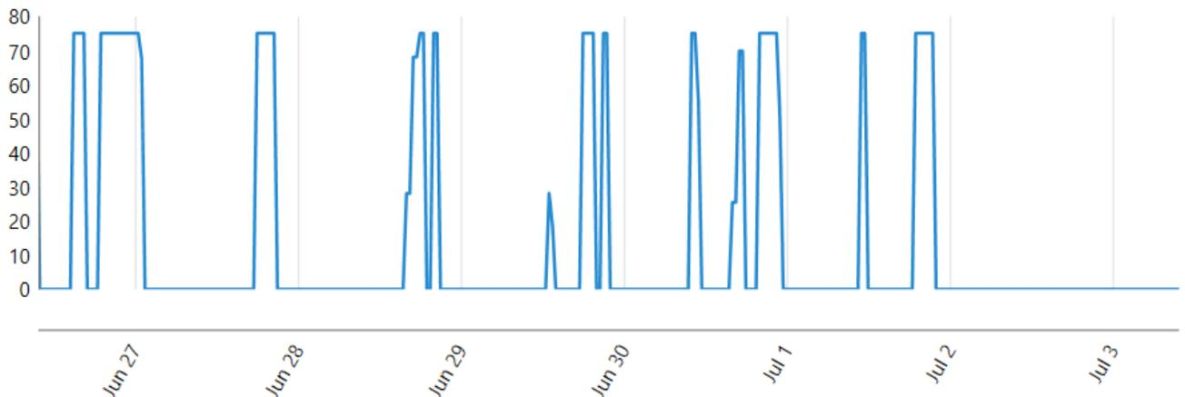
**Figure 33. Sample generator power output (kW) for microgrid with diesel generator, solar PV, and BESS (Scenario 2 – Community microgrid).**
