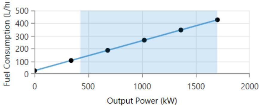
**Figure 14. Fuel consumption curve of generator.**
