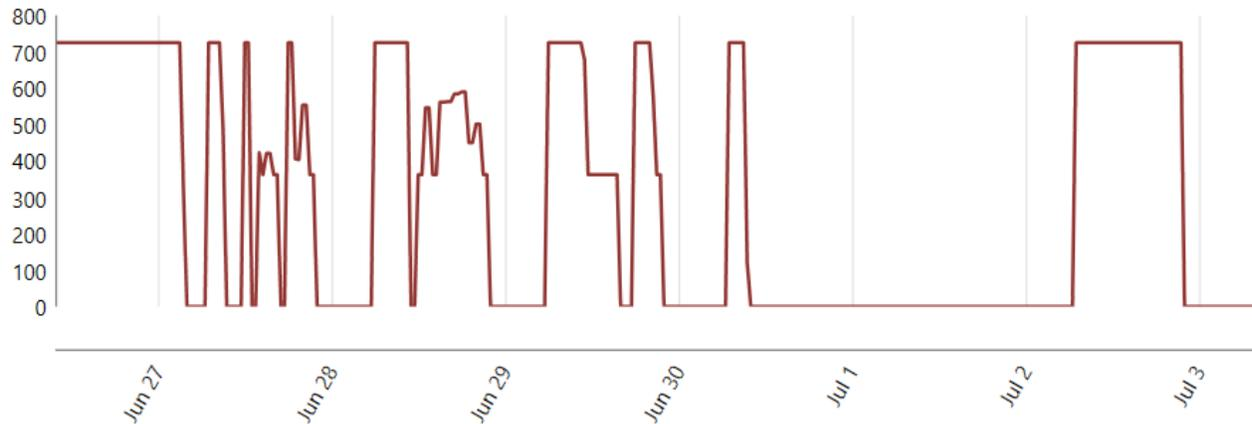
**Figure 20. Sample Generator power output (kW) for microgrid with diesel generator, solar PV, and BESS (Scenario 2 – Business microgrid).**
