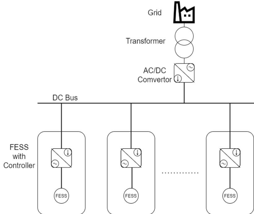
**Figure 7. DC microgrid with FESS based on [68].**
