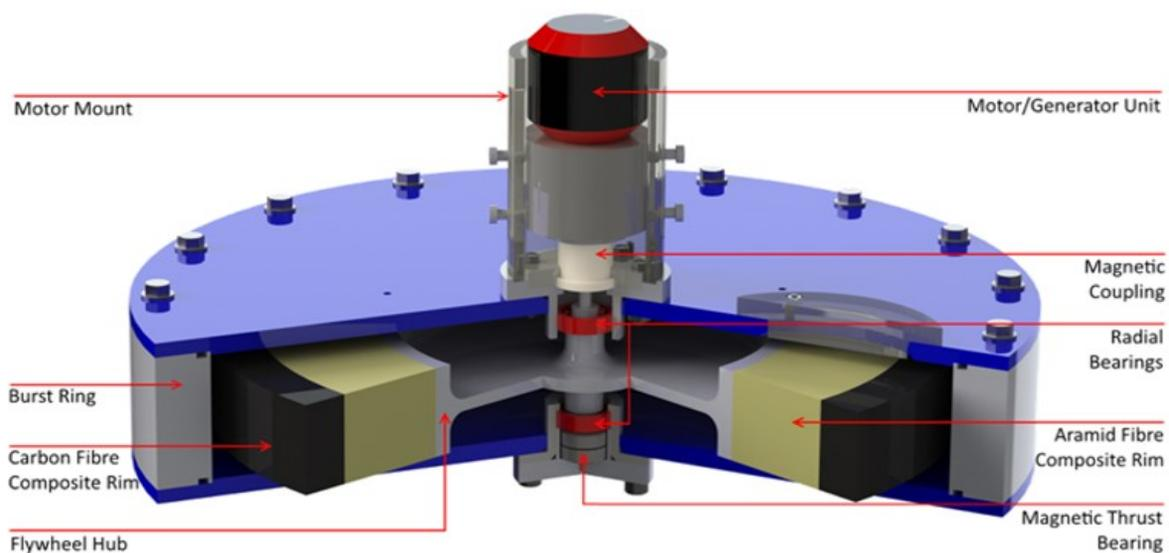
*Figure 4. Example of Flywheel Energy Storage System.*
