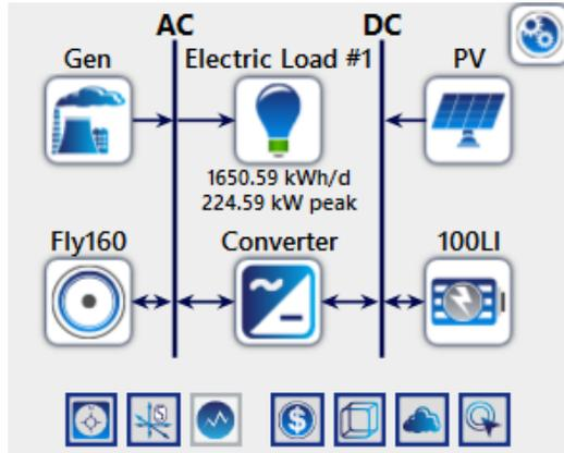
**Figure 35. Schematic of standalone microgrid with diesel generator, solar PV, BESS and FESS (Scenario 3 - Community microgrid).**
