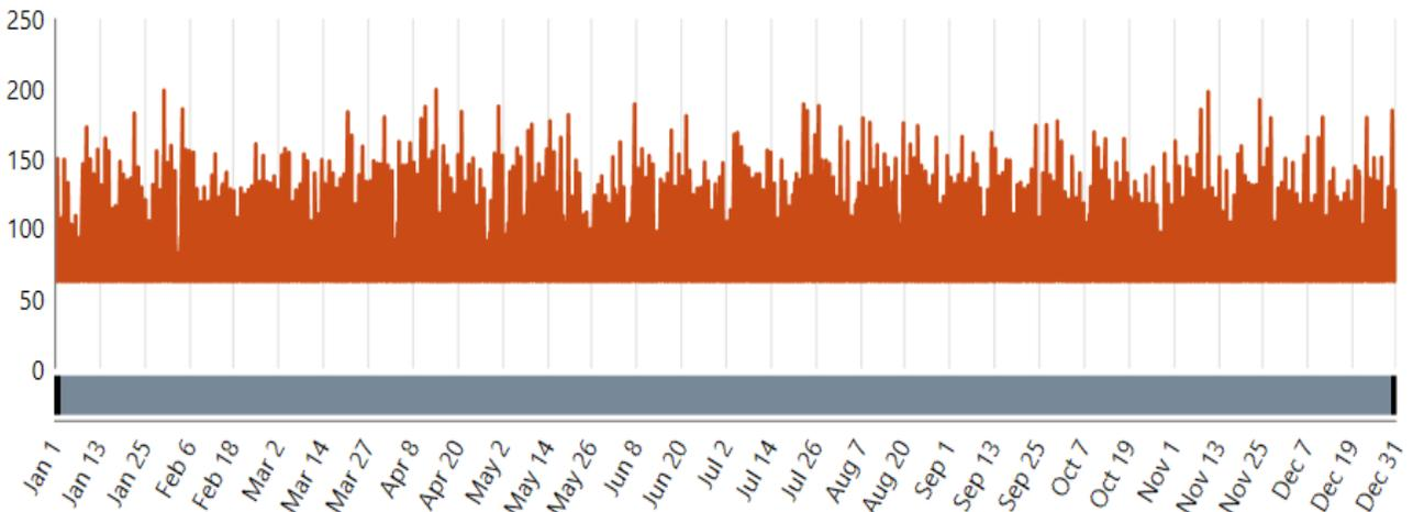
**Figure 29. Generator power output (kW) for microgrid with diesel generator (Scenario 1 – Community microgrid).**
