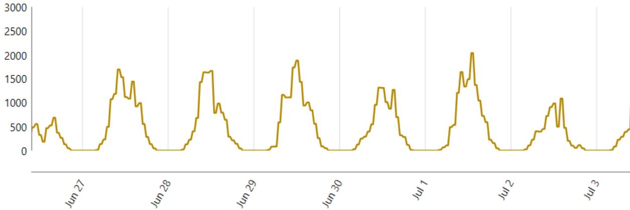
**Figure 23. Sample PV array power output (kW) for microgrid with diesel generator, solar PV, BESS, and FESS (Scenario 3 – Business microgrid).**
