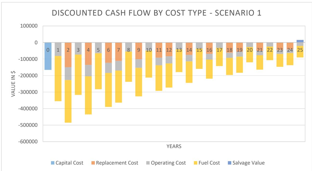
**Figure 30. Discounted cash flow by type of cost incurred for microgrid with diesel generator (Scenario 1 - Community microgrid).**
