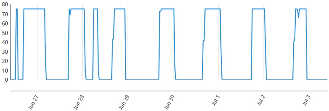
**Figure 37. Sample generator power output (kW) for microgrid with diesel generator, solar PV, BESS, and FESS (Scenario 3 – Community microgrid).**
