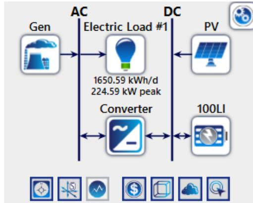
**Figure 31. Schematic of standalone microgrid with diesel generator, solar PV, and BESS (Scenario 2 - Community microgrid).**
