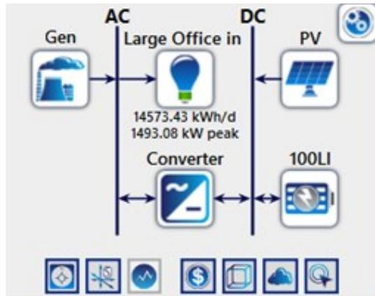
**Figure 18. Schematic of standalone microgrid with diesel generator, solar PV, and BESS (Scenario 2 - Business microgrid).**
