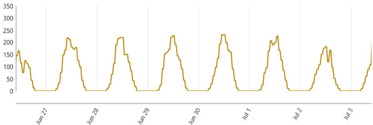
**Figure 32. Sample PV array power output (kW) for microgrid with diesel generator, solar PV, and BESS (Scenario 2 – Community microgrid).**
