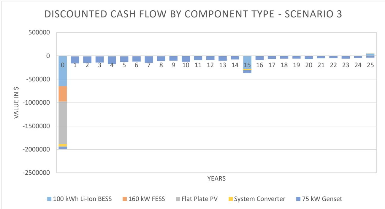
**Figure 38. Discounted cash flow by component type for microgrid with diesel generator, solar PV, BESS and FESS (Scenario 3 - Community microgrid).**
