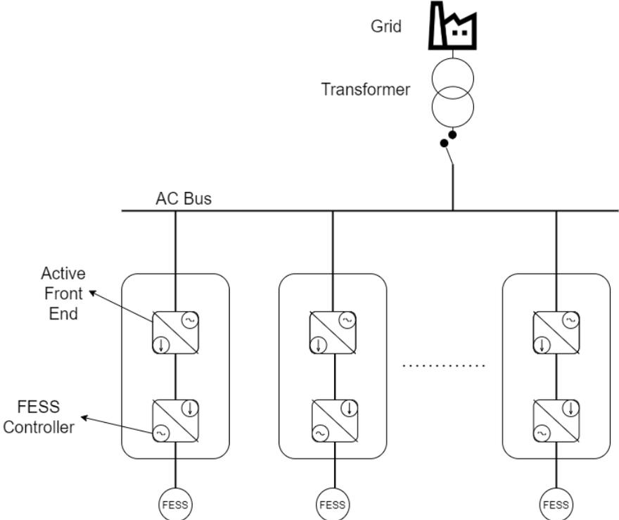
**Figure 6. AC microgrid with FESS based on [68].**
