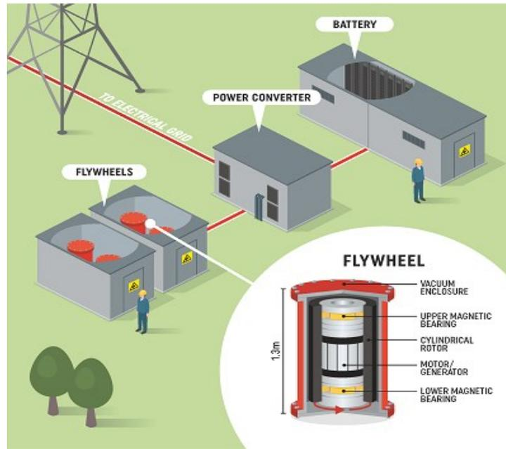
Figure 11. Hybrid energy storage system at University of Sheffield [103].
