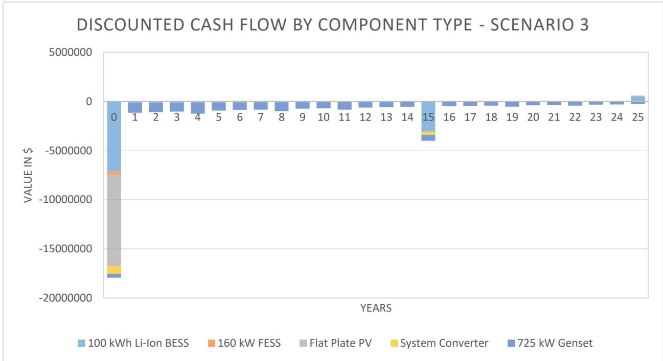
**Figure 25. Discounted cash flow by component type for microgrid with diesel generator, solar PV, BESS, and FESS (Scenario 3 - Business microgrid).**
