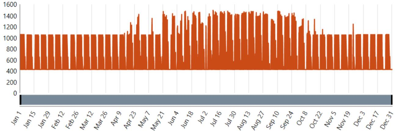
**Figure 17. Generator power output (kW) for microgrid with diesel generator (Scenario 1 – Business microgrid).**
