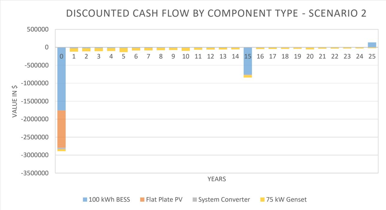
**Figure 34. Discounted cash flow by component type for microgrid with diesel generator, solar PV and BESS (Scenario 2 - Community microgrid).**
