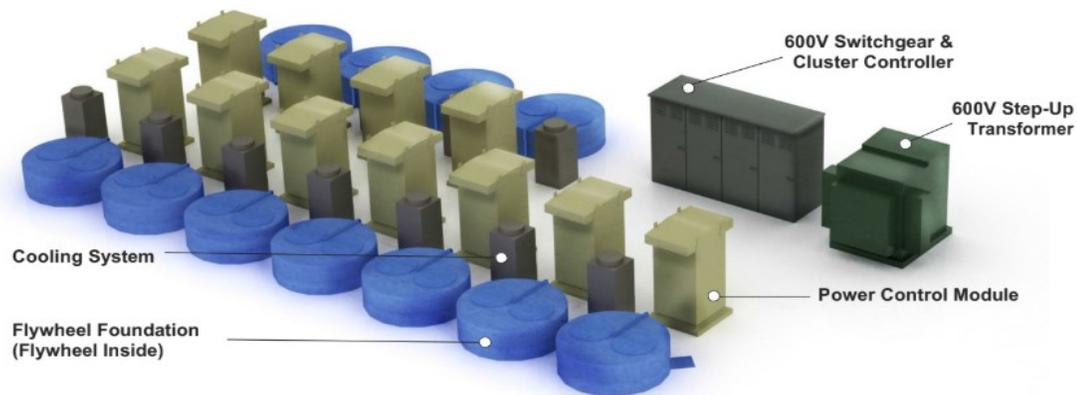
*Figure 5. Flywheel Energy Storage System modules [68].*
