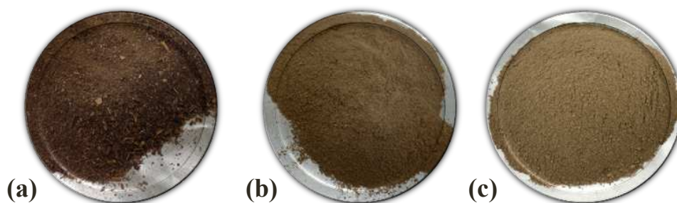
Figure 3.1: Air-dried, crushed, and sieved (a) PEAT-1, (b) PF-1 and (c) PF-2 reclamation materials received from an oil and gas industry located in Alberta.
