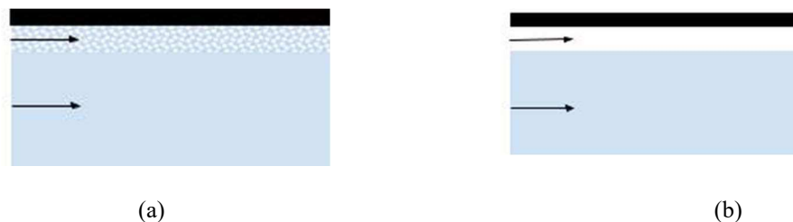
Figure 2.12. Distribution of the air injected beneath a flat plate, (a) bubble drag reduction (BDR) and (b) air layer drag reduction (ALDR)
