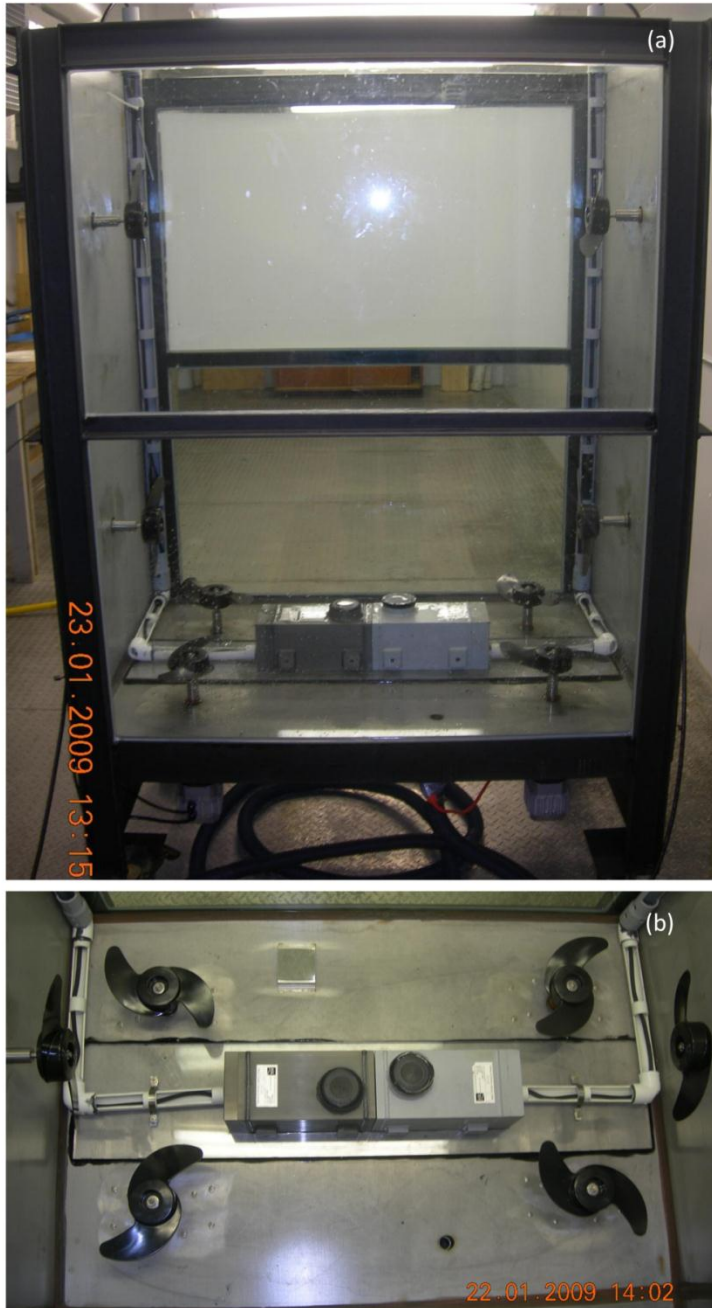
Fig. 2.2. (a) Front view of the frazil ice tank. (b) top view of the frazil ice tank setup showing the high and low frequency sonar units, the Plexiglas base plate, and cables inside the hollow PVC tubes; two of the side mounted propellers and the four bottom mounted propellers are also shown.
