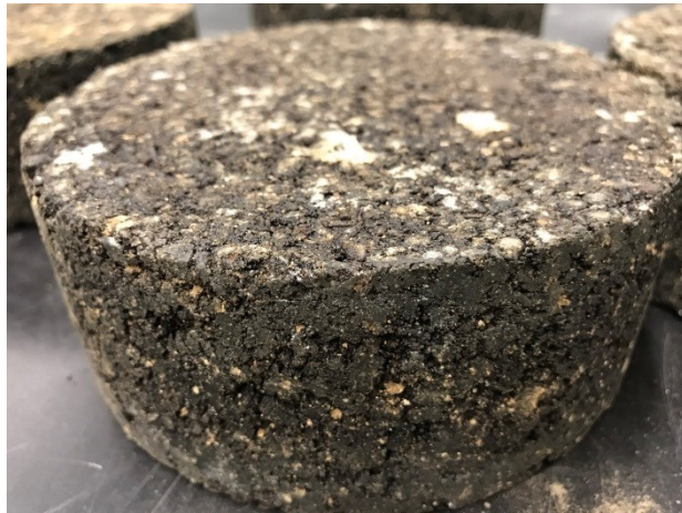
Figure: Details of water activated CMA before wheel tracker test
