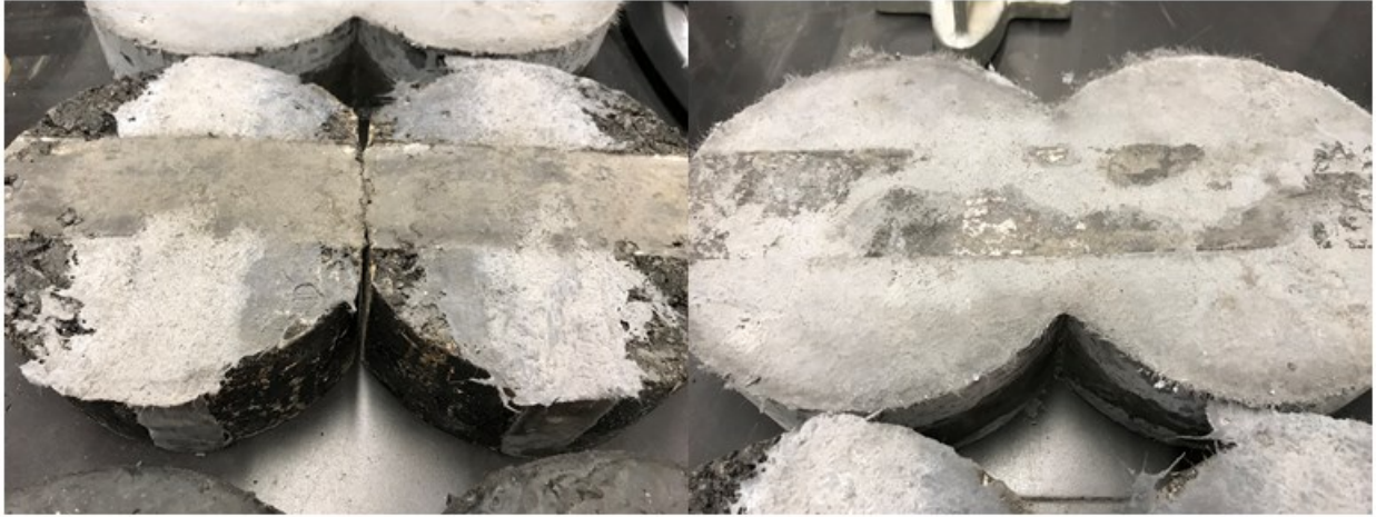
Figure: Details of ECC and ECC (trench) after wheel tracker test
