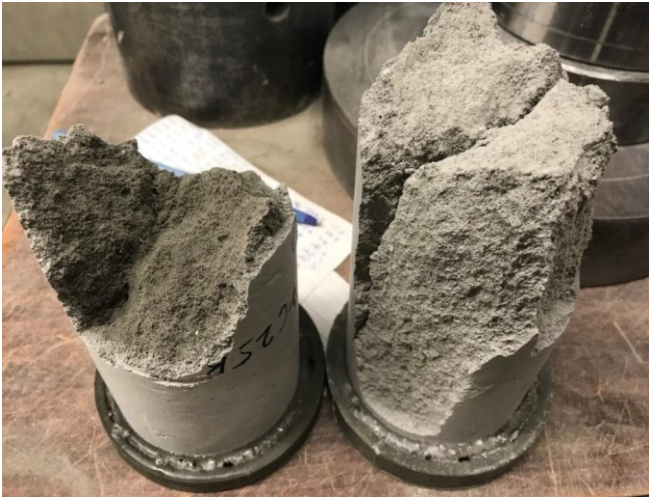
Figure 3-8: Water absorption samples before (right) and after conditioning (left)
