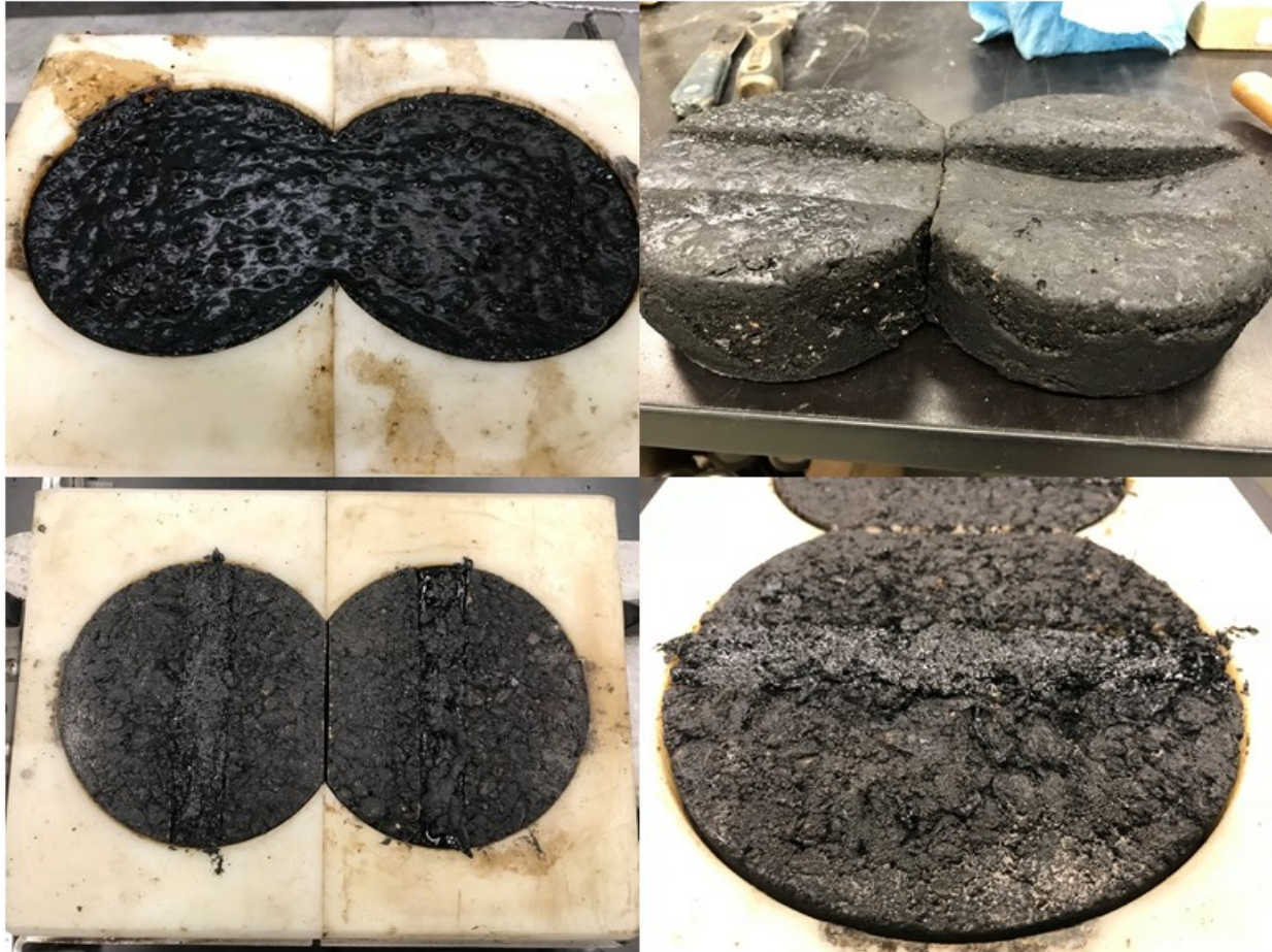
Figure: Details of PMA and PMA (trench) before and after wheel tracker test
