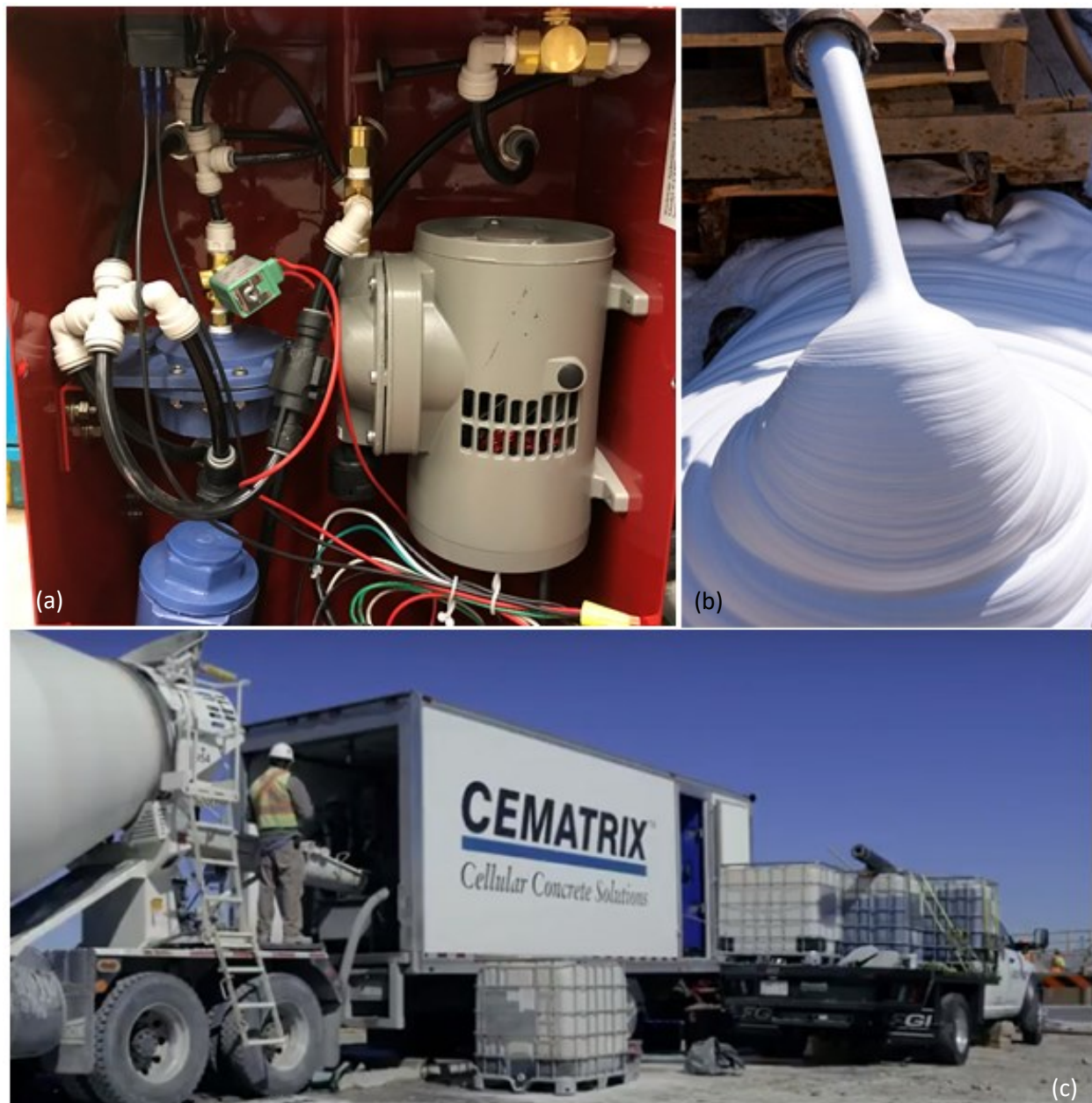
Figure 2-2: Cellular concrete production. (a) Foam dry method system. (b) Foam consistency (Thiessen Team, 2011). (c) In-situ application (Cematrix, 2018)
