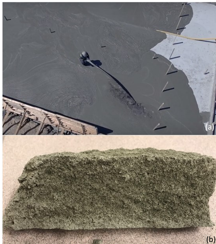
Figure 2-3: Details of foam grout (a) flowability (Cematrix, 2018), and (b) air void content
