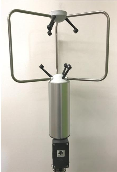
(a) 3D ultrasonic anemometer
