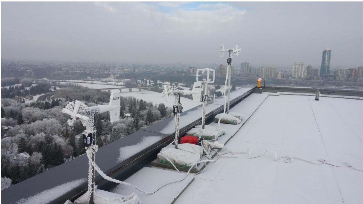
(e) Anemometers under icing conditions
