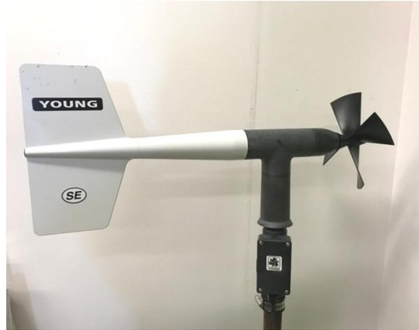
(b) Mechanical anemometer (wind monitor)
