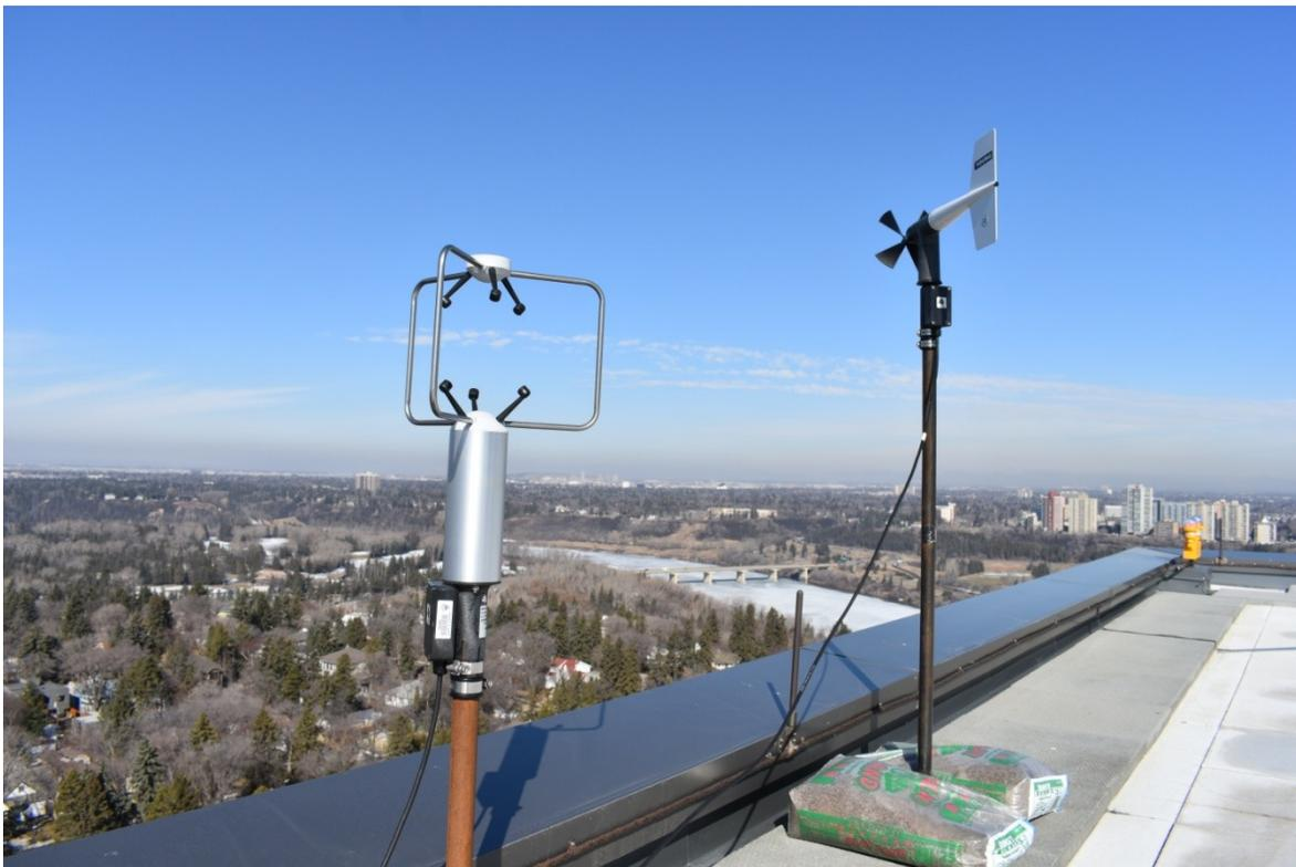
(c) Ultrasonic anemometer and Wind Monitor #3
