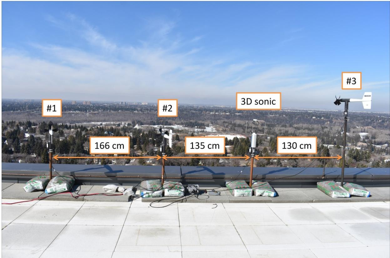
**Figure 19 Anemometers set up on DICE rooftop (2)**
