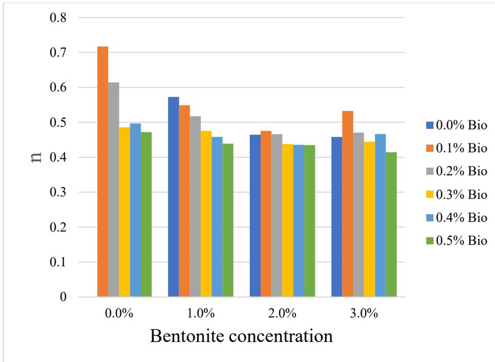
Figure A-2 Herschel-Bulkley flow behavior index (n) of drilling fluids
