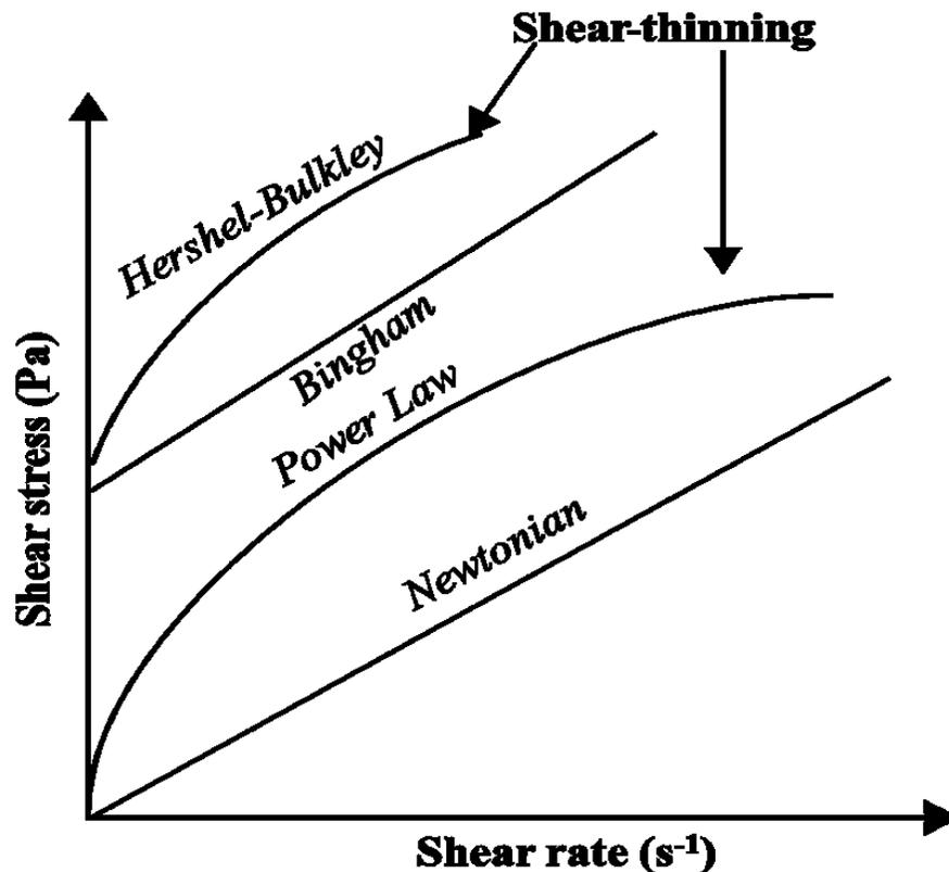
Figure 3.1. Shear stress versus shear rate relationships of various rheological models
