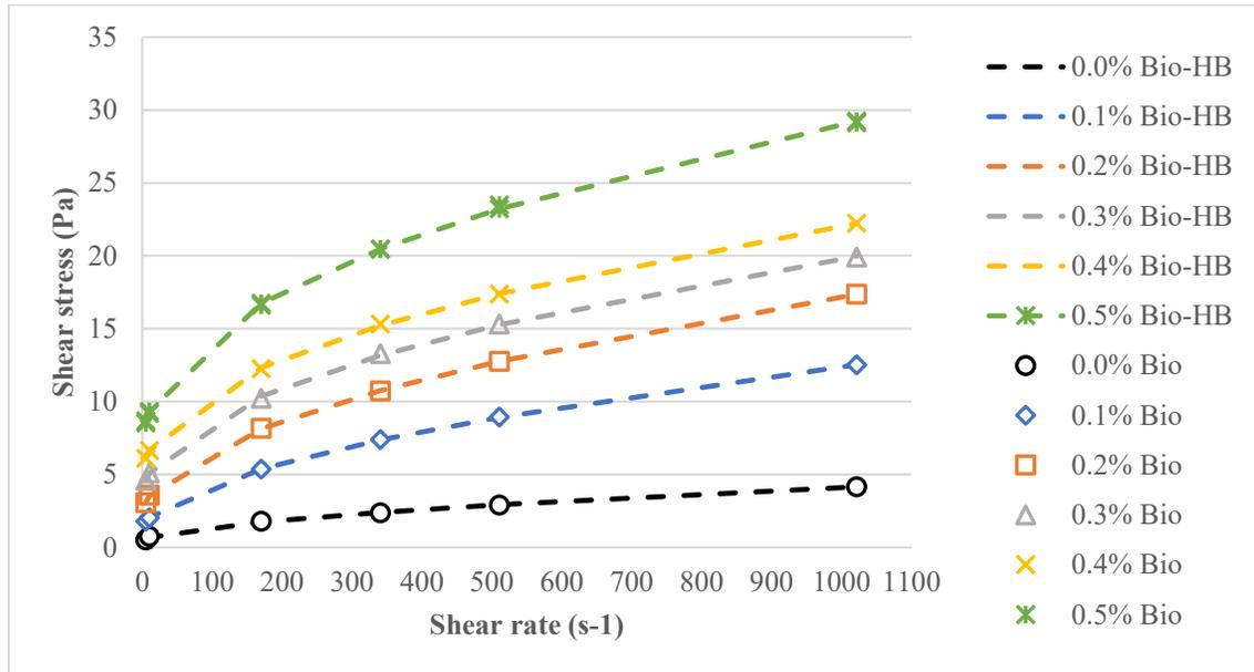
Figure 4.5 Rheograms of 1% bentonite with the biopolymer and estimated rheograms of HB model
