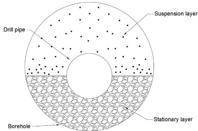
Figure 2.2. Two-layer model for cuttings transport in the annulus
