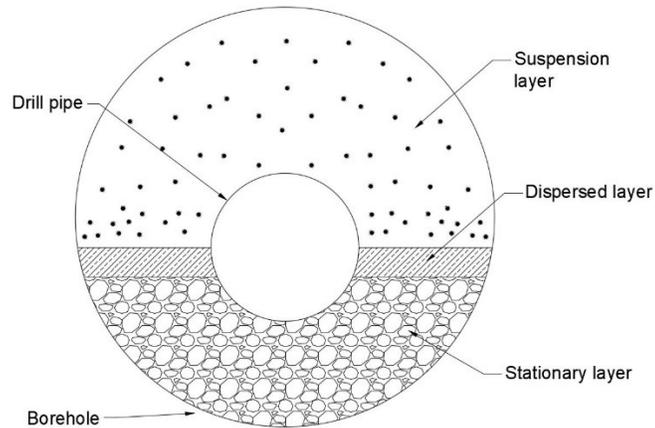
Figure 2.3. Three-layer model for cuttings transport in the annulus
