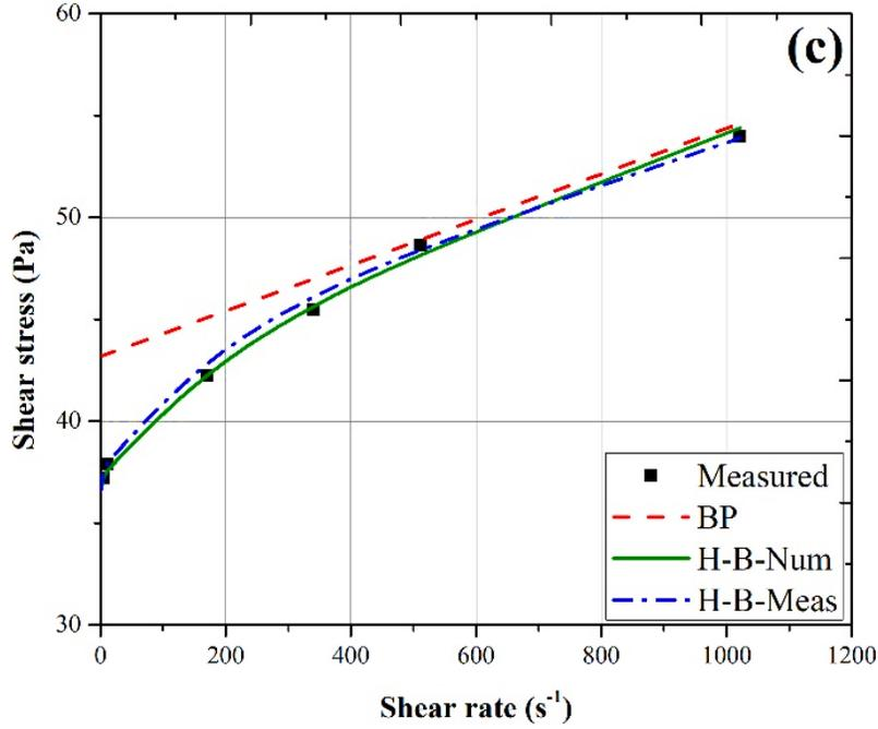
Figure 3.6. Comparison of the experimental shear stress vs shear rate data with the predictions from BP and H-B models (a) 1% bentonite drilling fluid (b) 3% bentonite drilling fluid (c) 5% bentonite drilling fluid
