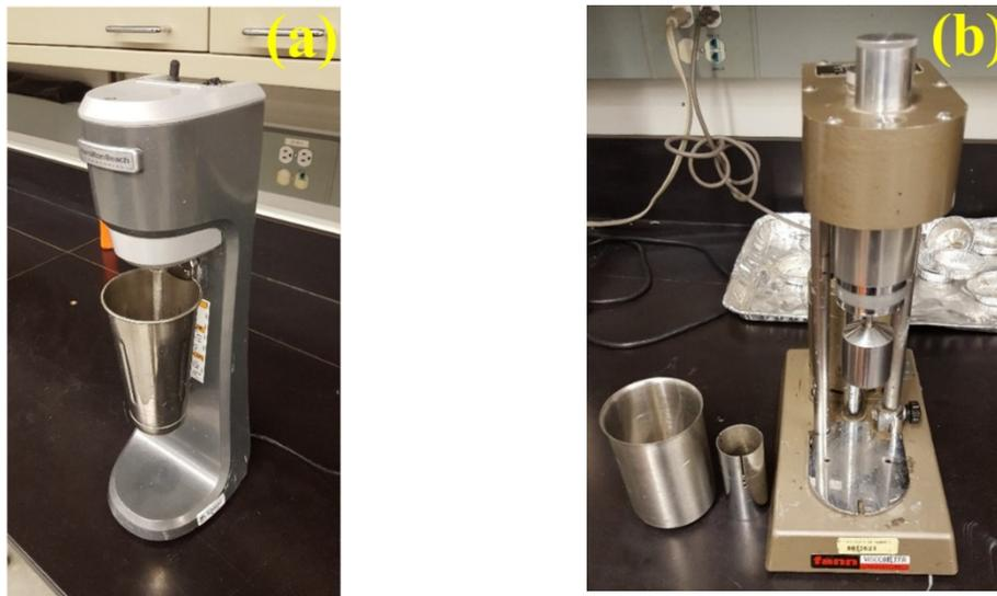
Figure 3.4. Testing apparatus (a) Hamilton Beach HMD200 Series Single Spindle mixer(b) Fann 35A viscometer
