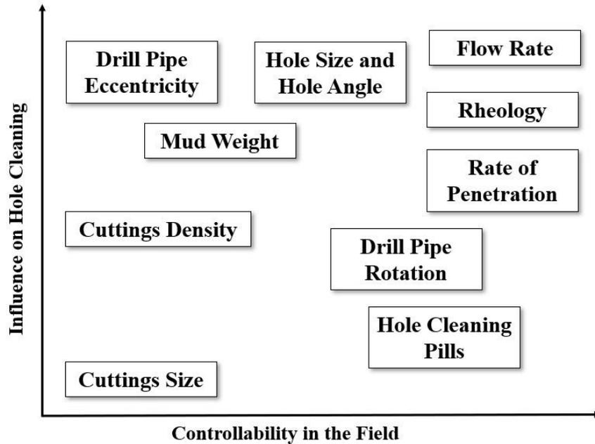
Figure 2.5 Key variables controlling cuttings transport (Adari et al. 2000)
