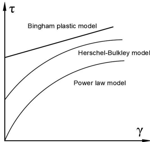
Figure 2.6 Shear stress-shear rate relationships of the three rheological models
