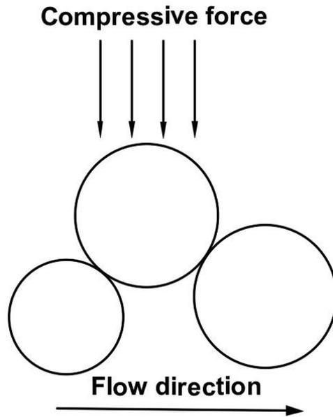
Figure 3.3 Compressive force caused by the normal stress difference in viscoelastic fluids
