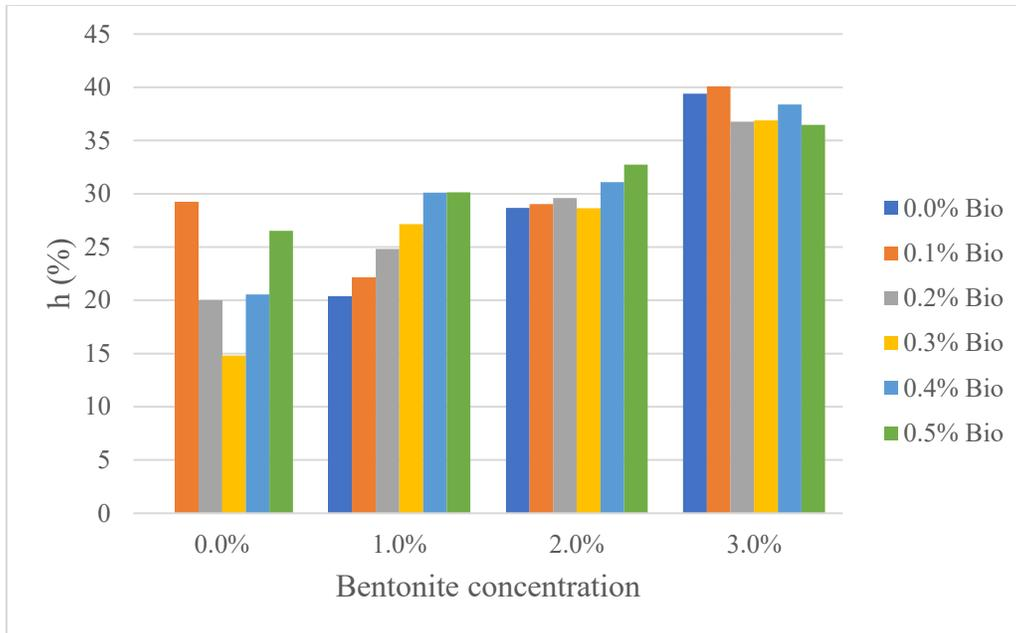
Figure 4.9 Plug width of drilling fluids
