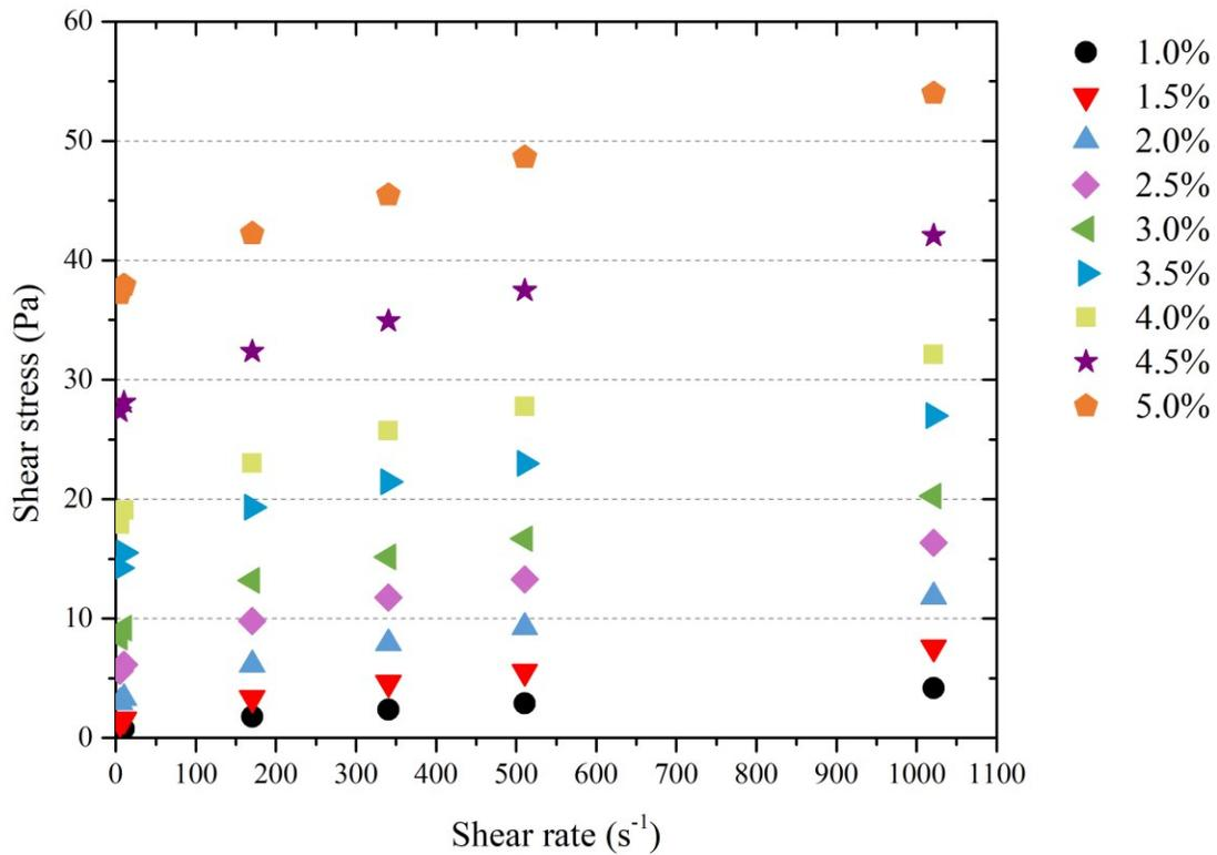
Figure 3.5. Rheograms of drilling fluids with different bentonite concentrations
