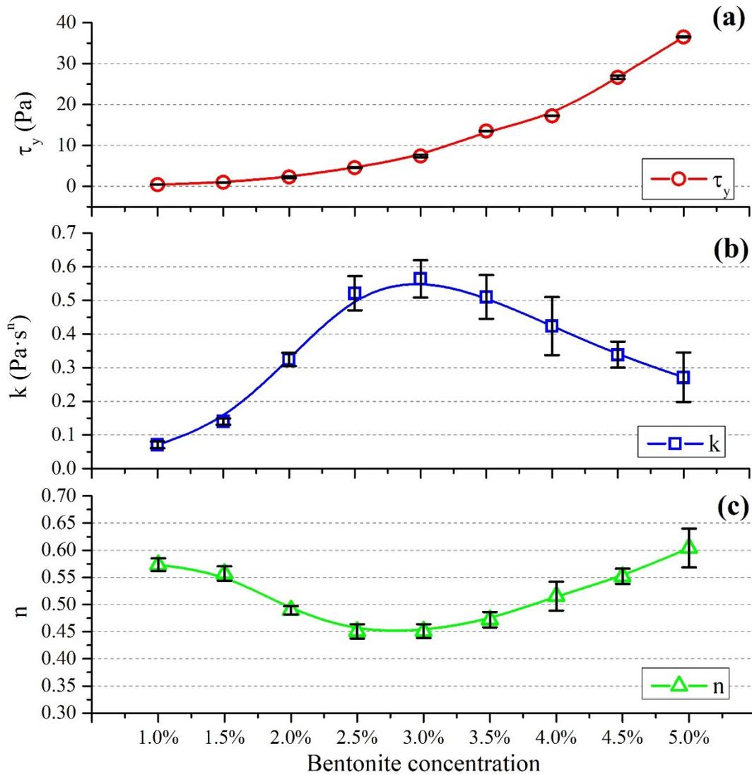
Figure 3.10 Herschel-Bulkley parameters (a) yield stress ( $\tau_y$ ) (b) consistency index ( $k$ ) (c) flow behavior index ( $n$ )
