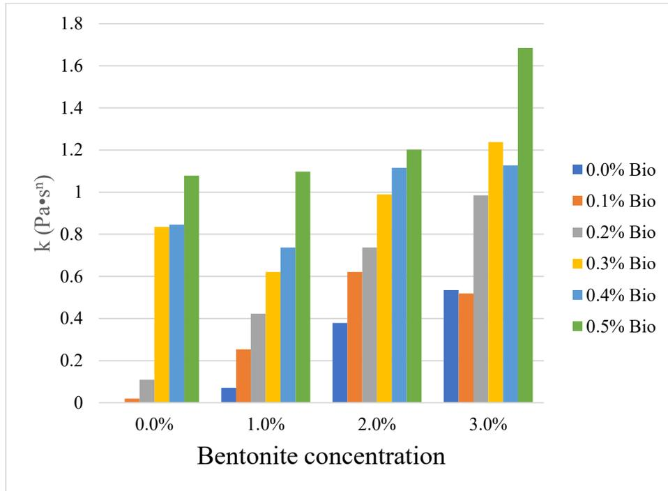
Figure A-1 Herschel-Bulkley consistency index (k) of drilling fluids
