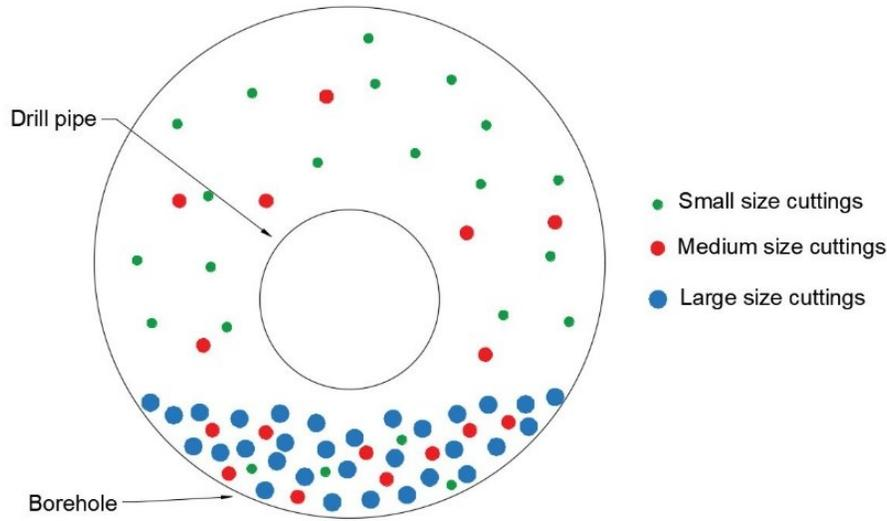
Figure 2.4. Annular cuttings transport model for large-diameter HDD borehole (Shu et al. 2015)
