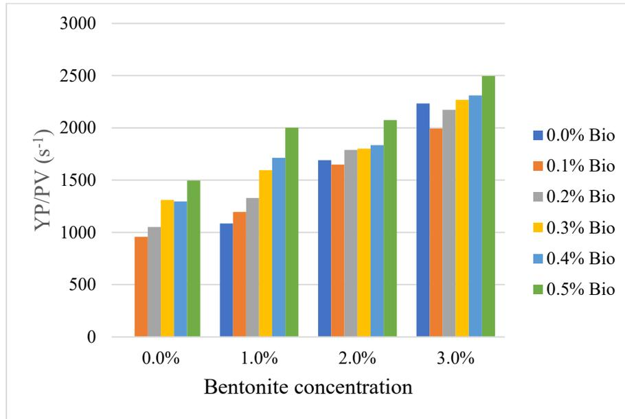
Figure 4.10  $YP/PV$  of drilling fluids
