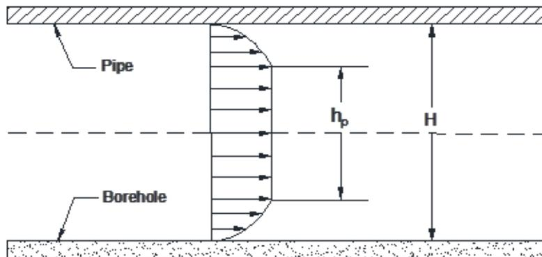
Figure 3.2. Velocity profile of drilling fluid in the annulus
