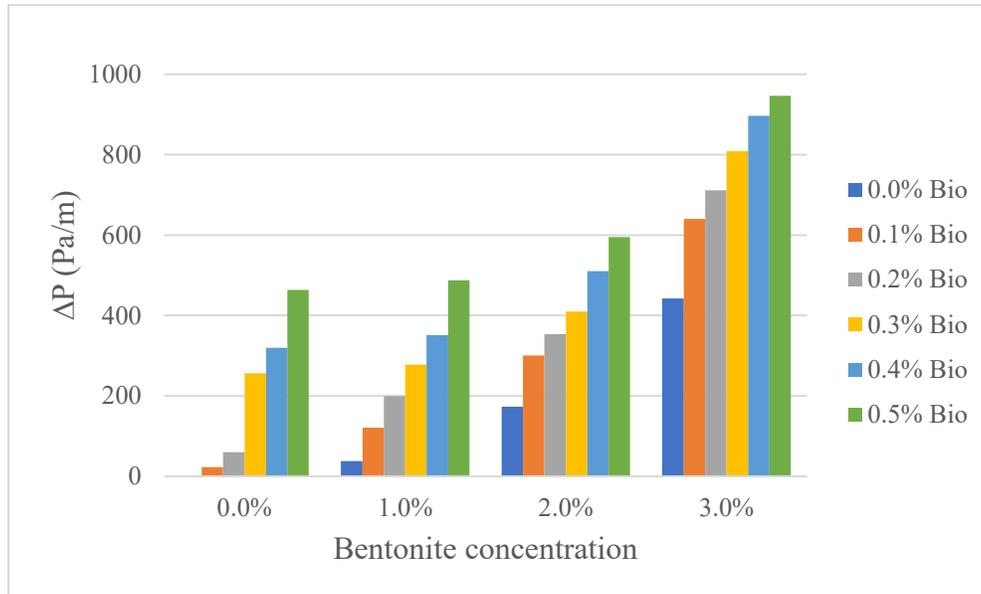
Figure 4.11 Frictional pressure loss of drilling fluids
