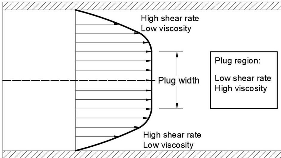
Figure 4.1 Flattened velocity profile in the annulus
