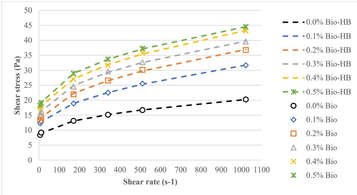
Figure 4.7 Rheograms of 3% bentonite with the biopolymer and estimated rheograms of HB model
