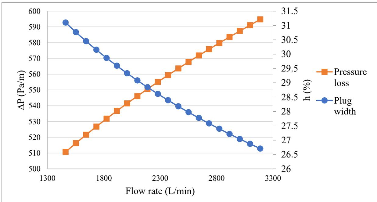
Figure 4.12 Effect of increasing flow rate when using sample #2-4
