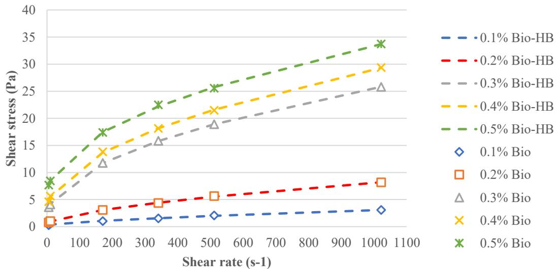
Figure 4.4 Rheograms of 0% bentonite with the biopolymer and estimated rheograms of HB model
