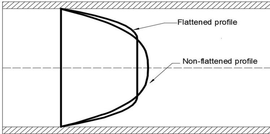
Figure 2.7 Flattened and non-flattened velocity profiles
