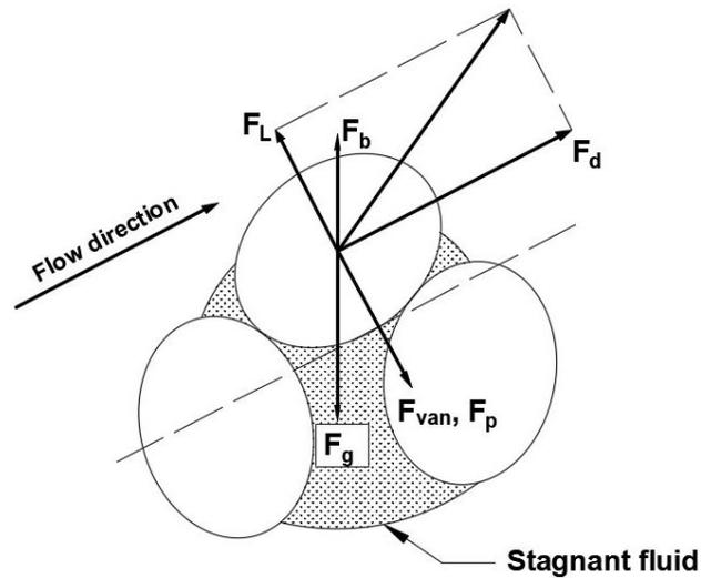
Figure 2.1 Schematics of forces acting on a single particle in the cuttings bed
