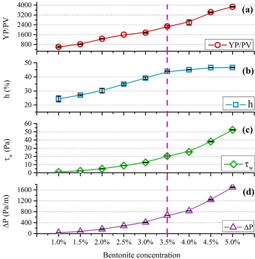
Figure 3.11 (a)  $YP/PV$  vs. Bentonite concentration (b) Normalized plug width ( $h$ ) vs. Bentonite concentration Normalized (c) Wall shear stress ( $\tau_w$ ) vs. Bentonite concentration (d) Frictional pressure loss ( $\Delta P$ ) vs. Bentonite concentration
