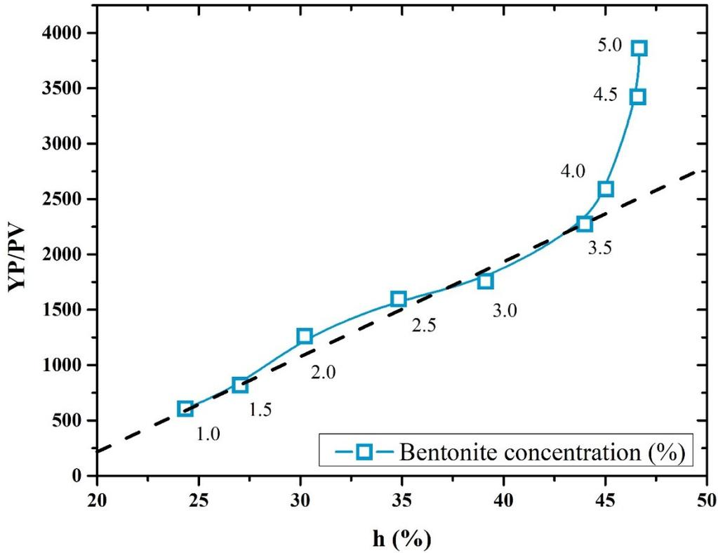
Figure 3.12 The correlation between parameters  $YP/PV$  and  $h$
