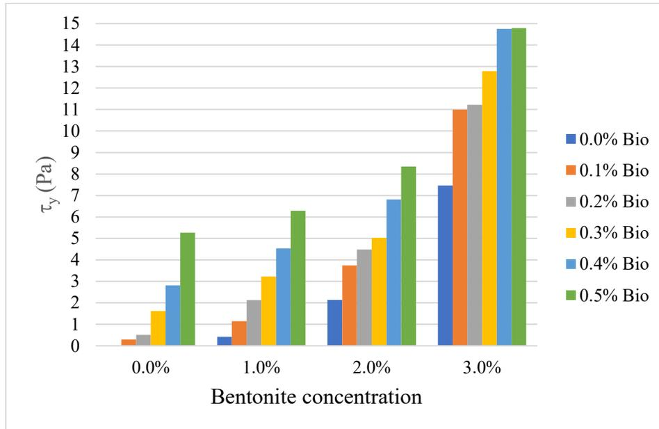
Figure 4.8 Herschel-Bulkley yield stress ( $\tau_y$ ) of drilling fluids
