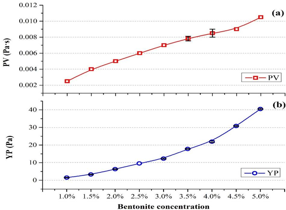
Figure 3.9 BP model parameters (a) Plastic Viscosity (b) Yield Point
