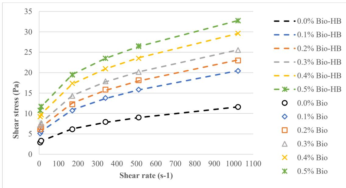
Figure 4.6 Rheograms of 2% bentonite with the biopolymer and estimated rheograms of HB model
