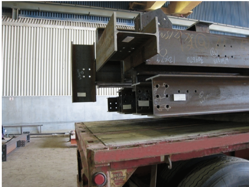
Figure 9. Tagged pieces ready to be shipped.
