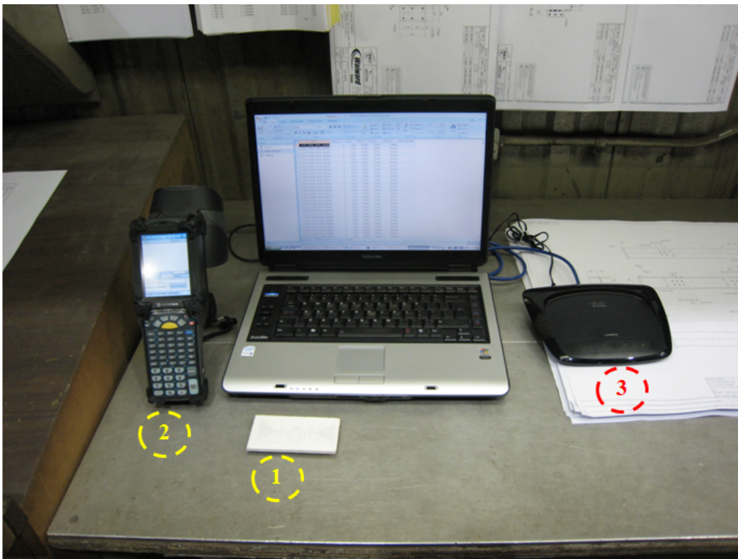
Figure B-1. Data acquisition system based on RFID technology.
