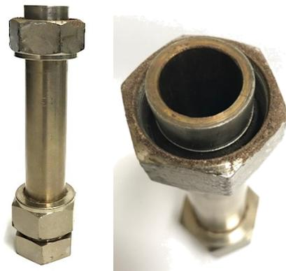
**Figure B. 3.** Photos of the Micro Batch Reactor
