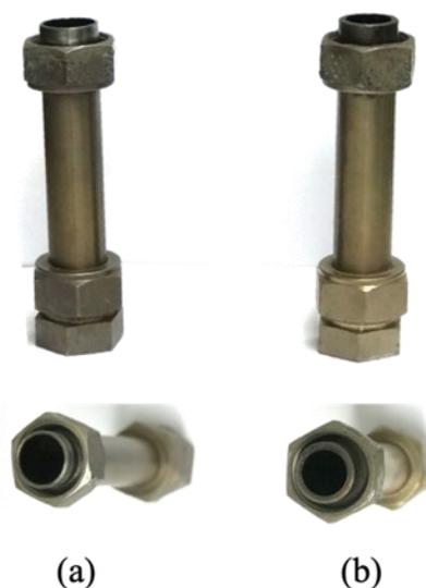
**Figure A. 1.** Photos of Micro Batch Reactors used in (a) Reactions B, B+S, B+W+S
