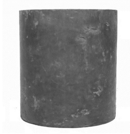
Figure 2.5: Intact Clearwater clay-shale sample to test.
