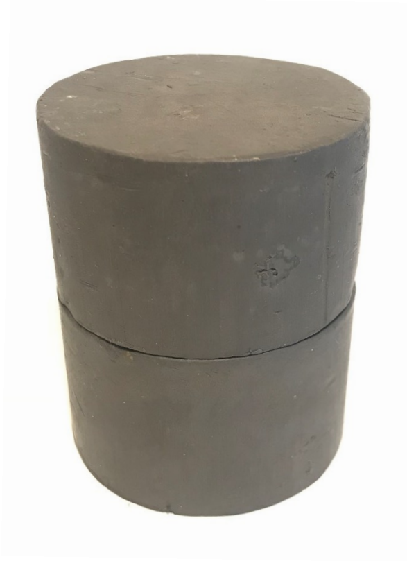
Figure 3.5: Reconstituted sample loaded to \sigma'_v = 1 MPa.
