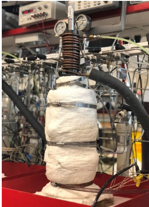
Figure 2.10: Oedometer fiberglass insulation
