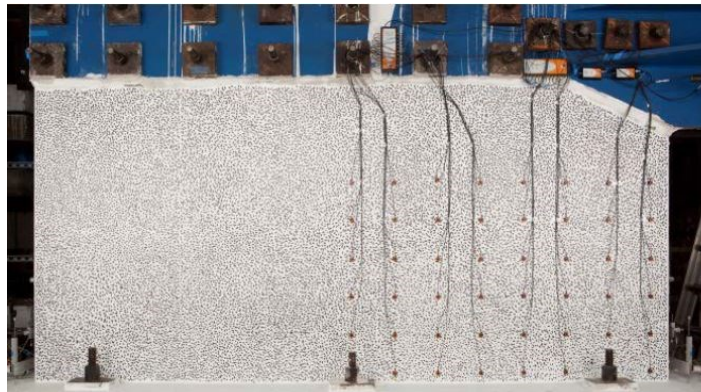
Figure 2.47. Hybrid testing of a shear wall specimen (Whyte and Stojadinovic 2012)
