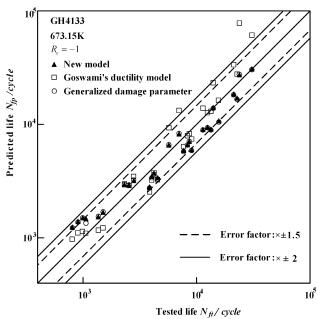
**Figure 2.** Comparison between lives predicted by new model, Goswami's ductility model, generalized damage parameter and lives tested for GH4133 at 673.15 K.
