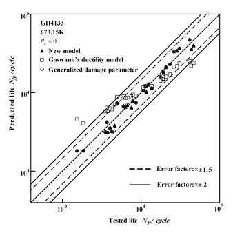
**Figure 3.** Comparison between lives predicted by new model, Goswami's ductility model, generalized damage parameter and lives tested for GH4133 under different mean strain levels at 673.15 K.
